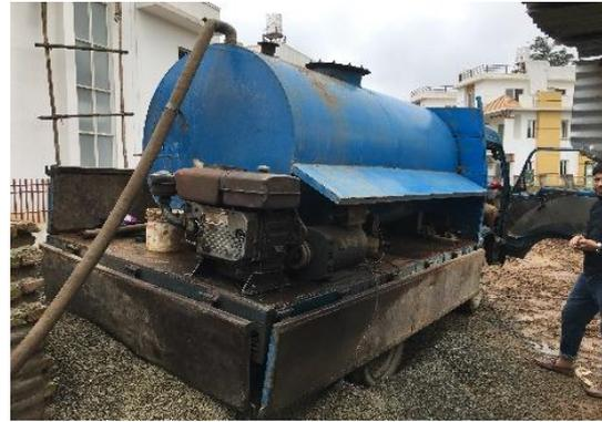
**Figure 3: Desludging vehicle; a tank equipped with movable centrifugal pump on a truck.**
