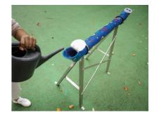
→ After brushing both ends of the WASHaLOT 3.0. flush the dirty water and rinse the pipe with clean water. WATER
