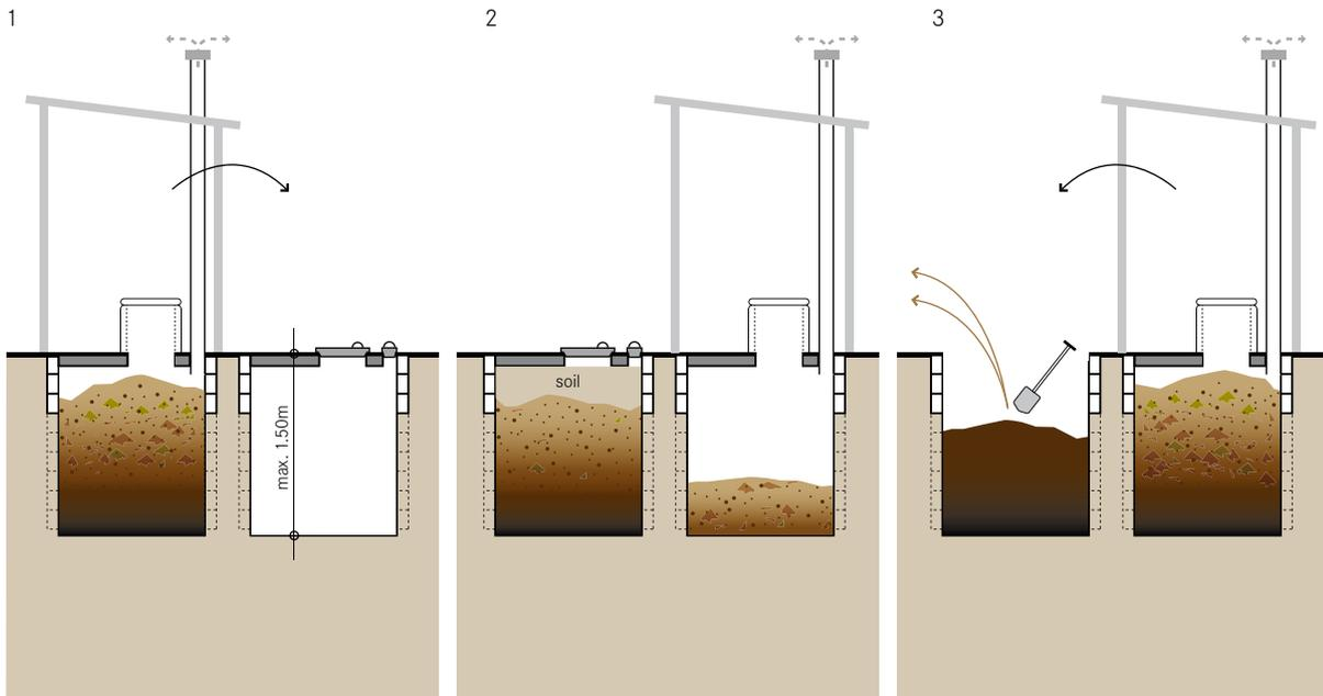
The Fossa Alterna is a short cycle alternating, waterless (dry) double pit technology. Compared to the Double VIP (S.4) which is just designed to collect, store and partially treat excreta, the Fossa Alterna is designed to make an earth-like product that can be used as a nutrient-rich soil conditioner. The Fossa Alterna is dug to a maximum depth of 1.5 m and requires a constant input of cover material (soil, ash, and/or leaves).
