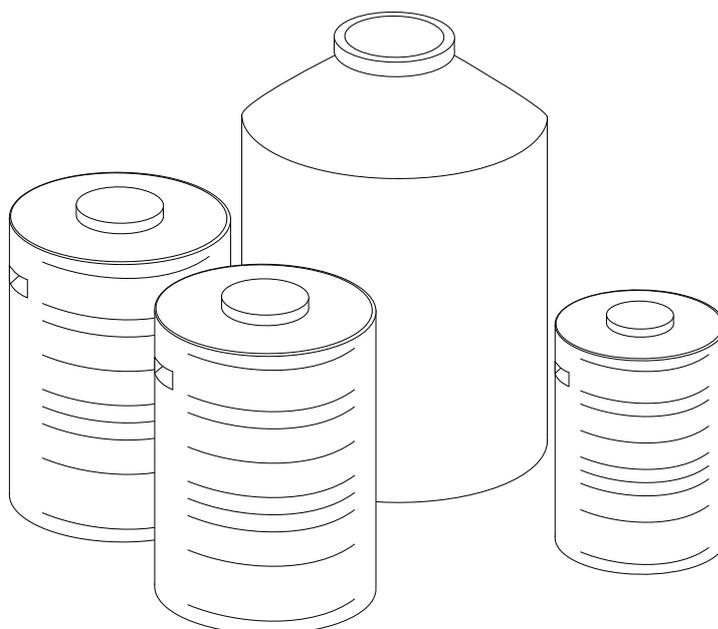
**When urine cannot be used immediately or transported using a Conveyance technology (i.e., Jerry-cans, see C.1), it can be stored onsite in containers or tanks. The storage tank must then be moved or emptied into another container for transport.**
