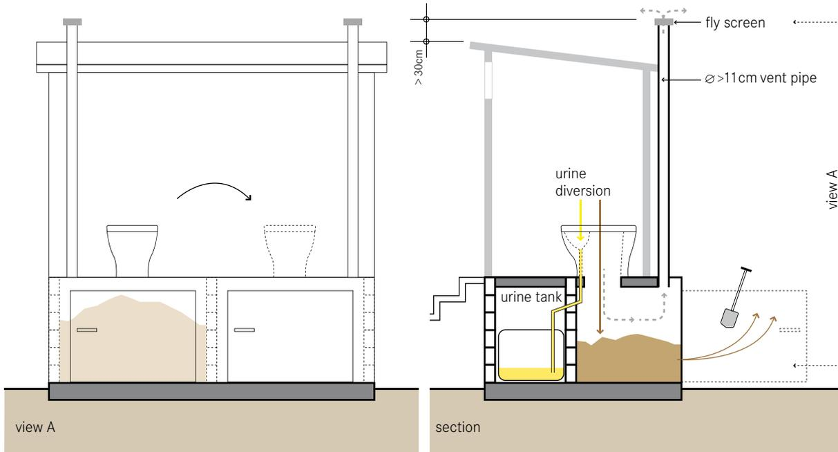
**Dehydration vaults are used to collect, store and dry (dehydrate) faeces. Faeces will only dehydrate when the vaults are well ventilated, watertight to prevent external moisture from entering, and when urine and anal cleansing water are diverted away from the vaults.**
