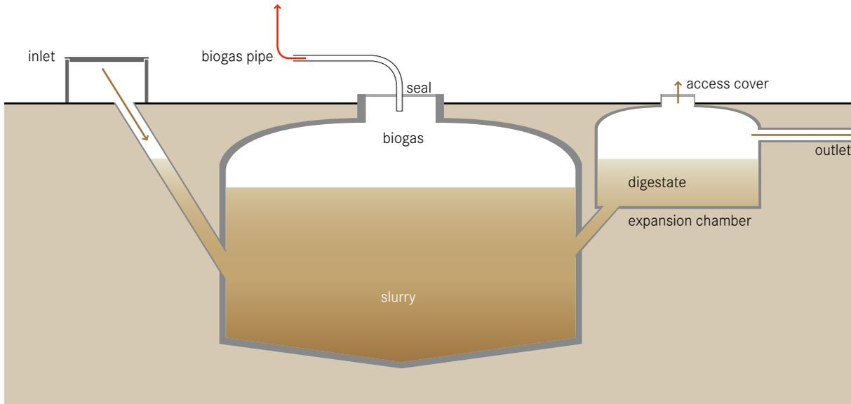
A biogas reactor or anaerobic digester is an anaerobic treatment technology that produces (a) a digested slurry (digestate) that can be used as a fertilizer and (b) biogas that can be used for energy. Biogas is a mix of methane, carbon dioxide and other trace gases which can be converted to heat, electricity or light.
