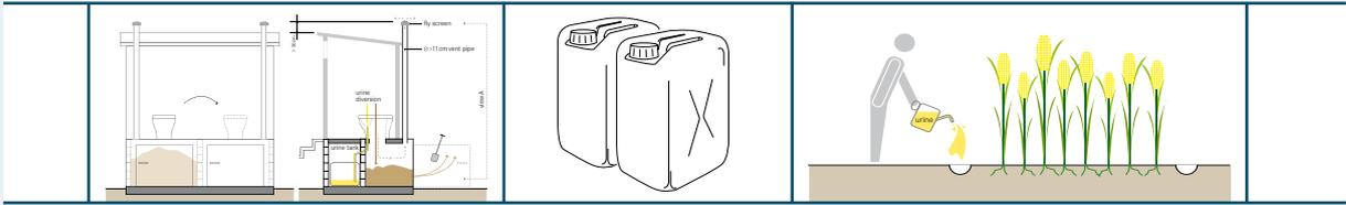
This system is designed to separate Urine and Faeces to allow the Faeces to dehydrate and/or recover the Urine for beneficial use. Inputs to the system can include Faeces, Urine, Anal Cleansing Water and Dry Cleansing Materials.
