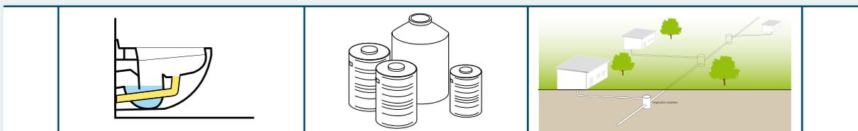
This is a water-based system that requires a Urine-Diverting Flush Toilet (UDFT, U.6) and a sewer. The UDFT is a special User Interface that allows for the separate collection of Urine without water, although it uses water to flush Faeces. Inputs to the system can include Faeces, Urine, Flushwater, Anal Cleansing Water, Dry Cleansing Materials, Greywater and possibly Stormwater.
