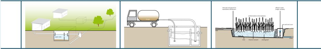
This system is characterized by the use of a household-level technology to remove and digest settleable solids from the Blackwater, and a Simplified (C.4) or Solids-Free (C.5) Sewer system to transport the Effluent to a (Semi-) Centralized Treatment facility. Inputs to the system can include Faeces, Urine, Flushwater, Anal Cleansing Water, Dry Cleansing Materials and Greywater.
