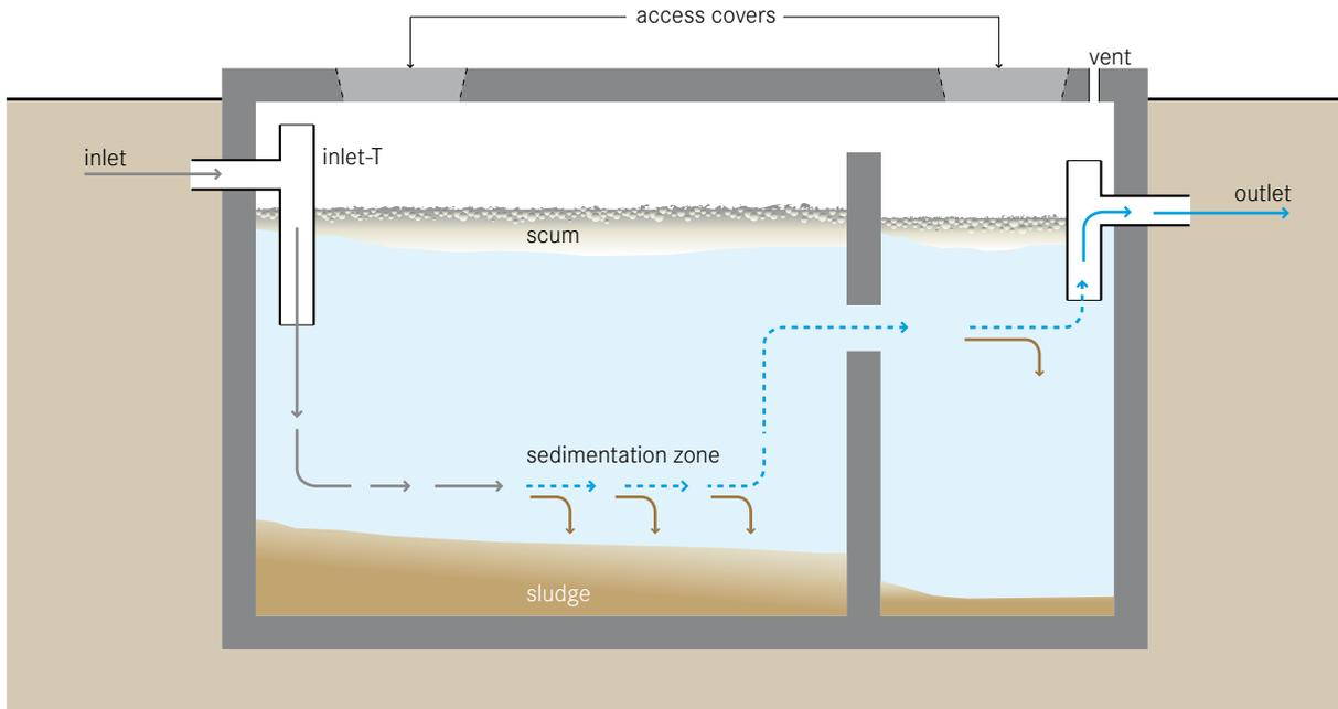
A septic tank is a watertight chamber made of concrete, fibreglass, PVC or plastic, through which blackwater and greywater flows for primary treatment. Settling and anaerobic processes reduce solids and organics, but the treatment is only moderate.
