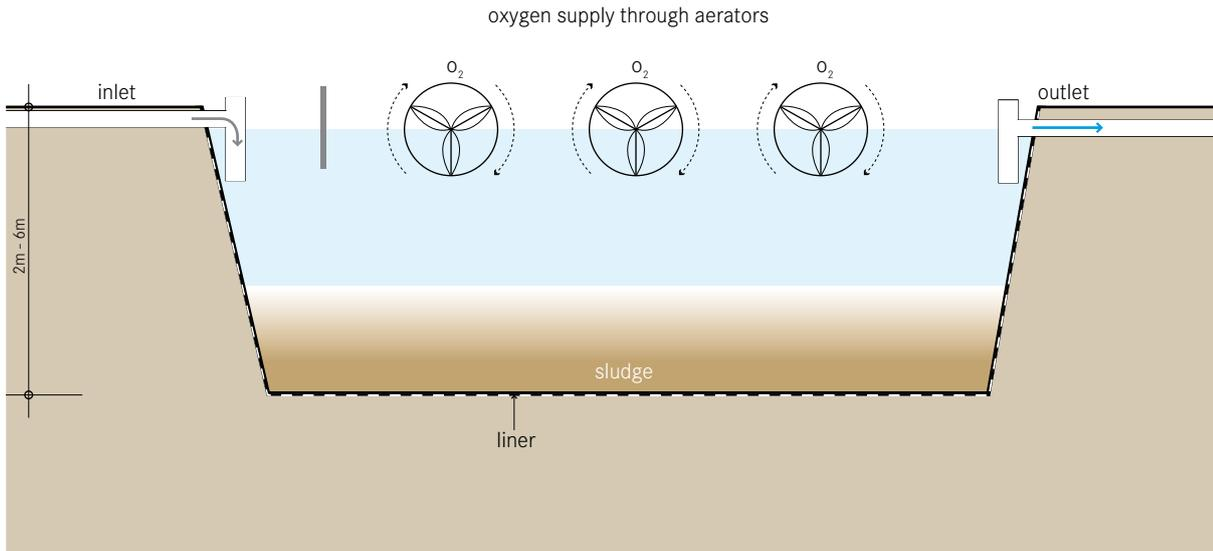
**An aerated pond is a large, mixed, aerobic reactor. Mechanical aerators provide oxygen and keep the aerobic organisms suspended and mixed with water to achieve a high rate of organic degradation.**
