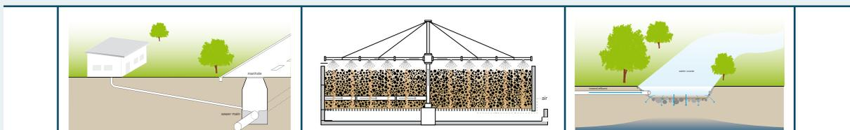
This is a water-based sewer system in which Blackwater is transported to a Centralized or Semi-Centralized Treatment facility. The important characteristic of this system is that there is no Collection and Storage/Treatment. Inputs to the system include Faeces, Urine, Flushwater, Anal Cleansing Water, Dry Cleansing Materials, Greywater and possibly Stormwater.
