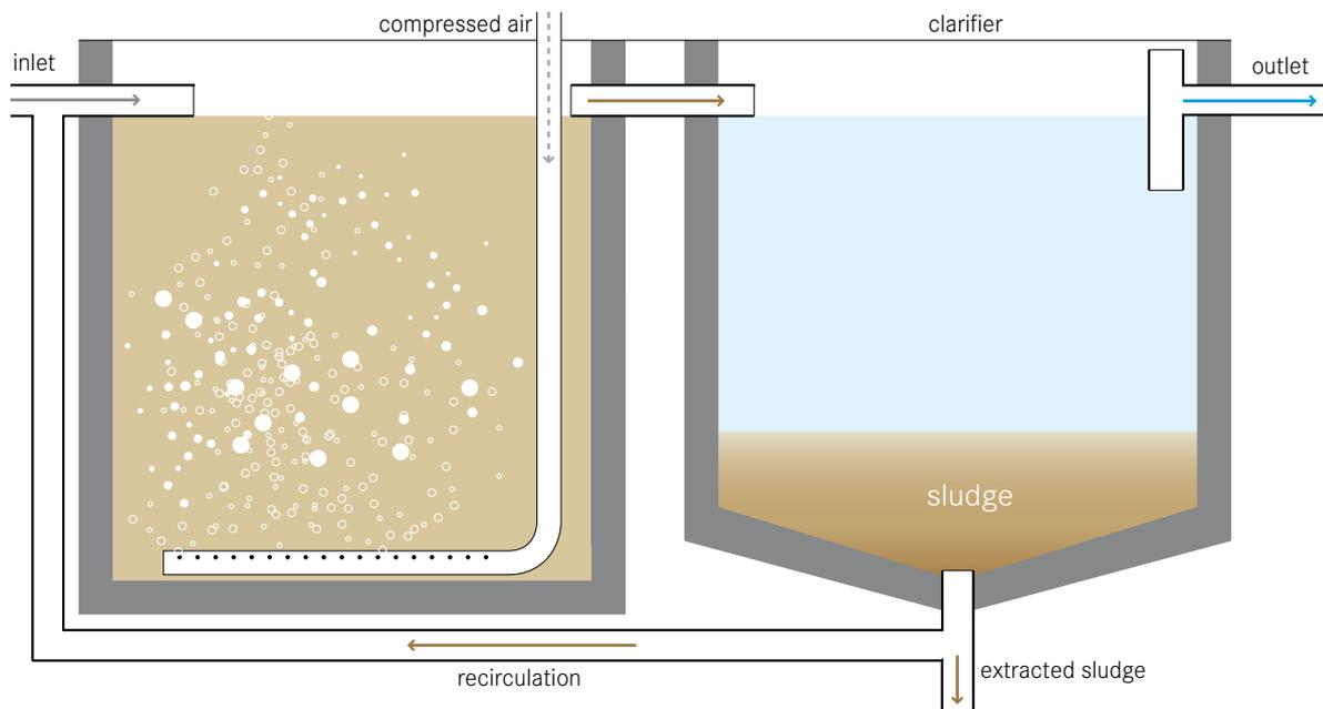
**An activated sludge process refers to a multi-chamber reactor unit that makes use of highly concentrated microorganisms to degrade organics and remove nutrients from wastewater to produce a high-quality effluent. To maintain aerobic conditions and to keep the activated sludge suspended, a continuous and well-timed supply of oxygen is required.**
