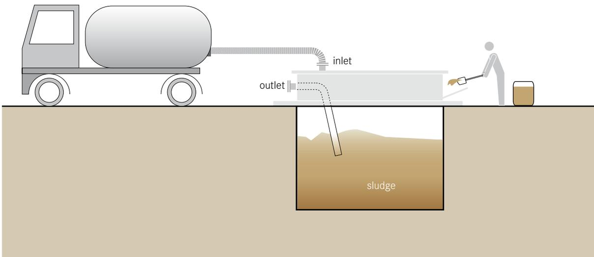
**Transfer stations or underground holding tanks act as intermediate dumping points for faecal sludge when it cannot be easily transported to a (Semi-) Centralized Treatment facility. A vacuum truck is required to empty transfer stations when they are full.**
