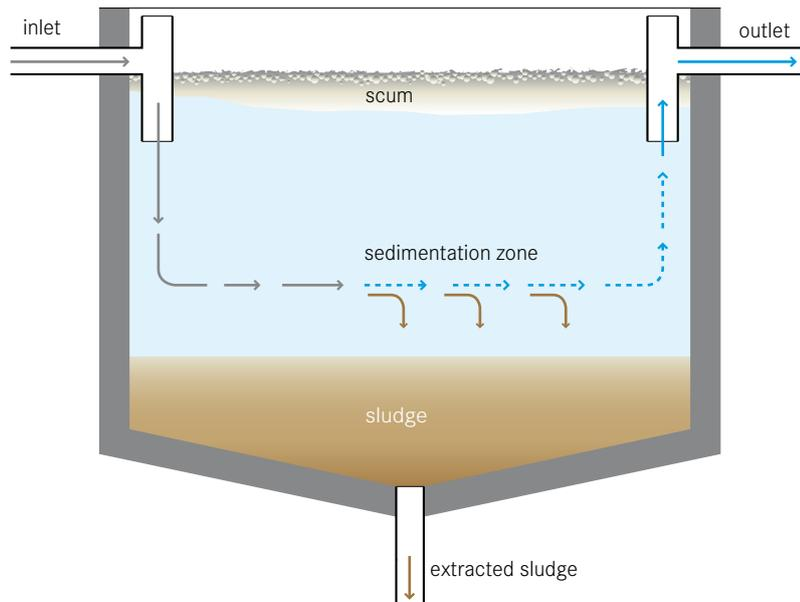
**A settler is a primary treatment technology for wastewater; it is designed to remove suspended solids by sedimentation. It may also be referred to as a sedimentation or settling basin/tank, or clarifier. The low flow velocity in a settler allows settleable particles to sink to the bottom, while constituents lighter than water float to the surface.**
