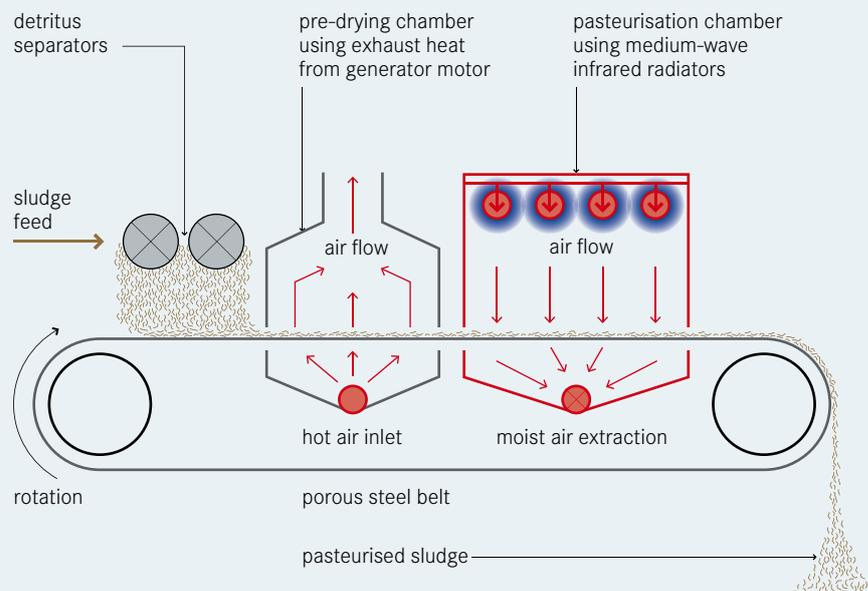
**Figure 6:** Schematic of the LaDePa sludge pelletizer
