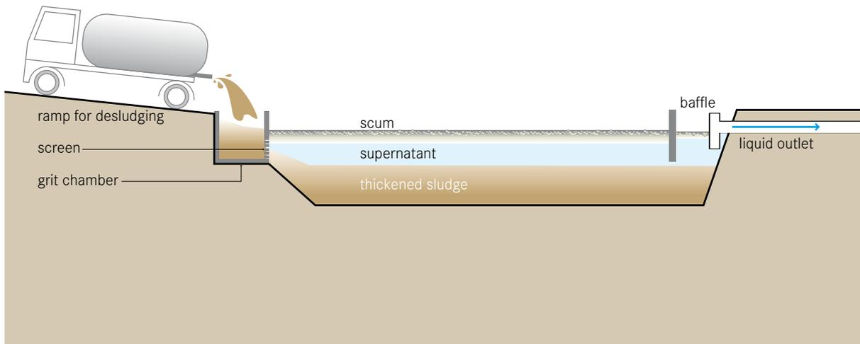
**Sedimentation or thickening ponds are settling ponds that allow sludge to thicken and dewater. The effluent is removed and treated, while the thickened sludge can be further treated in a subsequent technology.**
