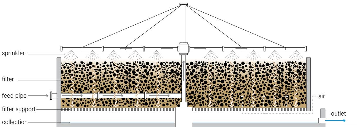
**A trickling filter is a fixed-bed, biological reactor that operates under (mostly) aerobic conditions. Pre-settled wastewater is continuously ‘trickled’ or sprayed over the filter. As the water migrates through the pores of the filter, organics are degraded by the biofilm covering the filter material.**
