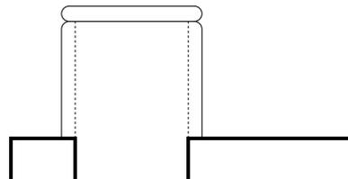
**A dry toilet is a toilet that operates without flushwater. The dry toilet may be a raised pedestal on which the user can sit, or a squat pan over which the user squats. In both cases, excreta (both urine and faeces) fall through a drop hole.**
