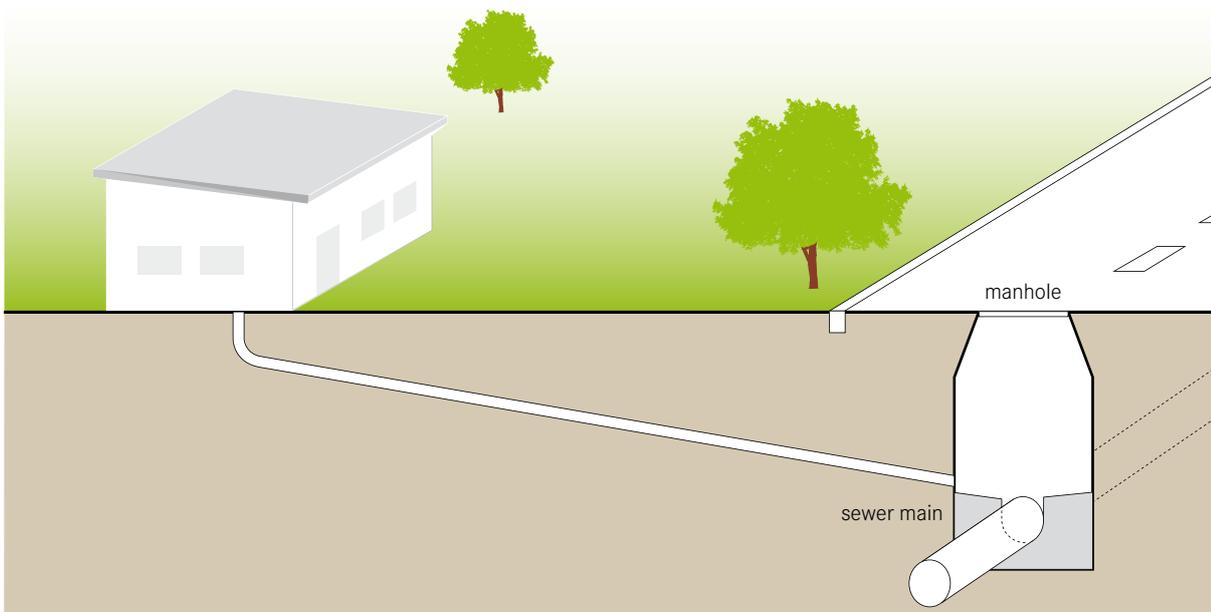
**Conventional gravity sewers are large networks of underground pipes that convey blackwater, greywater and, in many cases, stormwater from individual households to a (Semi-) Centralized Treatment facility, using gravity (and pumps when necessary).**
