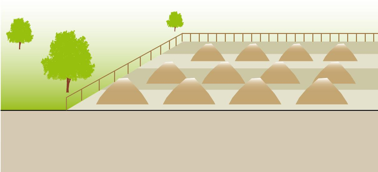
**Surface disposal refers to the stockpiling of sludge, faeces or other materials that cannot be used elsewhere. Once the material has been taken to a surface disposal site, it is not used later. Storage refers to temporary stockpiling. It can be done when there is no immediate need for the material and a future use is anticipated, or when further pathogen reduction and drying is desired before application.**
