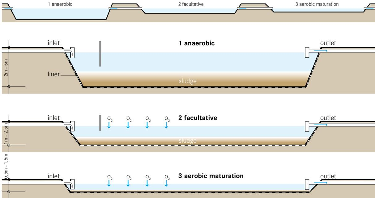
**Waste Stabilization Ponds (WSPs) are large, man-made water bodies. The ponds can be used individually, or linked in a series for improved treatment. There are three types of ponds, (1) anaerobic, (2) facultative and (3) aerobic (maturation), each with different treatment and design characteristics.**
