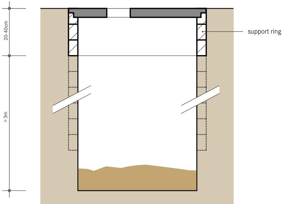
**The single pit is one of the most widely used sanitation technologies. Excreta, along with anal cleansing materials (water or solids) are deposited into a pit. Lining the pit prevents it from collapsing and provides support to the superstructure.**
