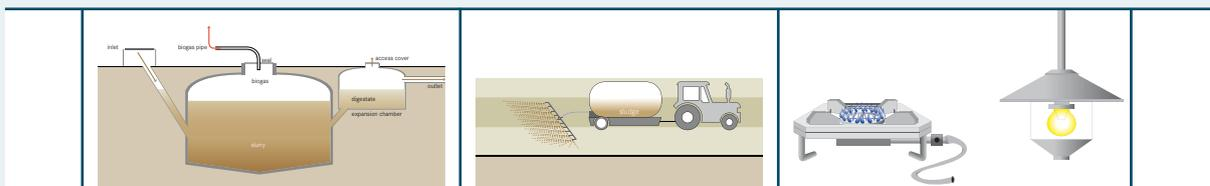
This system is based on the use of a Biogas Reactor (S.12) to collect, store and treat the Excreta. Additionally, the Biogas Reactor produces Biogas which can be burned for cooking, lighting or electricity generation. Inputs to the system can include Urine, Faeces, Flush-water, Anal Cleansing Water, Dry Cleansing Materials, Organics (e.g., market or kitchen waste) and, if available, animal waste.
