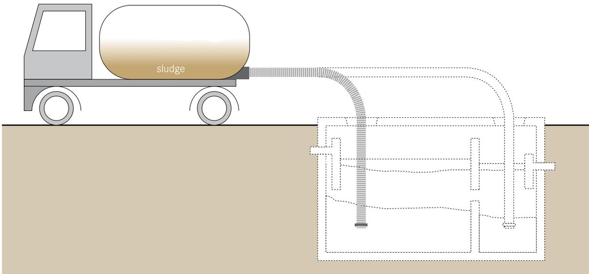
**Motorized emptying and transport** refers to a vehicle equipped with a motorized pump and a storage tank for emptying and transporting faecal sludge and urine. Humans are required to operate the pump and manoeuvre the hose, but sludge is not manually lifted or transported.
