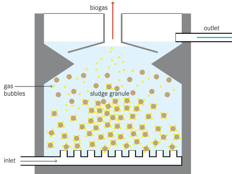
**The upflow anaerobic sludge blanket reactor (UASB) is a single tank process. Wastewater enters the reactor from the bottom, and flows upward. A suspended sludge blanket filters and treats the wastewater as the wastewater flows through it.**
