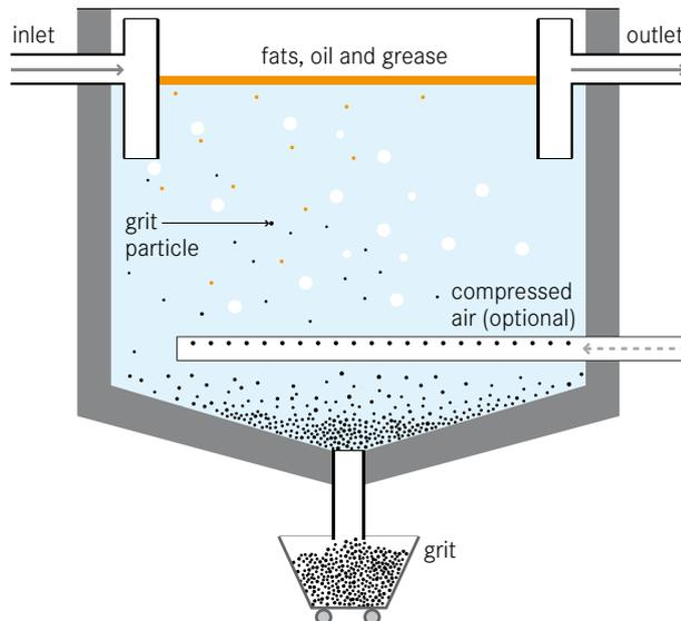
**Pre-treatment is the preliminary removal of wastewater or sludge constituents, such as oil, grease, and various solids (e.g., sand, fibres and trash). Built before a Conveyance or Treatment technology, pre-treatment units can retard the accumulation of solids and minimize subsequent blockages. They can also help reduce abrasion of mechanical parts and extend the life of the sanitation infrastructure.**
