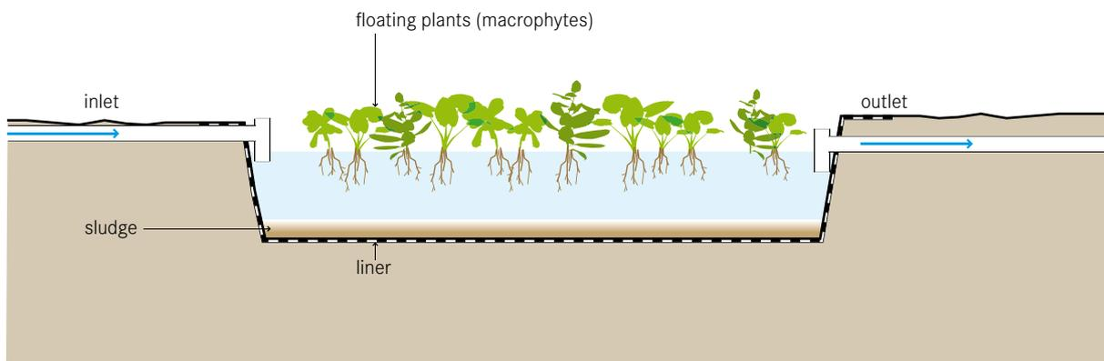
A floating plant pond is a modified maturation pond with floating (macrophyte) plants. Plants such as water hyacinths or duckweed float on the surface while the roots hang down into the water to uptake nutrients and filter the water that flows by.
