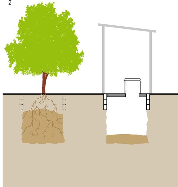
To decommission a pit, it can simply be filled with soil and covered. Although there is no benefit, the full pit poses no immediate health risk and the contents will degrade naturally over time. Alternatively, the Arborloo is a shallow pit that is filled with excreta and soil/ash and then covered with soil; a tree planted on top of the nutrient-rich pit will grow vigorously.
