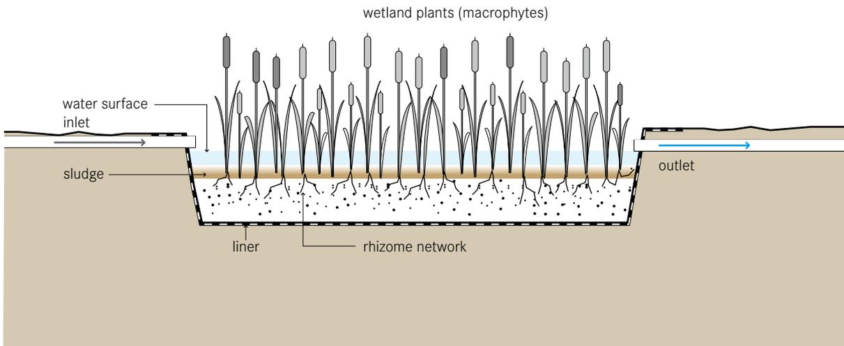
A free-water surface constructed wetland aims to replicate the naturally occurring processes of a natural wetland, marsh or swamp. As water slowly flows through the wetland, particles settle, pathogens are destroyed, and organisms and plants utilize the nutrients. This type of constructed wetland is commonly used as an advanced treatment after secondary or tertiary treatment processes.
