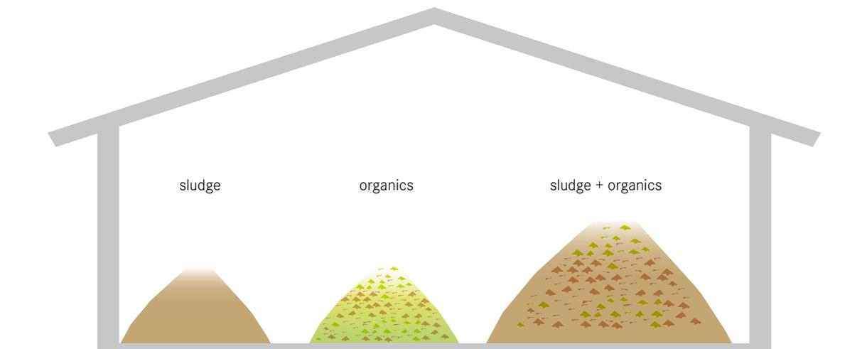
**Co-composting is the controlled aerobic degradation of organics, using more than one feedstock (faecal sludge and organic solid waste). Faecal sludge has a high moisture and nitrogen content, while biodegradable solid waste is high in organic carbon and has good bulking properties (i.e., it allows air to flow and circulate). By combining the two, the benefits of each can be used to optimize the process and the product.**
