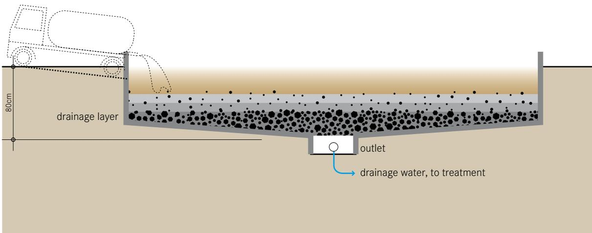
**An unplanted drying bed is a simple, permeable bed that, when loaded with sludge, collects percolated leachate and allows the sludge to dry by evaporation. Approximately 50% to 80% of the sludge volume drains off as liquid or evaporates. The sludge, however, is not effectively stabilized or sanitized.**
