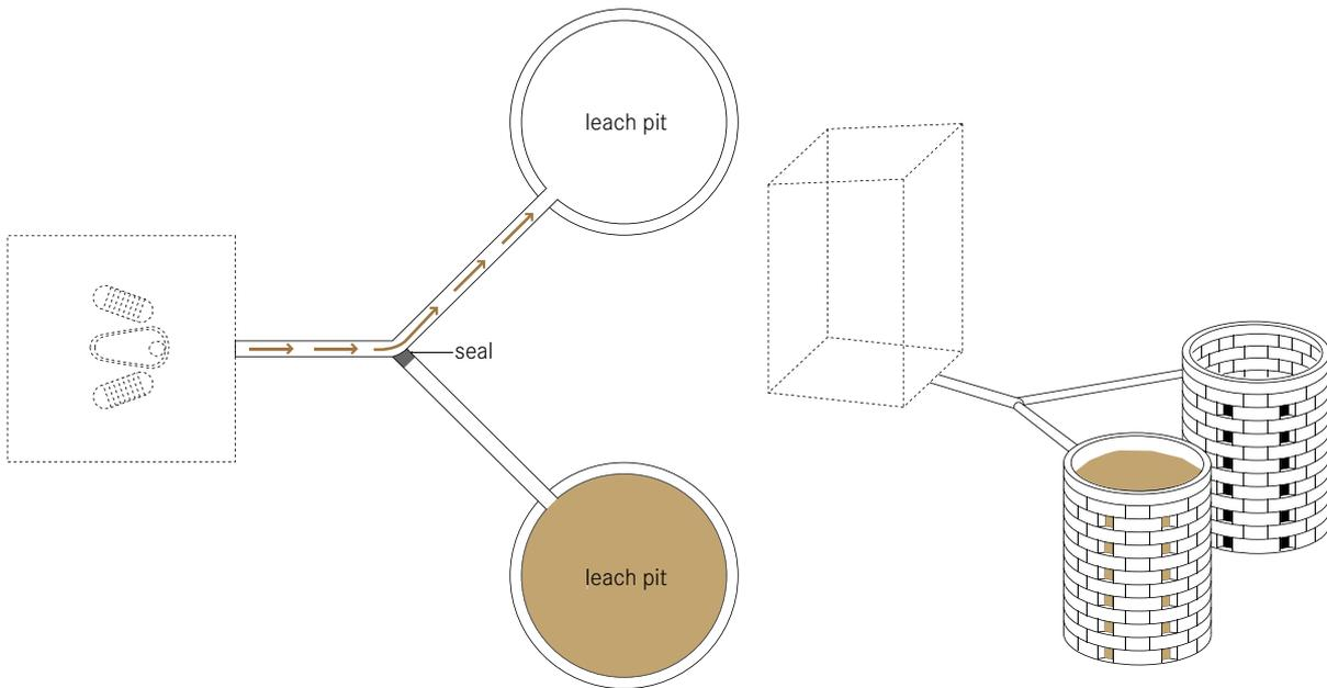
**This technology consists of two alternating pits connected to a Pour Flush Toilet (U.4). The blackwater (and in some cases greywater) is collected in the pits and allowed to slowly infiltrate into the surrounding soil. Over time, the solids are sufficiently dewatered and can be manually removed with a shovel.**
