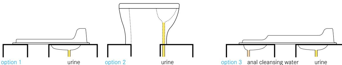
**A urine-diverting dry toilet (UDDT) is a toilet that operates without water and has a divider so that the user, with little effort, can divert the urine away from the faeces.**
