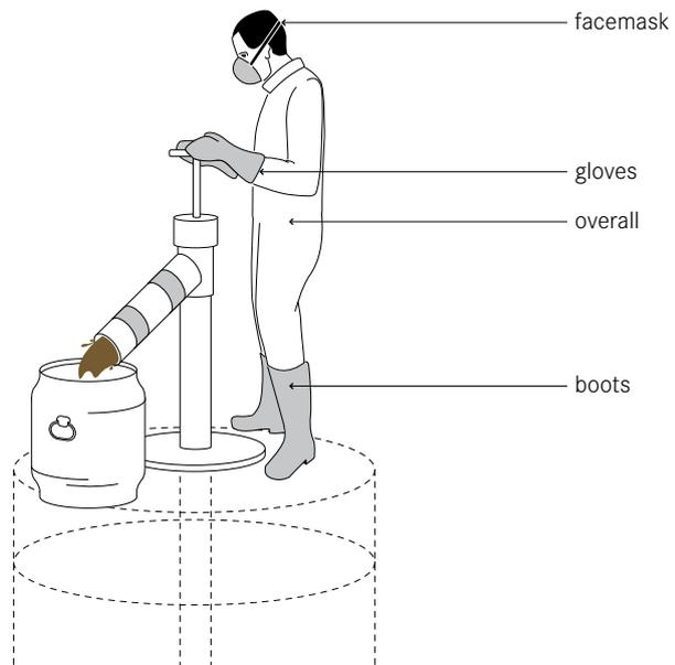
**Human-powered emptying and transport refers to the different ways by which people can manually empty and/or transport sludge and solid products generated in onsite sanitation facilities.**
