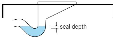
A pour flush toilet is like a regular Cistern Flush Toilet (U.5) except that the water is poured in by the user, instead of coming from the cistern above. When the water supply is not continuous, any Cistern Flush Toilet can become a pour flush toilet.
