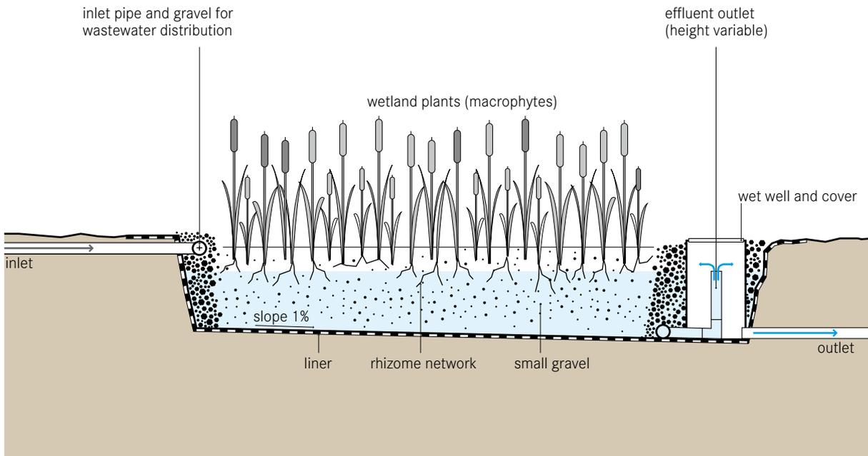
**A horizontal subsurface flow constructed wetland is a large gravel and sand-filled basin that is planted with wetland vegetation. As wastewater flows horizontally through the basin, the filter material filters out particles and microorganisms degrade the organics.**
