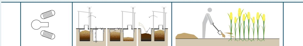
This system is designed to produce a solid, earth-like material by using alternating pits or a Composting Chamber (S.8). Inputs to the system can include Urine, Faeces, Organics, Anal Cleansing Water, and Dry Cleansing Materials. There is no use of Flushwater.
