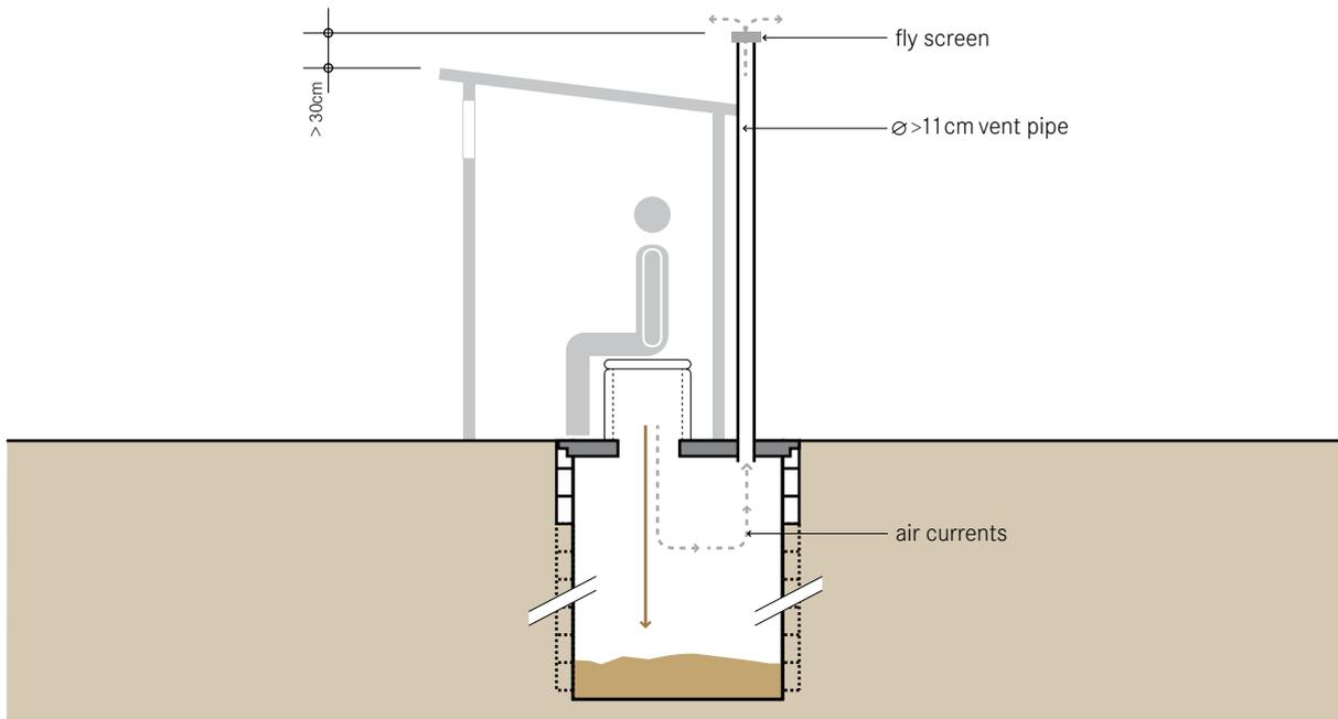
The single VIP is a ventilated improved pit. It is an improvement over the Single Pit (S.2) because continuous airflow through the ventilation pipe vents odours and acts as a trap for flies as they escape towards the light.
