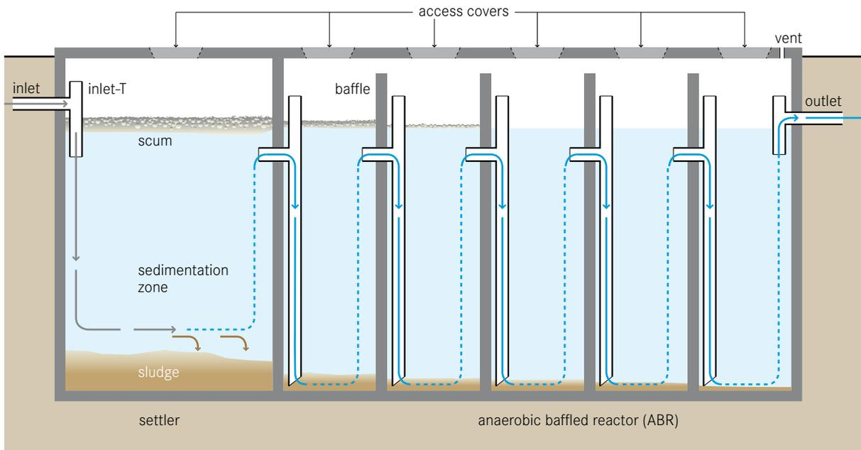
**An anaerobic baffled reactor (ABR) is an improved Septic Tank (S.9) with a series of baffles under which the wastewater is forced to flow. The increased contact time with the active biomass (sludge) results in improved treatment.**
