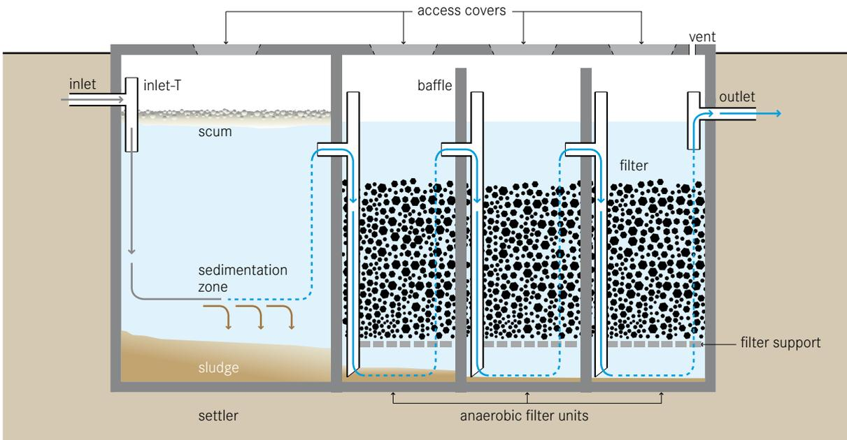
**An anaerobic filter is a fixed-bed biological reactor with one or more filtration chambers in series. As wastewater flows through the filter, particles are trapped and organic matter is degraded by the active biomass that is attached to the surface of the filter material.**
