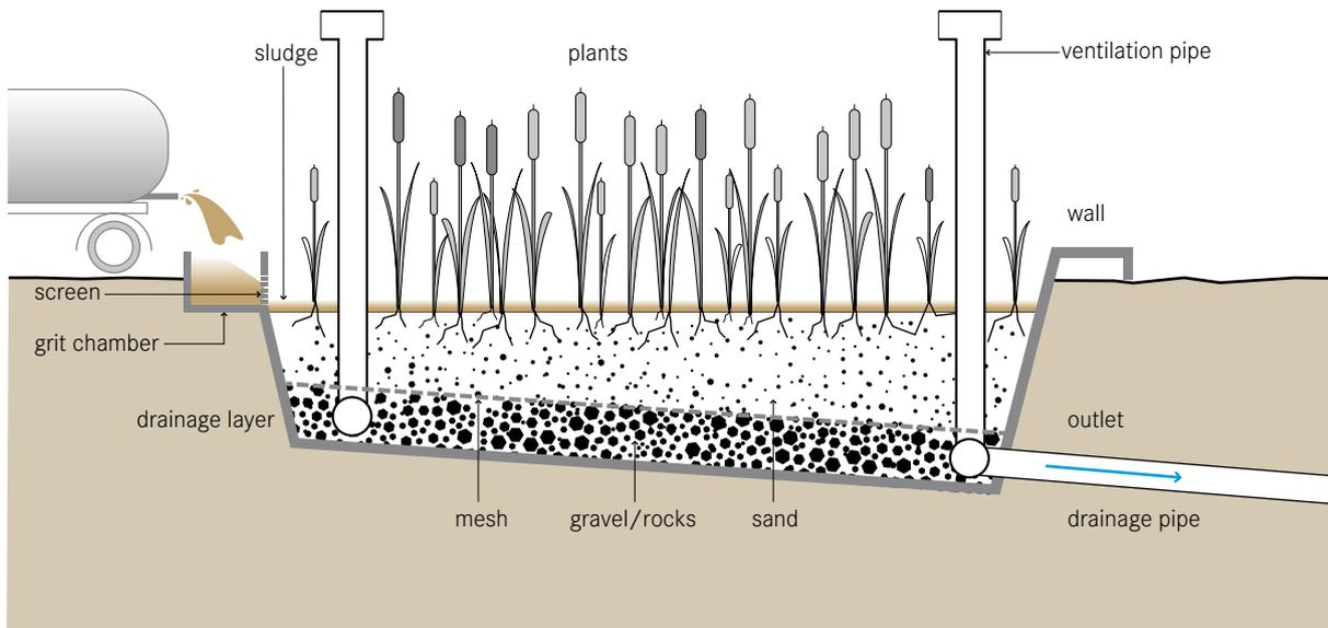
A planted drying bed is similar to an Unplanted Drying Bed (T.14), but has the added benefit of transpiration and enhanced sludge treatment due to the plants. The key improvement of the planted bed over the unplanted bed is that the filters do not need to be desludged after each feeding/drying cycle. Fresh sludge can be directly applied onto the previous layer; the plants and their root systems maintain the porosity of the filter.
