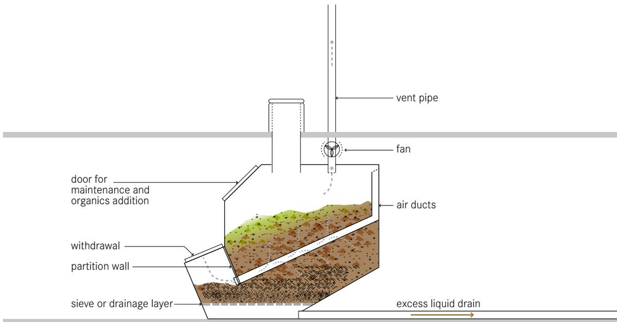
**Composting refers to the process by which biodegradable components are biologically decomposed by microorganisms (mainly bacteria and fungi) under aerobic conditions. A composting chamber is designed to convert excreta and organics into compost. Compost is a stable, inoffensive product that can be safely handled and used as a soil conditioner.**
