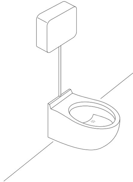
The urine-diverting flush toilet (UDFT) is similar in appearance to a Cistern Flush Toilet (U.5) except for the diversion in the bowl. The toilet bowl has two sections so that the urine can be separated from the faeces. Both sitting and squatting models exist.
