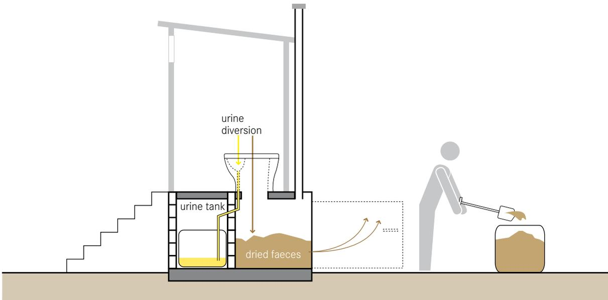
**When faeces are stored in the absence of moisture (i.e., urine), they dehydrate into a crumbly, white-beige, coarse, flaky material or powder. The moisture naturally present in the faeces evaporates and/or is absorbed by the drying material (e.g., ash, sawdust, lime) that is added to them. Dried faeces can be used as a soil conditioner.**
