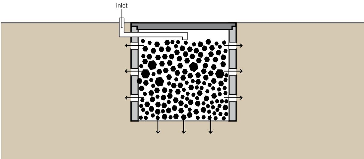
**A soak pit, also known as a soakaway or leach pit, is a covered, porous-walled chamber that allows water to slowly soak into the ground. Pre-settled effluent from a Collection and Storage/Treatment or (Semi-) Centralized Treatment technology is discharged to the underground chamber from which it infiltrates into the surrounding soil.**
