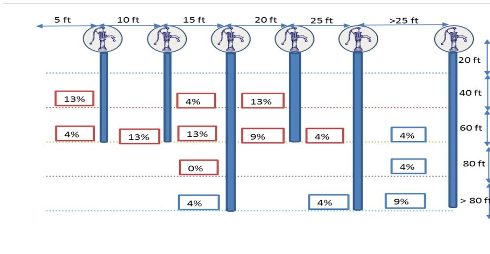
Figure 10: Depth of hand pumps and lateral spacing of it with containment type lined tank with impermeable wall and open bottom.
