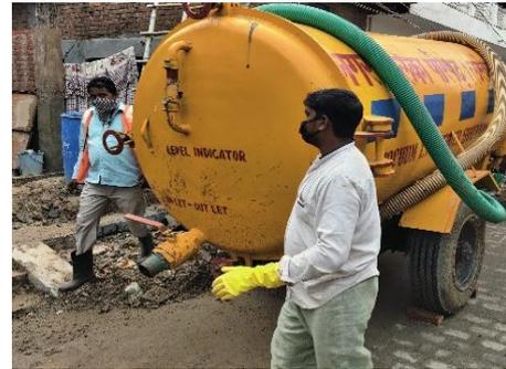
**Figure 5: Desludging by vacuum tanker in Santosh Nagar (Source: Abhishek/CSE, 2020)**
