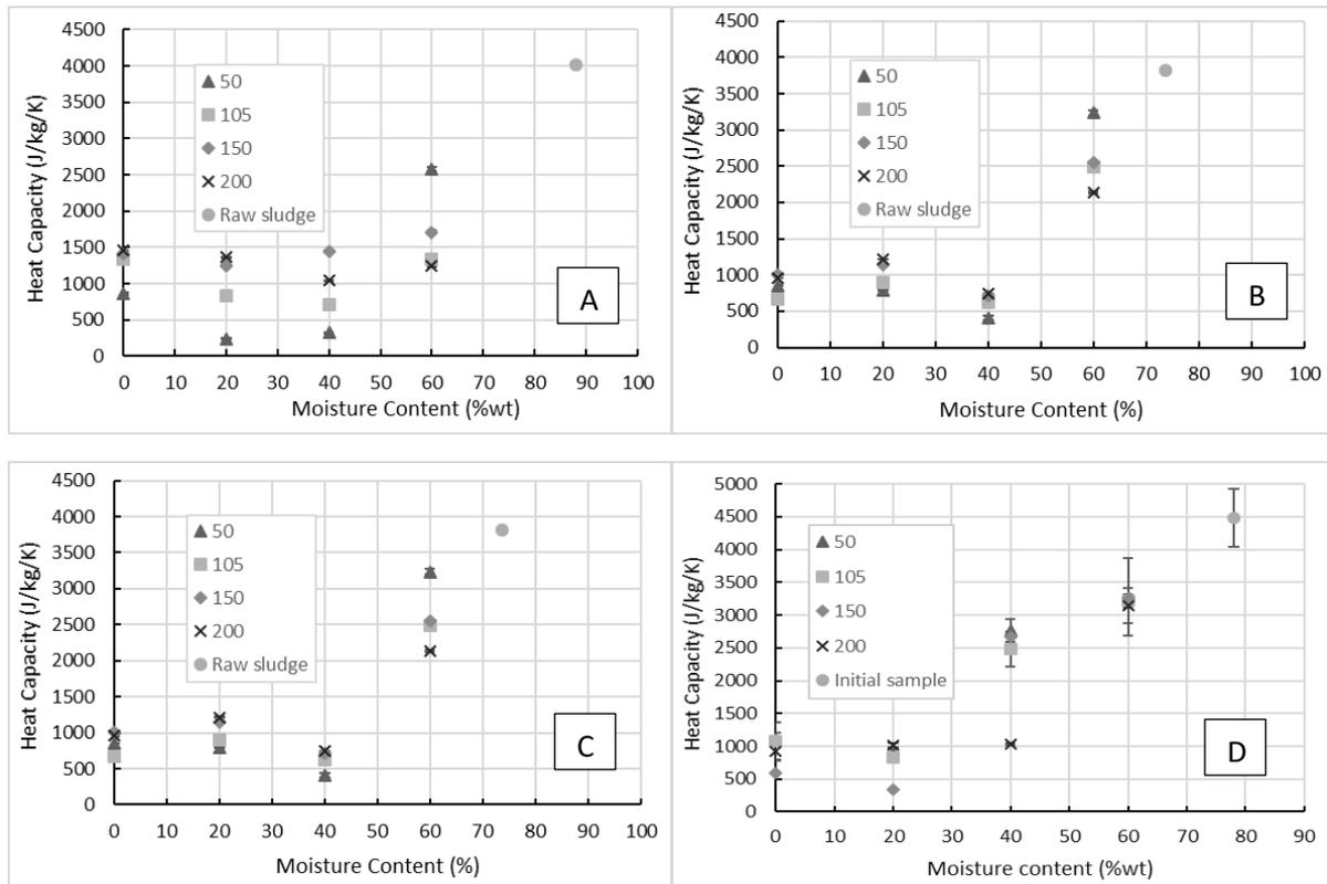
Figure 26. Heat capacity versus moisture content at different drying temperatures, for the faecal sludge from ABR (A), UDDT (B), wet VIP (C) and fresh faeces (D)
