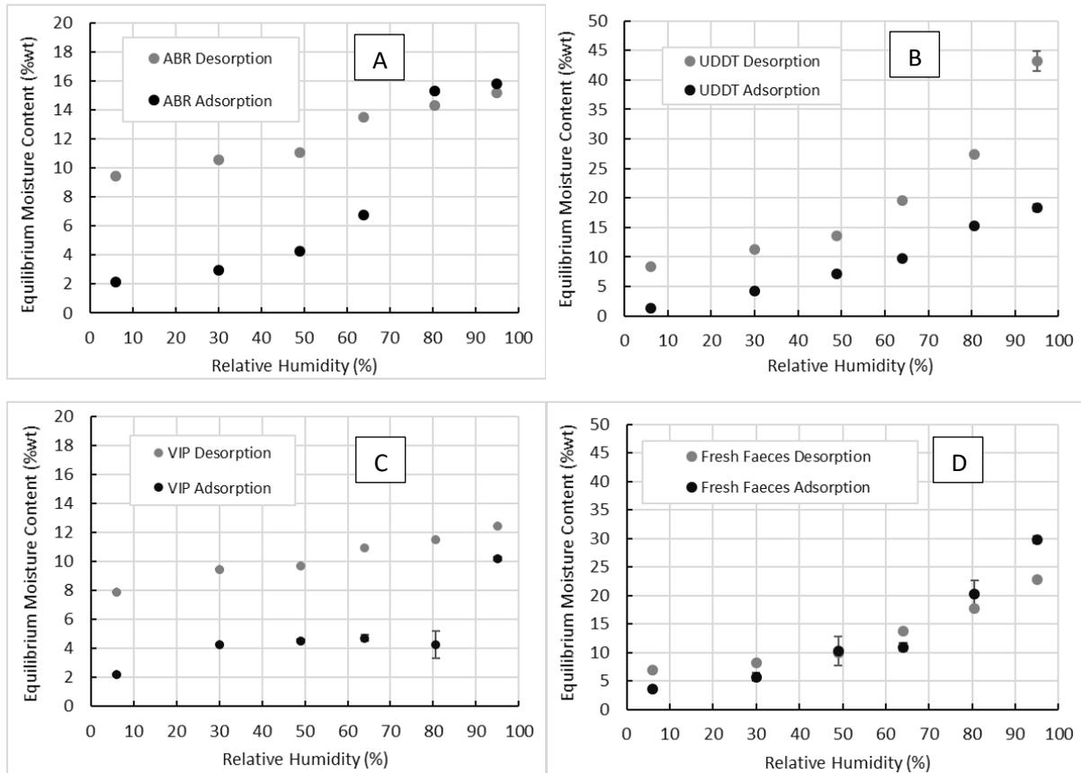
Figure 21. Desorption and adsorption isotherm curves for the sludge from ABR (A), UDDT (B), wet VIP (C) and fresh faeces (D) at ambient conditions
