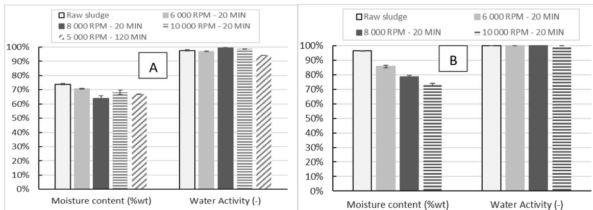
Figure 24. Moisture content and water activity before and after centrifugation for the sludge from UDDT (A) and wet VIP (B)
