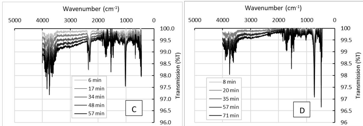
Figure 14. Transmittance spectrum measured by the FTIR analyzer at different instants during the drying STA tests at 55°C
