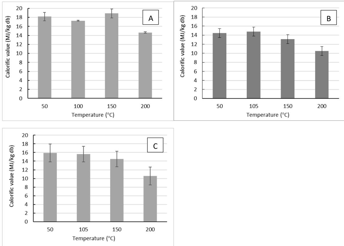
Figure 18. Gross calorific value of the sample after complete oven drying at different temperatures, for the faecal sludge from ABR (A), UDDT (B) and wet VIP (C)
