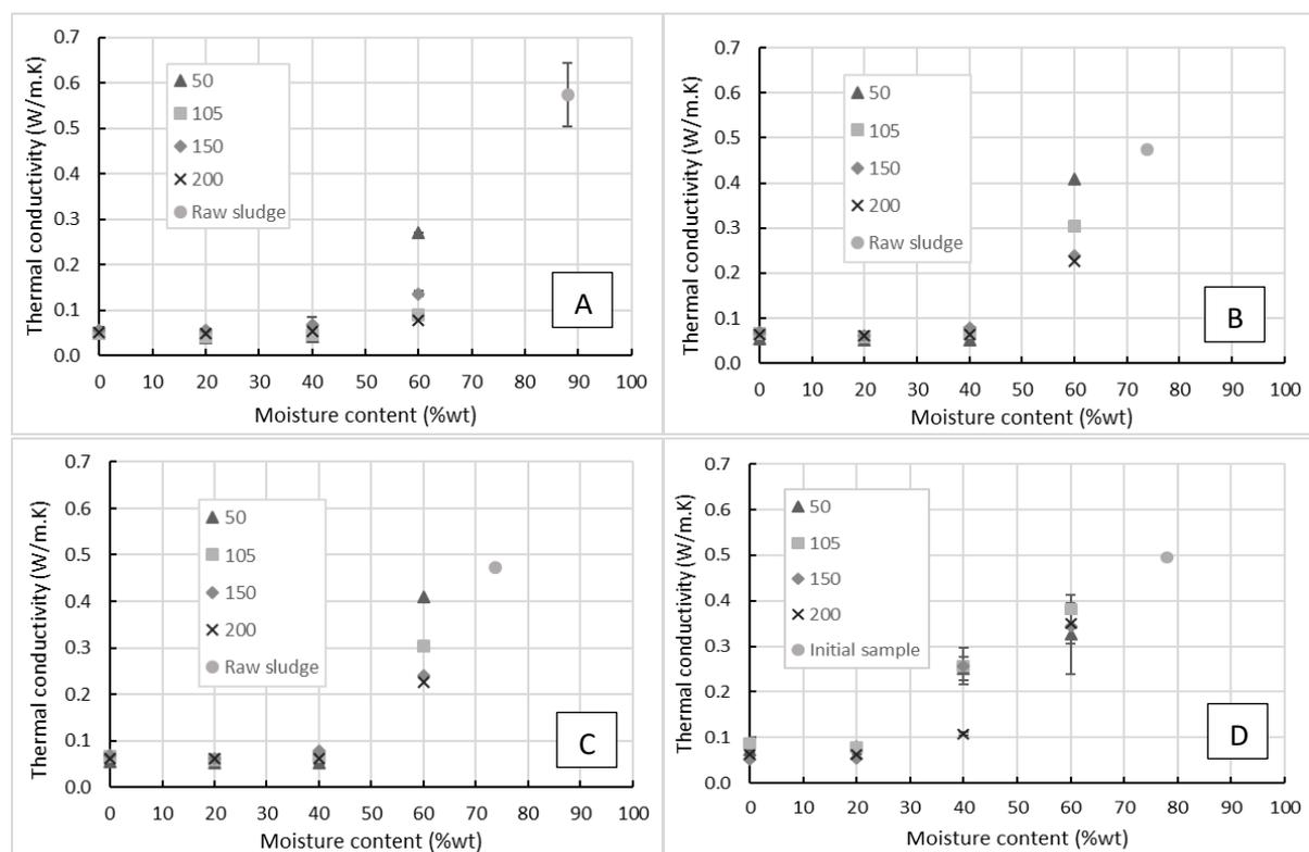
Figure 25. Thermal conductivity versus moisture content at different drying temperatures, for the faecal sludge from ABR (A), UDDT (B), wet VIP (C) and fresh faeces (D)
