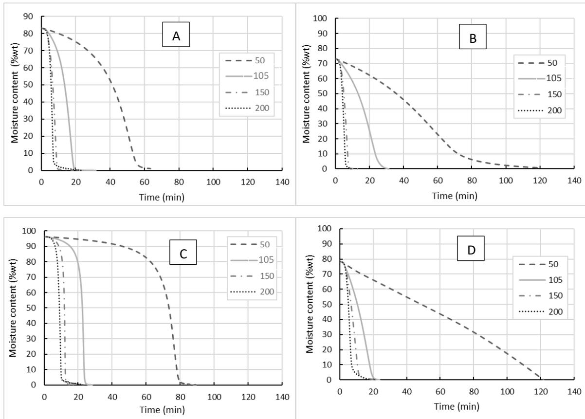
Figure 9. Drying curves obtained in the TGA at UKZN at different temperatures for the faecal sludge from ABR (A), UDDT (B), wet VIP (C) and fresh faeces (D).
