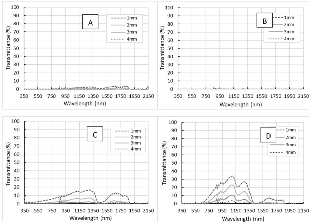
Figure 28. Transmittance for different thickness of ABR (A), UDDT (B), wet VIP (C) and fresh faeces (D) samples
