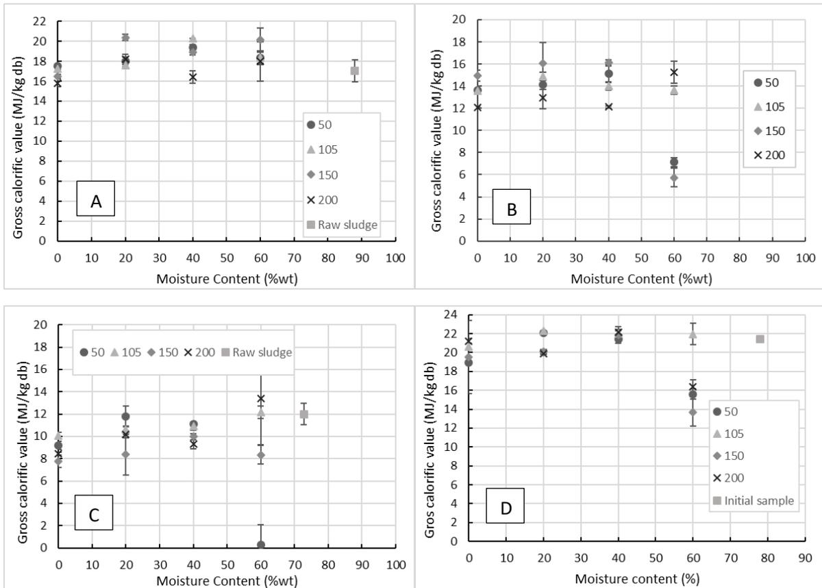
Figure 20. Gross calorific value versus moisture content at different drying temperatures, for the faecal sludge from ABR (A), UDDT (B), wet VIP (C) and fresh faeces (D)
