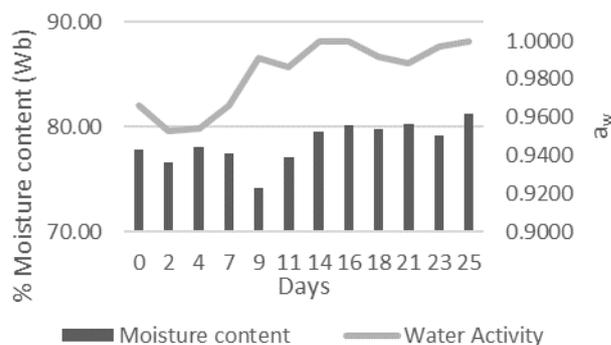
Figure 39. Moisture content and water activity measured in the faeces at different ageing times
