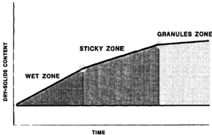
Figure 7. Presentation of the different phases during conductive drying (Lowe, 1995)
