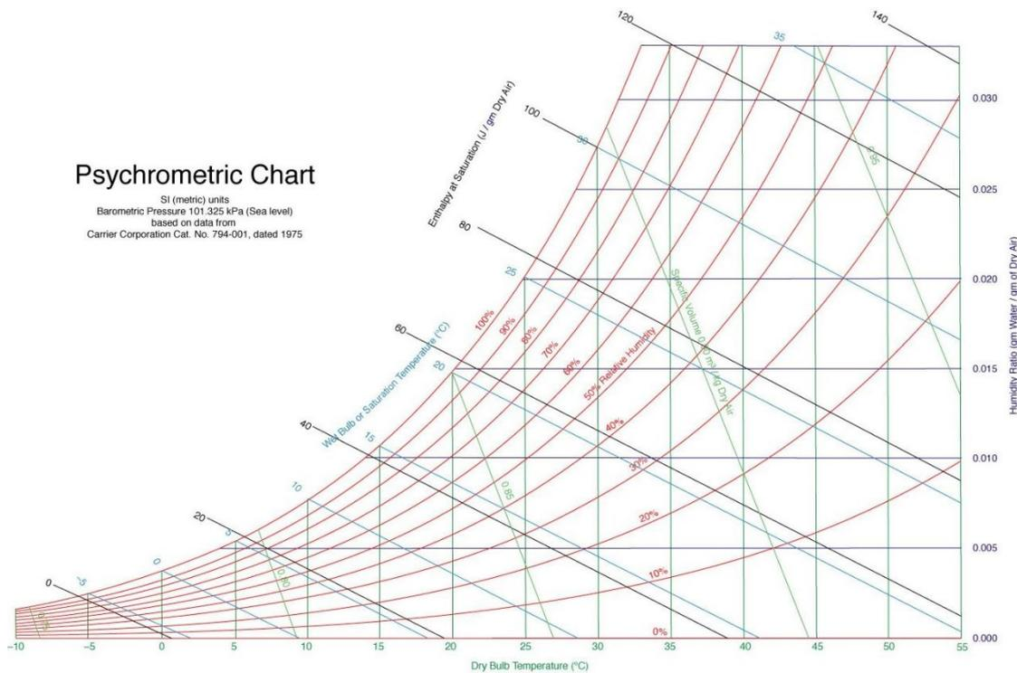
Figure 2. Psychrometric chart of vapour water-air mixture (source: Carrier Corporation)
