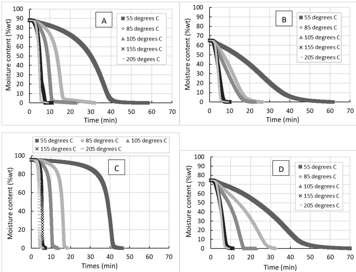
Figure 11. Drying curves obtained in the TGA at Cranfield University at different temperatures for the faecal sludge from ABR (A), UDDT (B), wet VIP (C) and fresh faeces (D)
