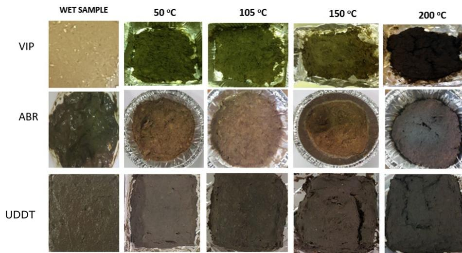
Figure 44. Photographs of ABR, UDDT and wet VIP samples dried in the oven at different temperatures
