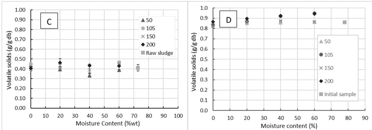
Figure 19. Volatile solids content versus moisture content at different drying temperatures, for the faecal sludge from ABR (A), UDDT (B), wet VIP (C) and fresh faeces (D)
