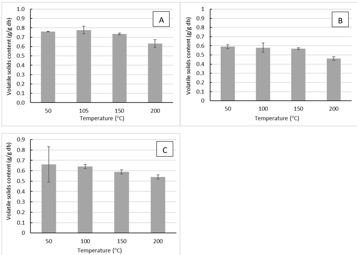
Figure 17. Volatile solids of the sample after complete oven drying at different temperatures, for the faecal sludge from ABR (A), UDDT (B) and wet VIP (C)
