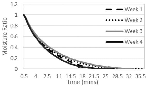
Figure 40. Moisture ratio versus time measured in the faeces at different ageing times (moisture ratio being as the moisture content normalized by its initial value)
