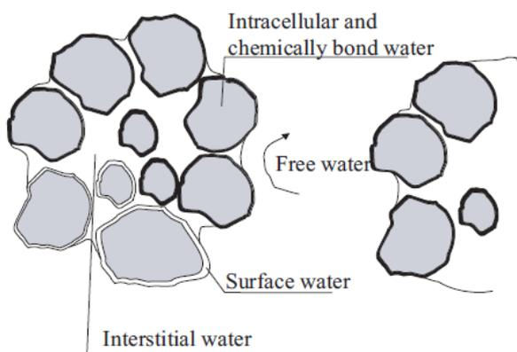
Figure 6. Water distribution in the sludge (Chen et al., 2002)
