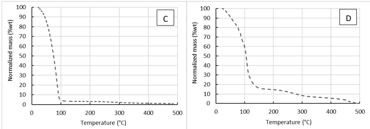
Figure 16. Normalized mass of the sample with respect to the initial value as a function of temperature for the faecal sludge from ABR (A), UDDT (B), dry VIP (C) and fresh faeces (D)
