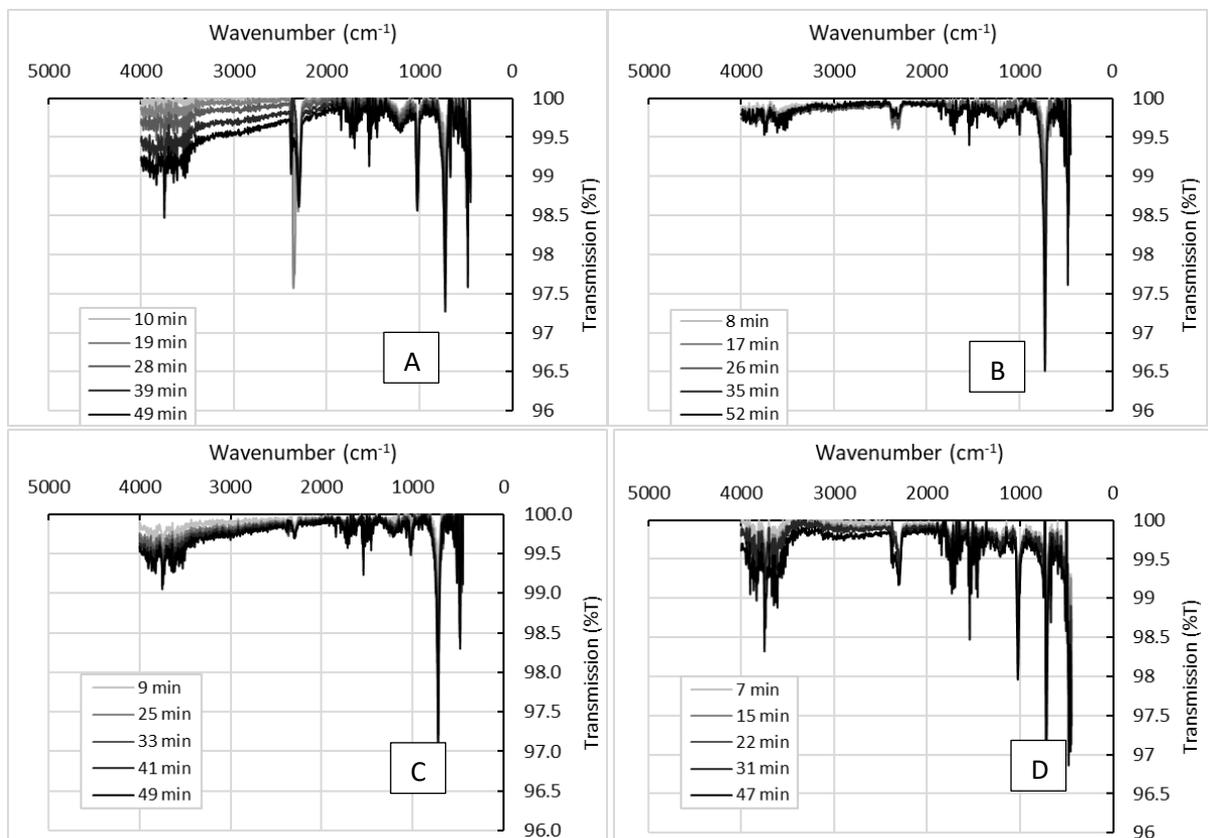
Figure 15. Transmittance spectrum measured by the FTIR analyzer at different instants during the drying STA tests at 155°C
