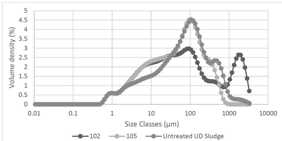
Figure 38. Particle size distribution of the UDDT faecal sludge before and after viscous heating treatment at different time-temperature exposures
