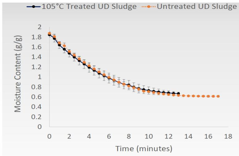
Figure 36. Moisture content versus time during the drying of the UDDT faecal sludge before and after viscous heating treatment at 105°C
