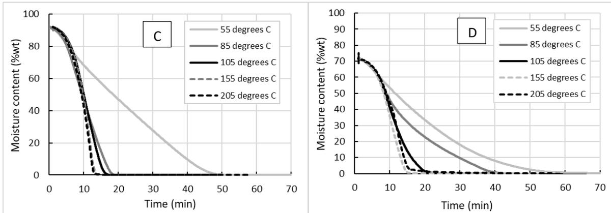
Figure 10. Drying curves obtained in the TGA at Swansea University at different temperatures for the faecal sludge from ABR (A), UDDT (B), wet VIP (C) and fresh faeces (D)
