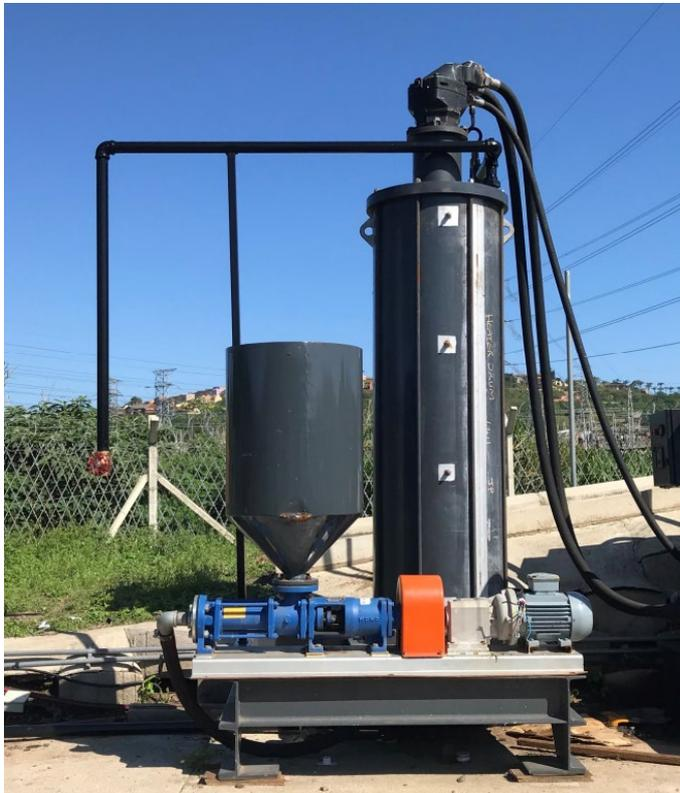
Figure 35. Photograph of the 1,000 L/h viscous heater
