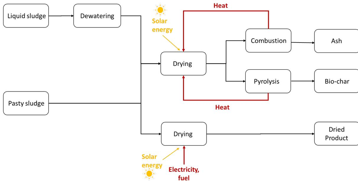
Figure 8. Faecal waste drying flow diagram
