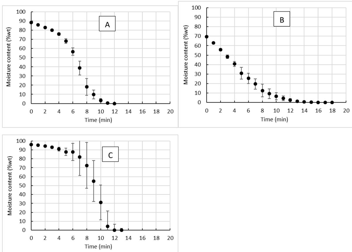
Figure 12. Drying curves obtained in the moisture analyzer balance at UKZN at 100°C for the faecal sludge from ABR (A), UDDT (B) and wet VIP (C)
