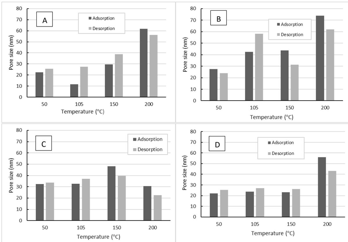
Figure 30. Mean pore size as a function of drying temperature for the samples from ABR (A), UDDT (B), wet VIP (C) and dry VIP (D), using two measurements methods (adsorption / desorption)
