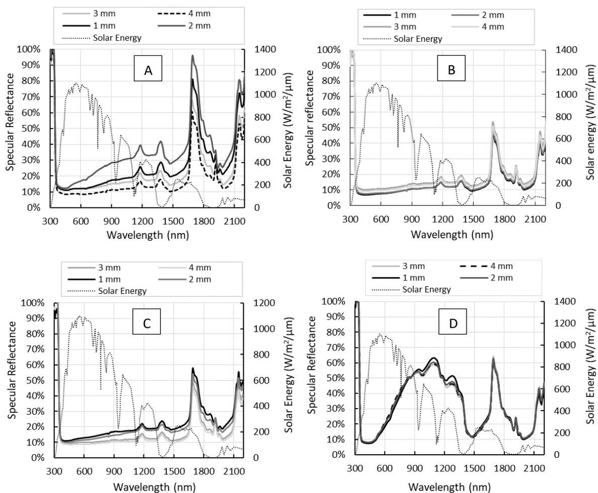
Figure 27. Reflectance for different thickness of ABR (A), UDDT (B), wet VIP (C) and fresh faeces (D) sample, compared to the solar irradiance spectrum
