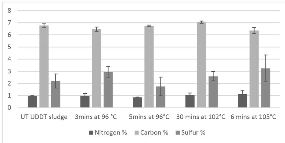
Figure 37. Carbon, nitrogen and sulphur content the UDDT faecal sludge before and after viscous heating treatment at different time-temperature exposures
