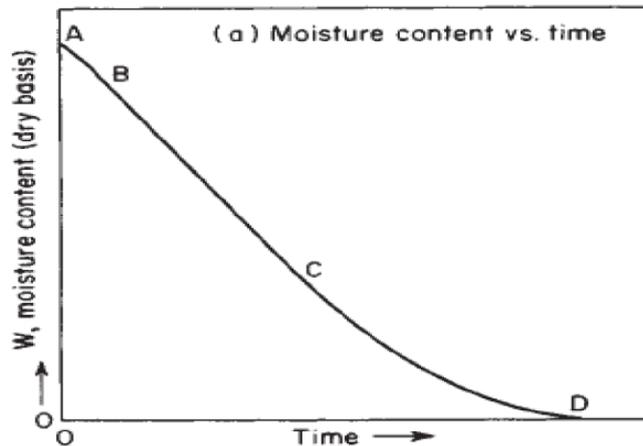
Figure 4. Typical drying curve (Moyers and Baldwin, 1997)
