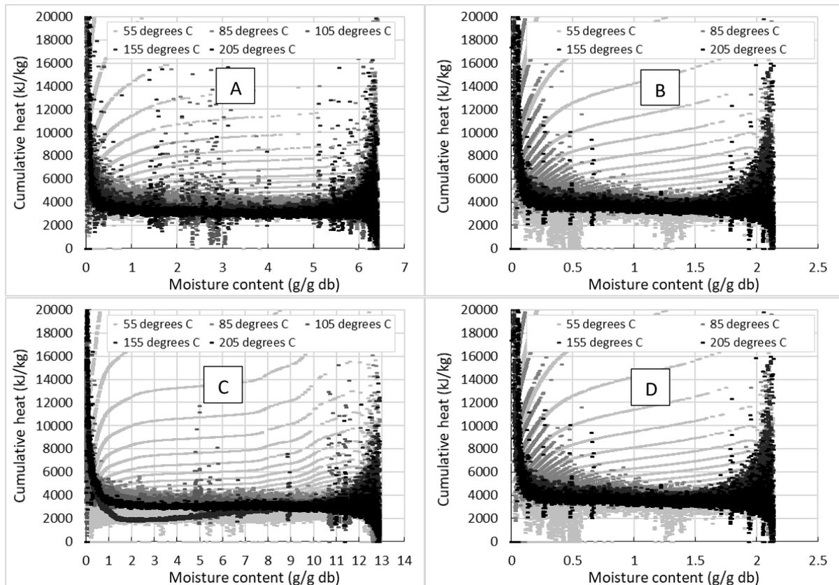
Figure 13. Heat of drying measured by the STA at Swansea University during the drying of faecal sludge from ABR (A), UDDT (B), wet VIP (C) and fresh faeces (D) at different temperatures
