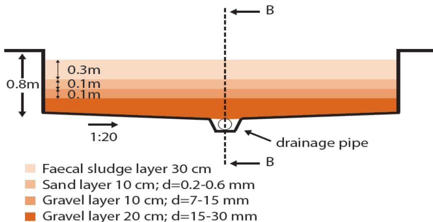
gravel that support the sludge and allow the liquid to infiltrate and collect in the pipe.
