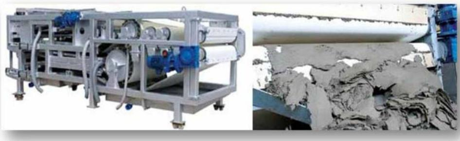
Both solid and liquid parts still contain pathogens and pollutants and further treatment is necessary. Mechanical parts need periodical inspection and replacement.
