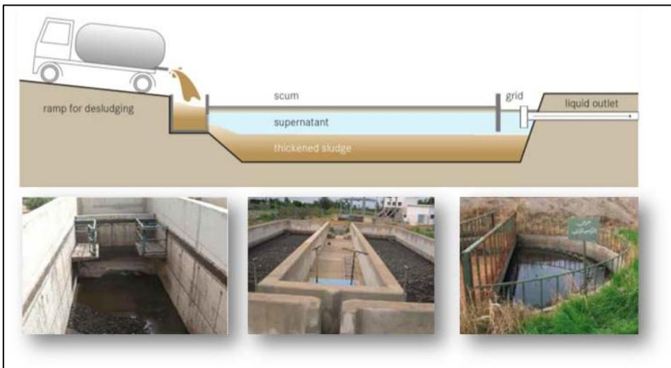
Here input is faecal sludge and output is dried Septage and effluent, which can be used in agriculture, arboriculture and pastures. This treatment option can be coupled with sludge drying bed or co-composting for treatment of thickened sludge. This technology is affected by seasonal changes and can be efficiently used in hot and temperate climate. The discharging area must be maintained
