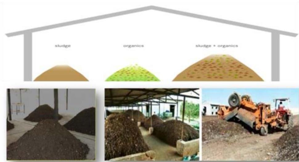
In this technique input is faecal sludge and biodegradable organic solid waste and output is compost which can be use in agriculture, arboriculture and pastures. It is affected by seasonal changes and depending on the climate (rainfall, temperature and wind) the Co-Composting facility can be built to accommodate the conditions. At places where there is heavy rainfall covered facilities are especially recommended.
