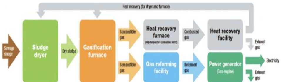
**Advantages:** Technology best suitable for dry feed stocks. The produced gas can be converted into any type of fuel by FT synthesis.
