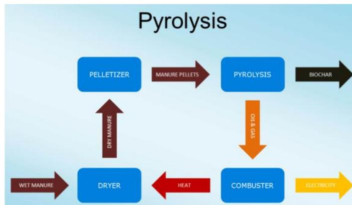
produce complex oil in the absence of air/oxygen. In this technology sludge is converted to Bio-oil, Pyrolytic Gas and Bio-char. Here also drying of sludge is required prior for treatment in incinerators. This technology requires trained operators and there is risk of malfunction if not properly maintained and operated.
