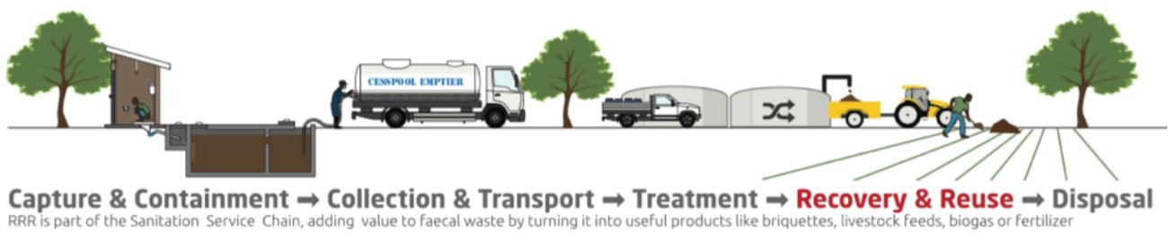
Figure 1: Considering the entire sanitation service and value chain from containment through collection & transport, treatment, recovery & reuse or disposal. [Source: GIZ-ENWASS]
