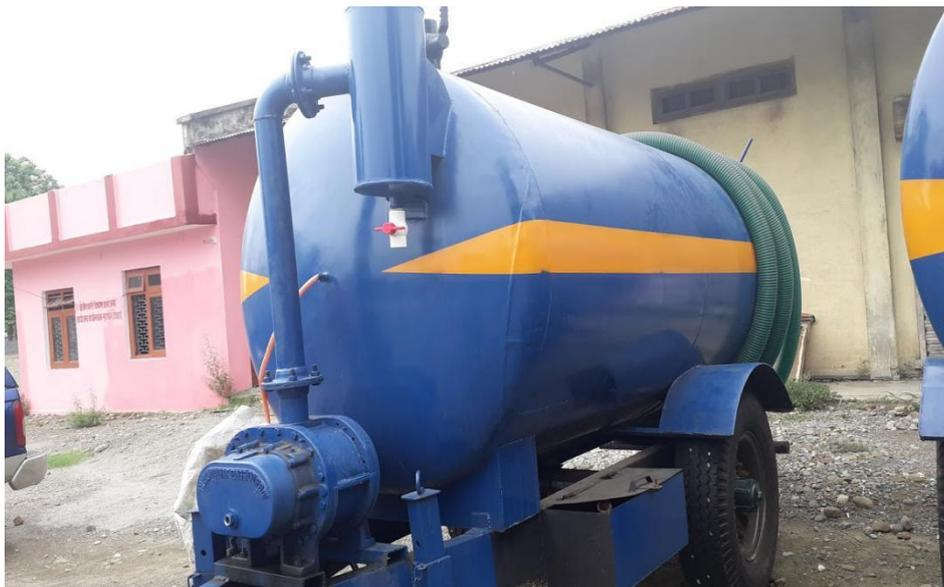
Figure 12: A newly purchased desludging vehicle by the Bheemdatt Municipality.
