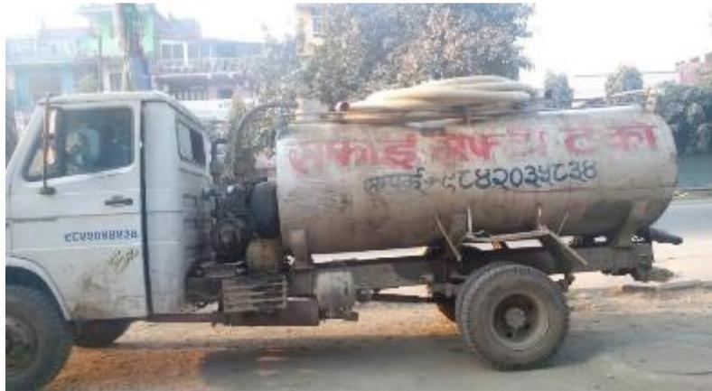
Figure 6: Locally assembled mechanized emptying vehicle
