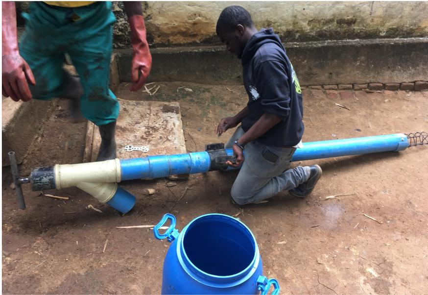
Figure 7. A Gulper used for manual emptying (Source: Tilley, 2018)
