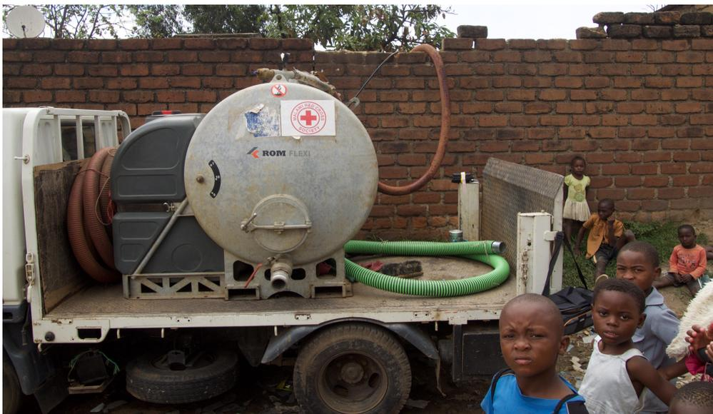
Figure 8. Mobile Desludging Unit (Source: Tilley, 2018)
