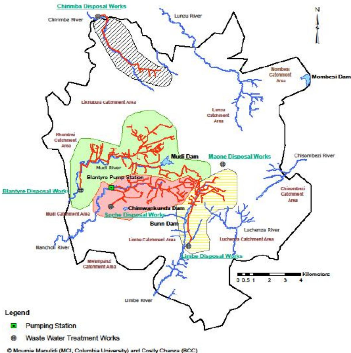
Figure 10. Sewer lines and treatment plants in Blantyre (Source: Maoulidi, 2012)
