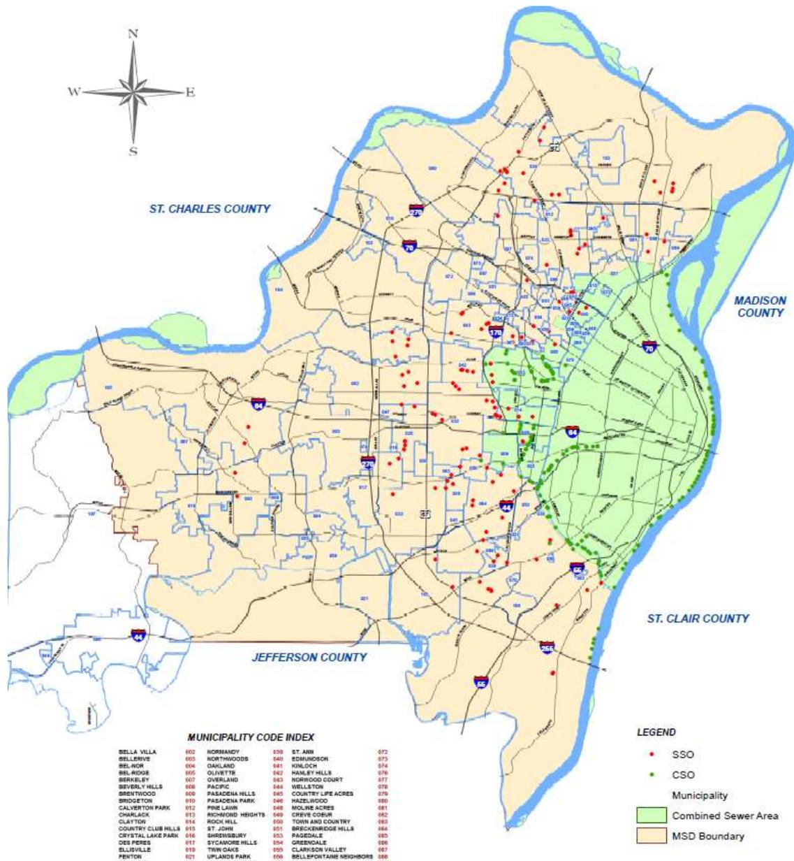
Figure 2: MSD Constructed Sewer Overflows Map
