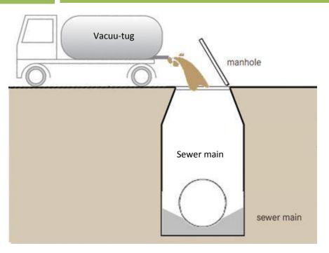
In cities that have an underground drainage system, sludge and effluent collected using vacuum emptiers is emptied into the sewer lines. The sludge and effluent is treated together with the sewage at STP.
