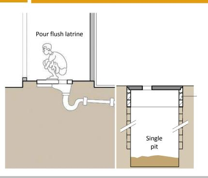
The collection system is widely prevalent and uses a single pit technology to collect and store excreta. Pits could be lined or left un-lined. The bottom of the pit is unlined to allow for the infiltration of liquids out of the pit into the soil. Depending on how deep they are , some pits may last 20 or more years without emptying.
