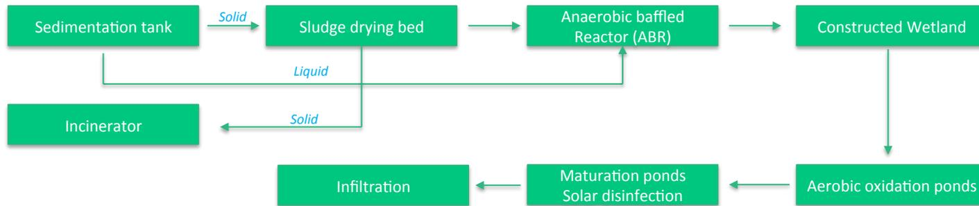
Figure 12. Sludge Treatment Plant in Sittwe (Solidarites International, 2018)
