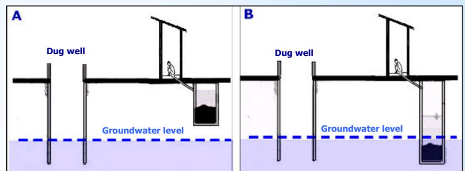
Fig. 2: Latrine pit above (A) and below (B) the groundwater level
