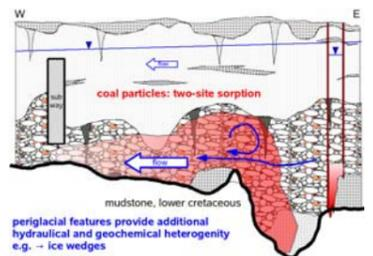
Fig. EW-schematic section to explain controlling processes in the CHC-plume of Hannover-Südstadt.
