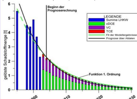
Fig. Prediction of Nat-Att. with transport, reaction and kinetic desorption from coal till 2030 for mass of diss. TCE, cDCE and VC (source: <sup>2)</sup>M & P)
