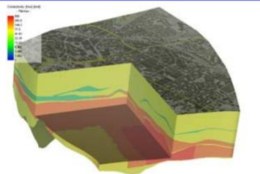
Fig. Subsurface model of the unconfined aquifer of glacio-fluvial origin (gravel, sand, silt-beds)
