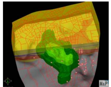
Fig. Model result: cDCE-plume will shrink from the border and concentration will fall but plume holds position (source: <sup>2)</sup>M & P, u.r. and m.r.)
