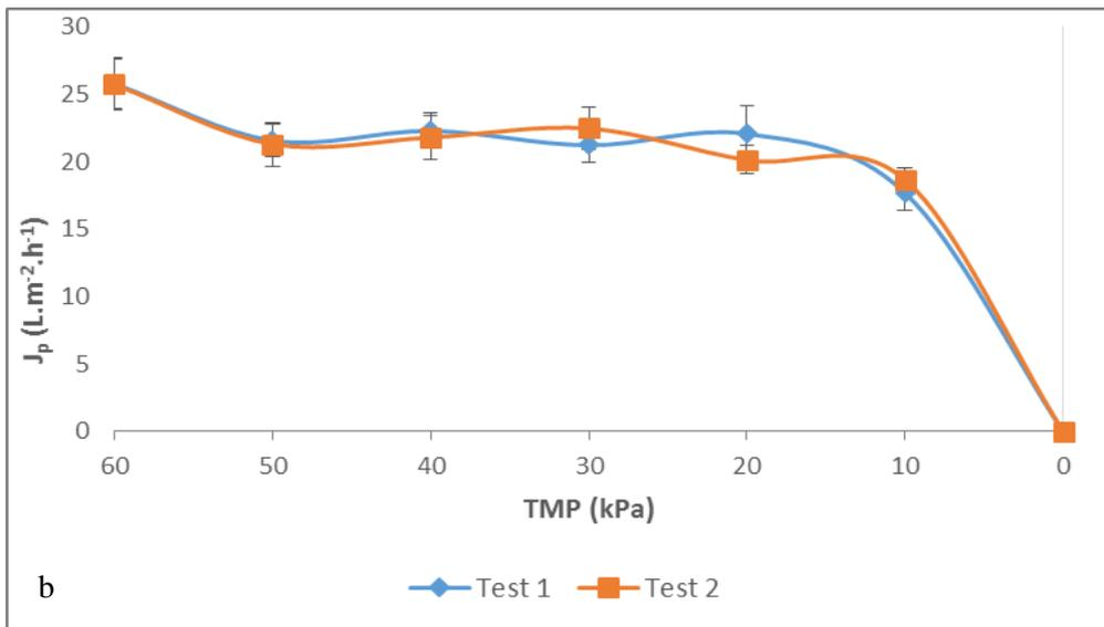
Figure C 2: Permeate flux at 20°C obtained during urine filtration for case 2 - a) membrane 4 ; b) membrane 5
