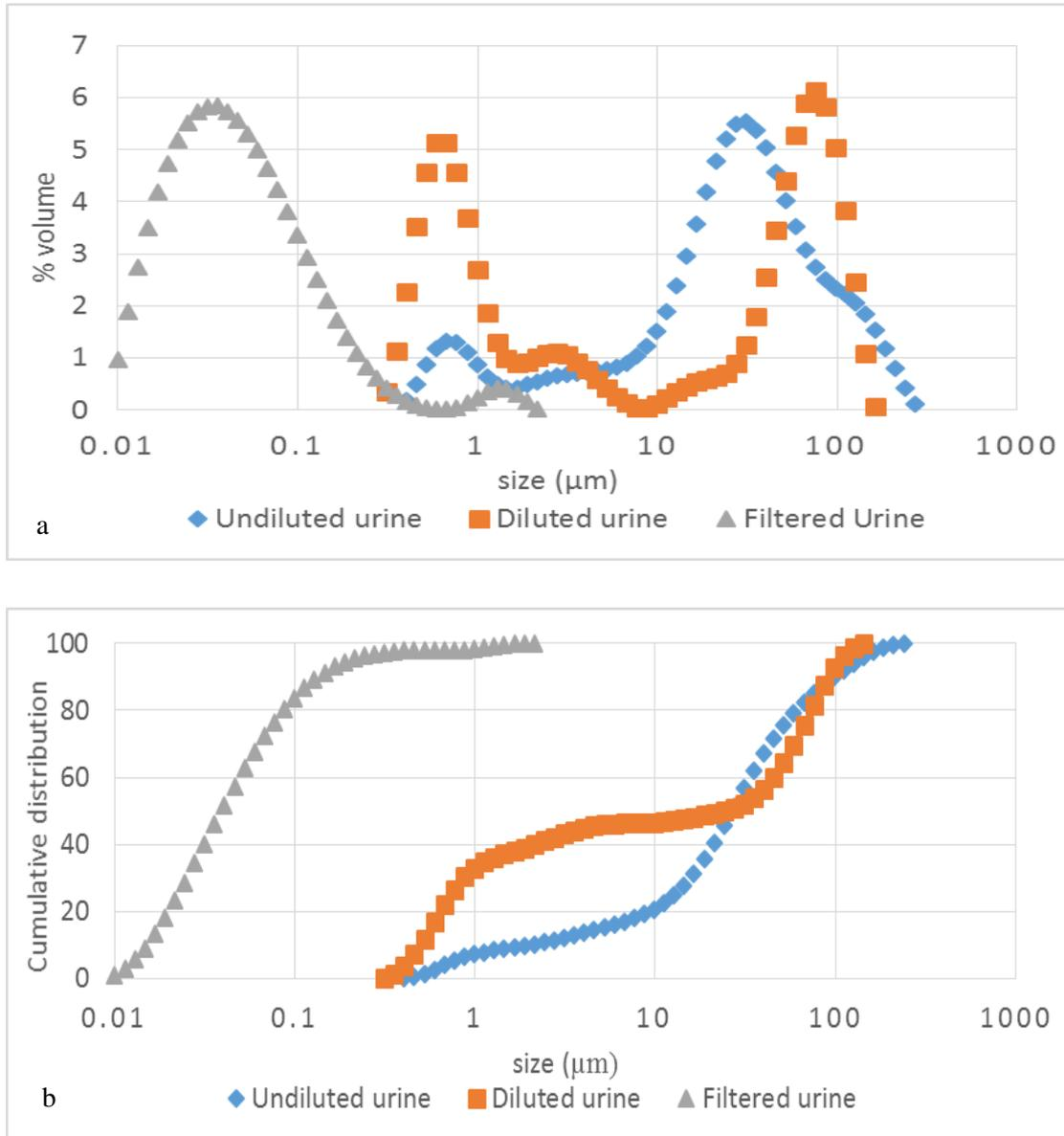
**Figure 4-12: Particle size distribution in the stored undiluted and diluted urine, and in the permeate - (a) volume distribution; (b) cumulative volume distribution**
