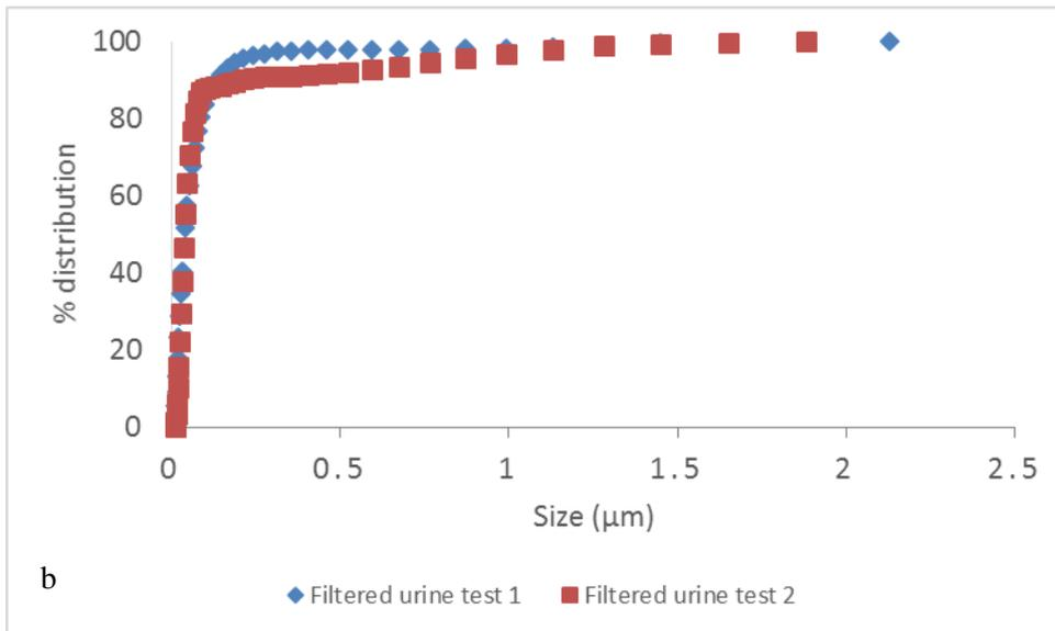
**Figure F 2: Particle size distribution of stored urine after filtration - (a) Volume distribution; (b) Cumulative volume distribution**
