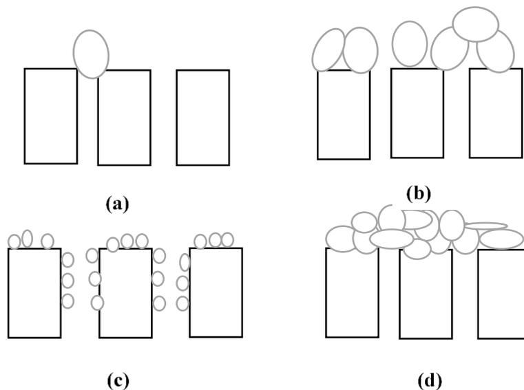
**Figure 2-2: Types of fouling : (a) complete blocking, (b) standard blocking, (c) intermediate blocking (adsorption) and (d) cake filtration (Judd, 2006)**
