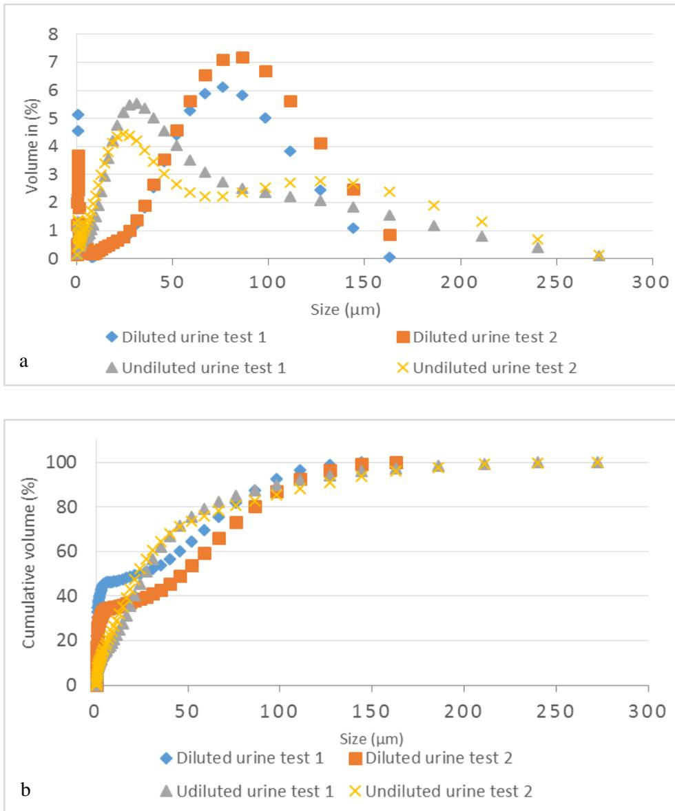
**Figure F 1: Particle size distribution of stored undiluted and diluted urine before filtration - (a) Volume distribution; (b) Cumulative volume distribution**
