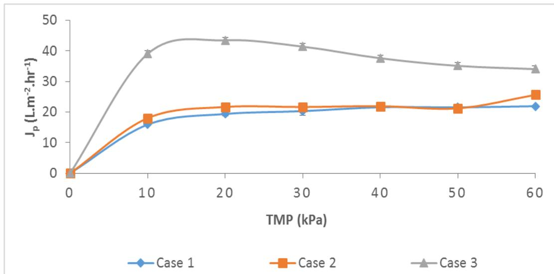
**Figure 4-1: Permeate flux at 20°C against transmembrane pressure for case 1 (urine flux 10-60 kPa), case 2 (urine flux 60-10 kPa) and case 3 (diluted urine flux)**
