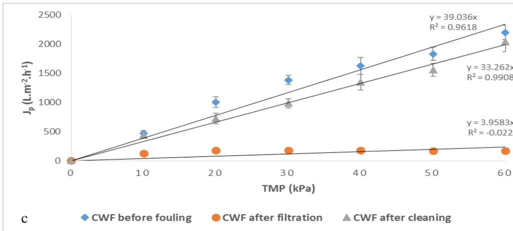
**Figure D 3: Clean water flux tests for the membranes used in case 3 – a) Membrane 6 ; b) Membrane 7 ; c) Membrane 8**
