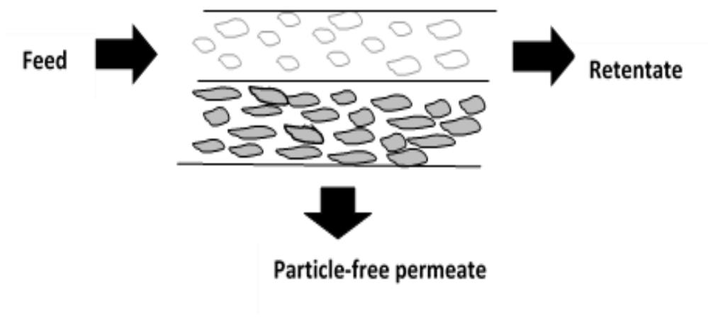
Figure 2-6: Cross flow filtration (Baker, 2012)
