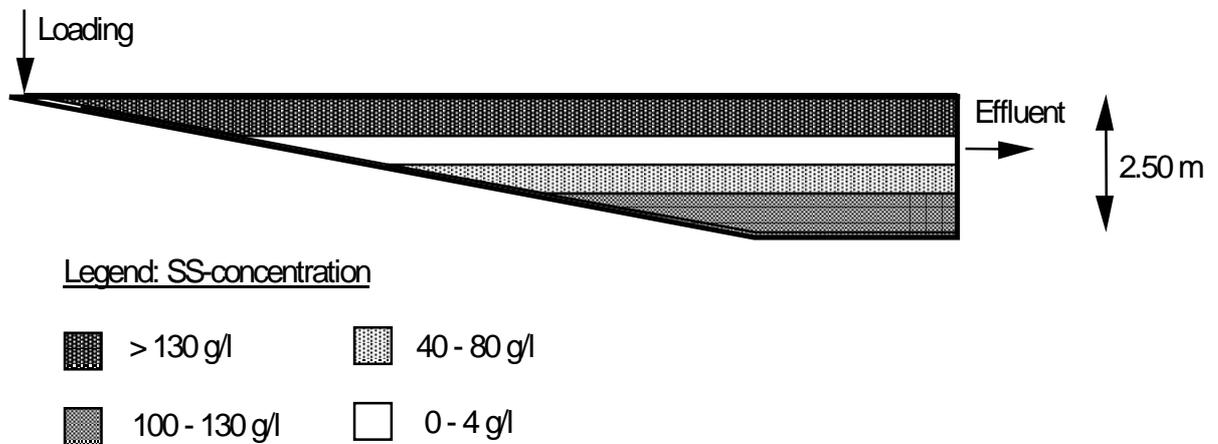
**Fig. 2:** Average SS concentration in a settling/ thickening tank after 4 weeks of operation and 1 week at rest (Achimota FSTP, Accra).
