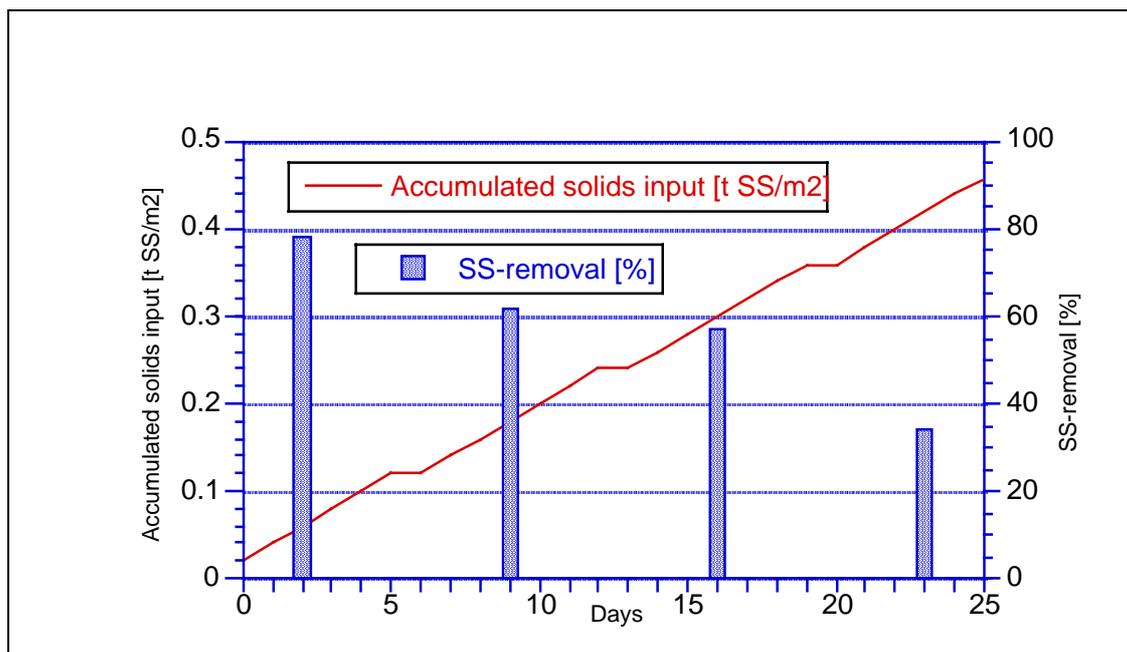
**Fig. 3:** Accumulated Solids Loading and Removal Efficiency in the Sedimentation/Thickening Tank as a Function of the Loading Duration
