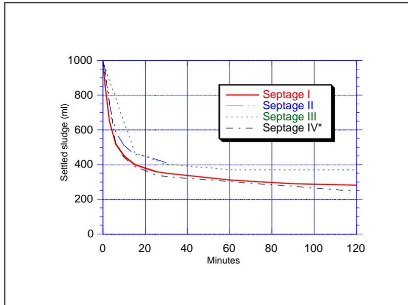
**Fig. 1:** Results of settling tests performed in 1-litre cylinders (septage I-III) and in a cylinder of 20 cm diameter and 2 m height (septage IV\*)
