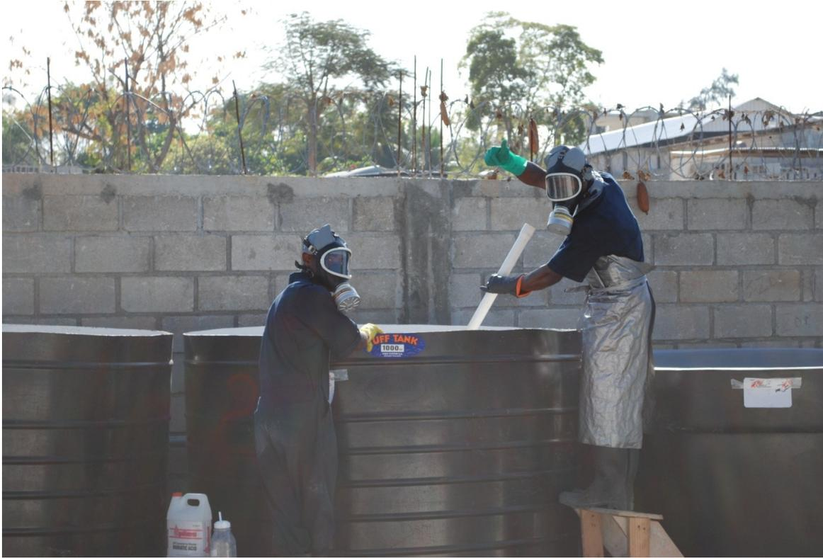
*Figure 2: Neutralisation process within a 3.8 m<sup>3</sup> 'Tuff Tank'*
