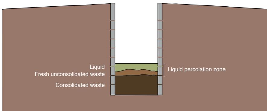
**Figure 6.** Liquid percolation zone in a pit latrine
