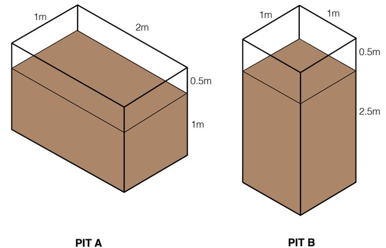
**Figure 6.** Two pits with the same total volume but a different effective volume
