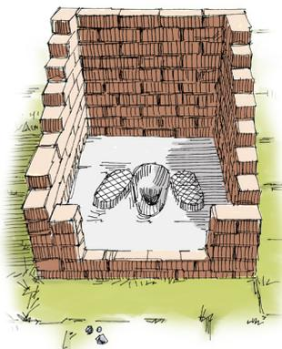
A latrine is a structure that contains a toilet and in some cases, somewhere to bathe. It is usually separate from a residence. The latrine slab is a platform over a vault with a drop hole or a flush pan into which a user excretes. The slab may incorporate a squat-plate with footrests or a seat on a pedestal.
