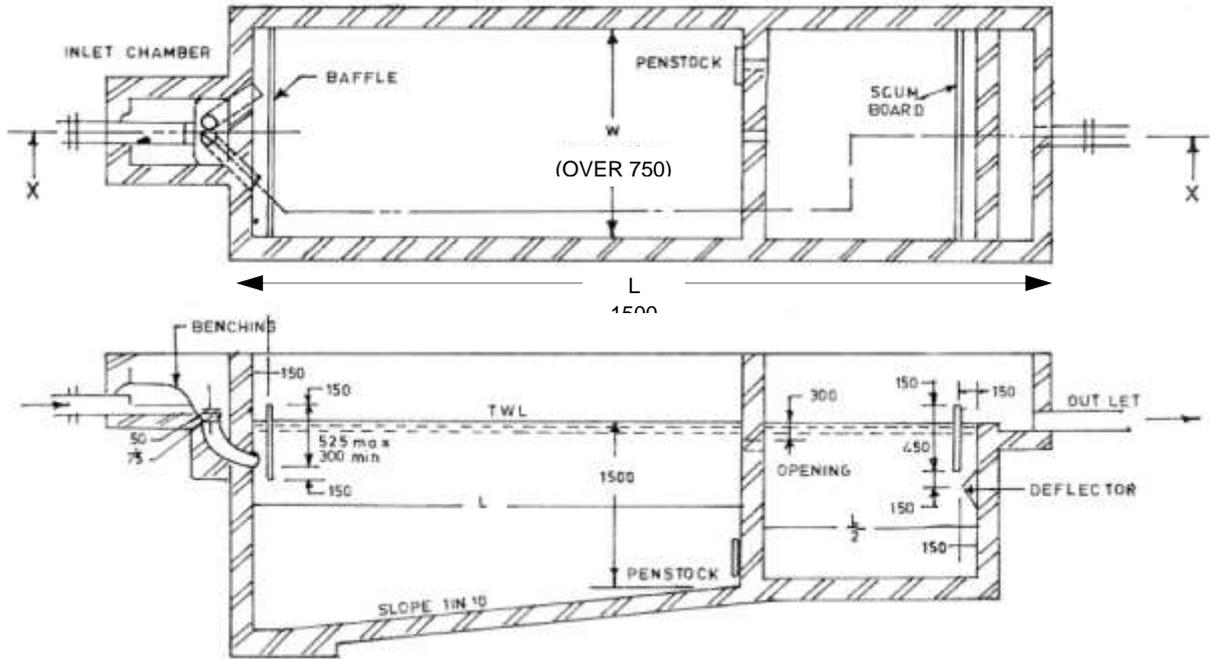
Figure 7: Details of bio-digester with reed bed
