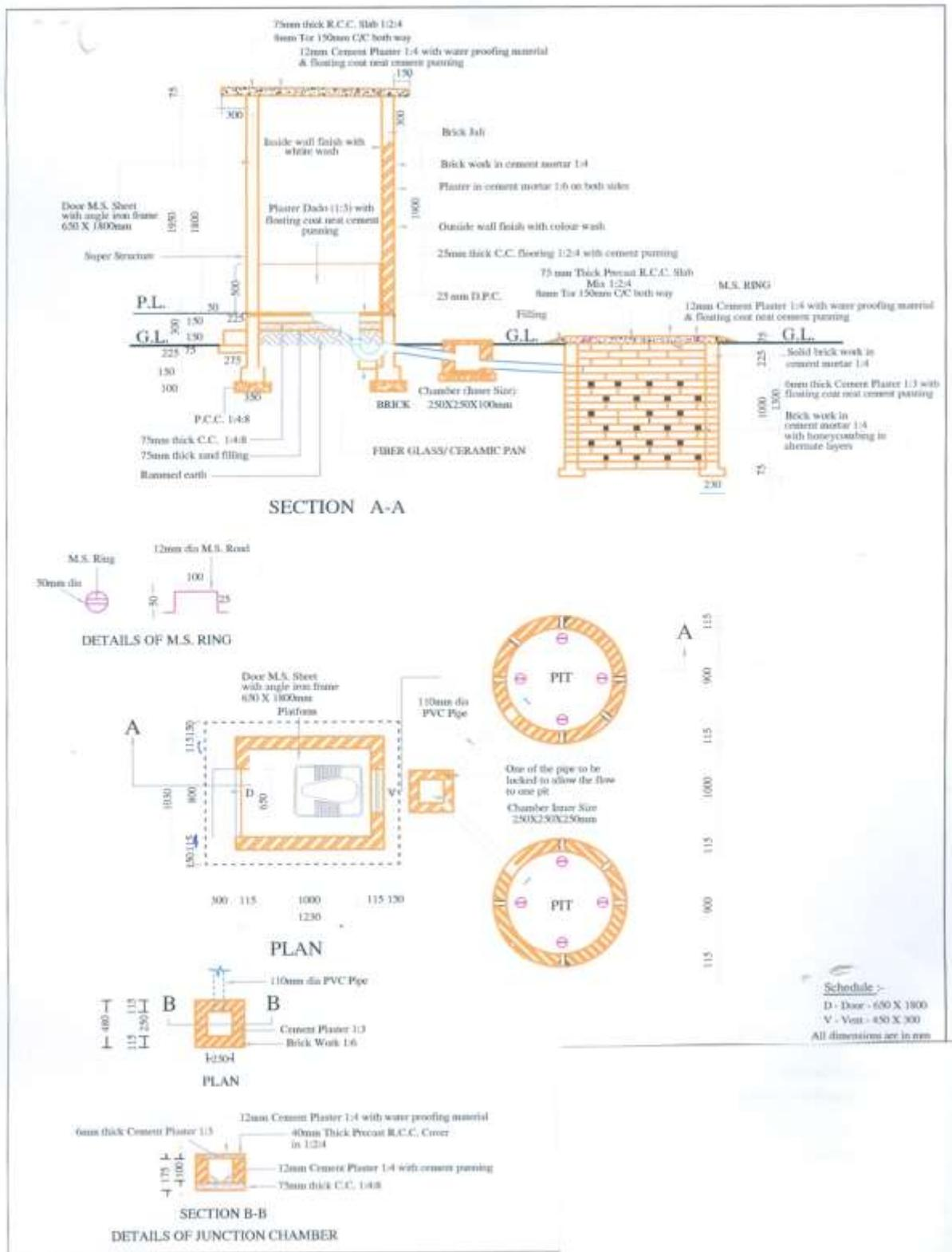
Figure 2: Pour-flush latrine with circular pits
