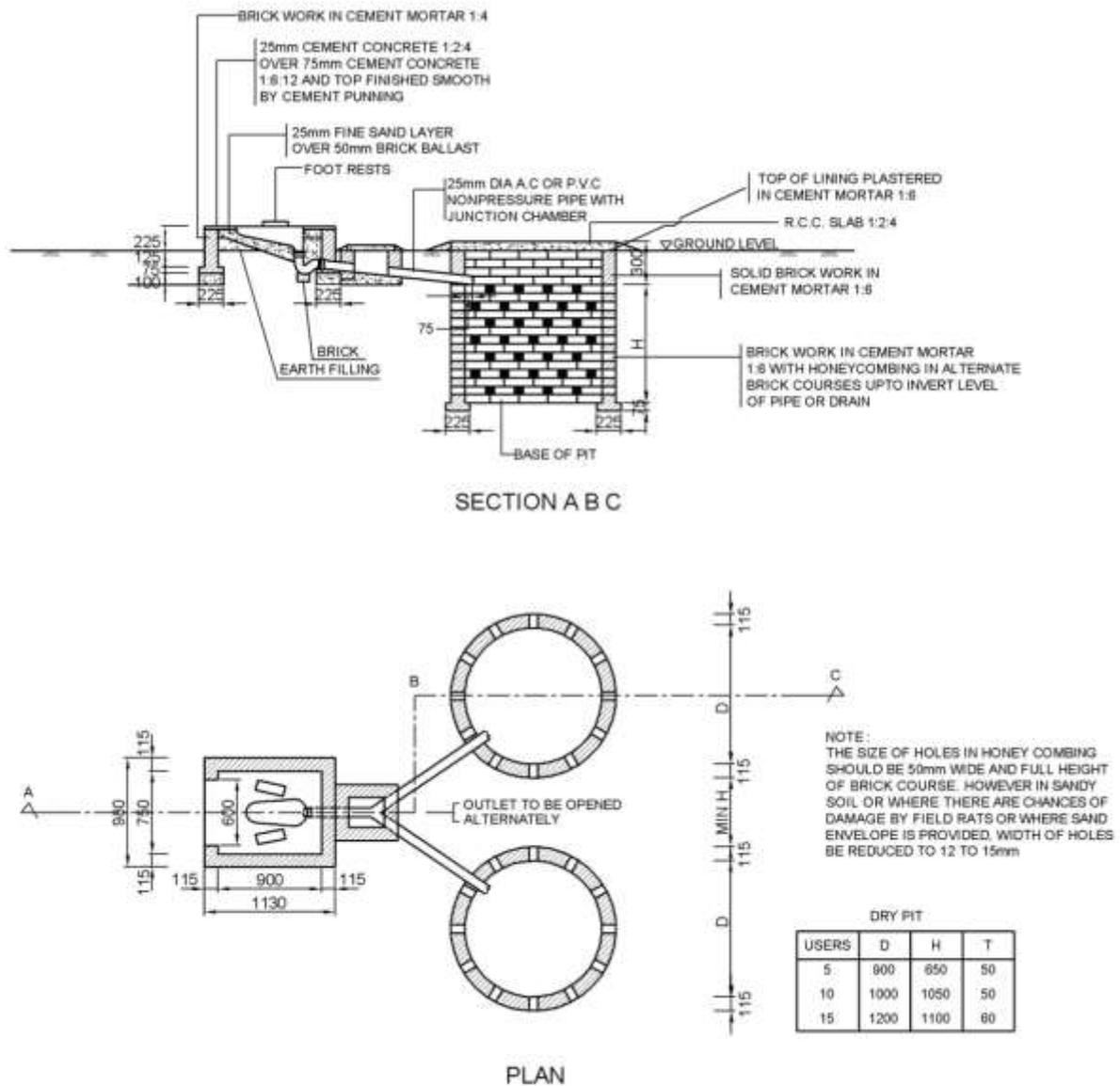
Figure 6: Typical sketch of two-compartment septic tank for 5 users
