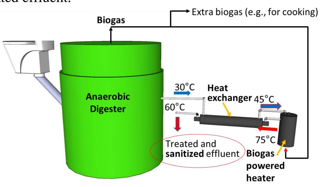
The concept was investigated in the lab with a 17 L floating dome anaerobic digester treating simulant feces and urine. An efficient biogas-powered pasteurization system was also developed. Key findings were that anaerobic digestion of undiluted human waste yields sufficient biogas to maintain
