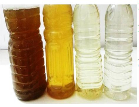
Left side: untreated sewage. 2<sup>nd</sup> : Partial treatment in bio digester, free of solid waste. > 3<sup>rd</sup> : properly treated in bio digester : good for agriculture and arboriculture. 4<sup>th</sup> : CWL treated with natural aerobic treatment: good for
