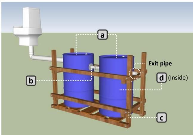
**Fig. 4:** Schematic drawing of a black water floating treatment system in the Amazon várzea.
