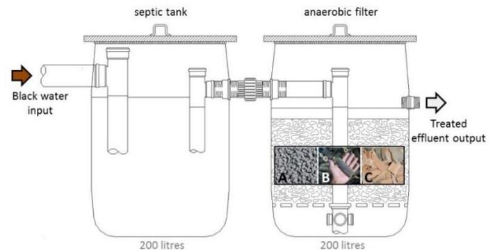
**Fig. 5:** Cross section of black water floating treatment system.
