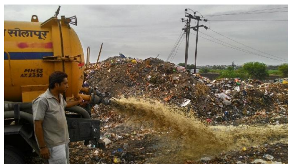
Figure 3: Disposal of septage in solid waste dump yard (Source: Rahul/CSE, 2015)
