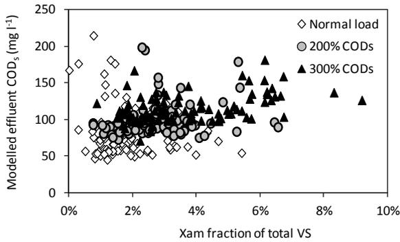
**Figure 166: Xam fraction of total VS in reactor at the end of each modelling iteration vs modelled effluent COD<sub>s</sub> concentration depending on feed concentration**
