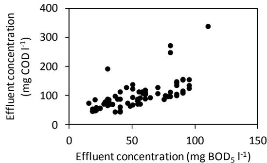
**Figure 23: COD vs. BOD<sub>5</sub> effluent concentrations**
