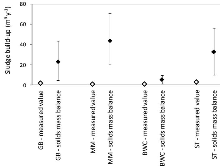
**Figure 146: Average sludge build-up rates observed in reactors and estimated through mass balance of particulate organics, error-bars represent confidence intervals taking a feed flow variation of 20%, the standard error of means of COD<sub>p</sub> concentrations and the standard deviation of sludge VS concentration data into account**
