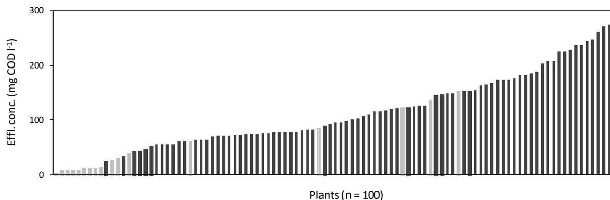
**Figure 38: Effluent  $\text{COD}_t$  concentrations and rain occurrence prior to sampling (light columns represent sites where it rained within 24 h prior to sampling) at visited plants with raw-water conductivity below  $6 \text{ mS cm}^{-1}$  (n=100)**
