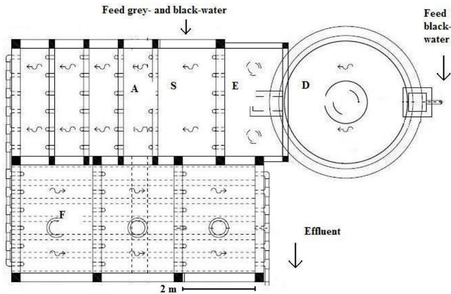
**Figure 83: Schematic diagram (top-view) of the DEWATS plant built in Gambiran/ Yogyakarta with biogas-digester (D), expansion chamber (E), settler (S), ABR (A), anaerobic filter (F); water-depth of the system: 2,000 mm**
