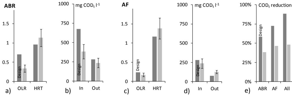
**Figure 97 a, b, c, d and e: Loading and treatment parameters of ABR and AF reactors: OLR, HRT, feed and effluent COD concentrations and COD reduction rates, OLR error-bars indicate combination of standard error of mean of COD<sub>t</sub> measurements and standard deviation of Q, all other error-bars indicate standard deviations of concentration measurement results**
