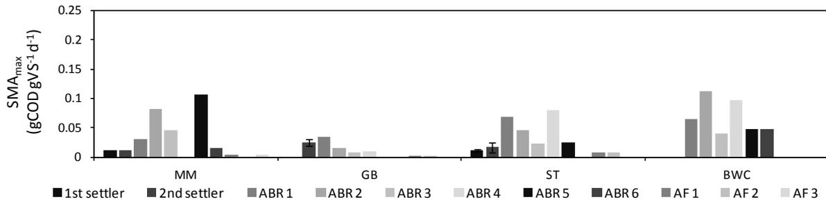
Figure 138: SMA<sub>max</sub> values measured across reactor chambers of the four case study plants during wet-season
