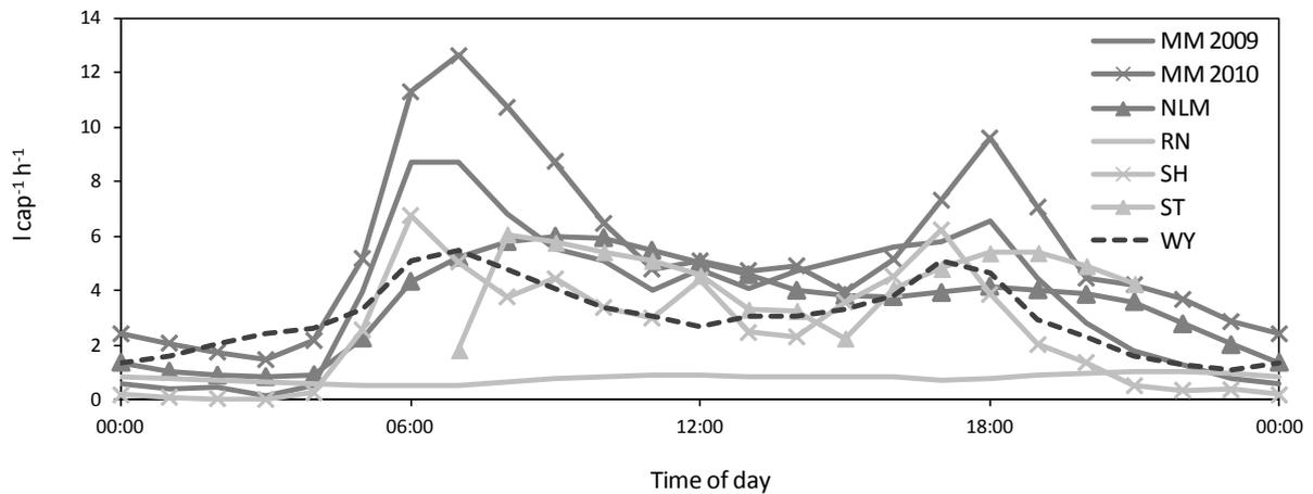
**Figure 22:** Average per capita diurnal flow fluctuations measured during seven measurement campaigns at six sites
