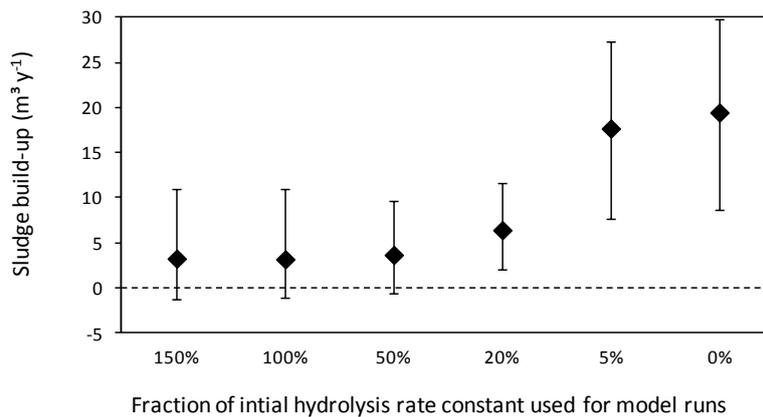
**Figure 160: Sensitivity of the modelled sludge build-up rate towards the hydrolysis rate constant, error-bars represent 95% confidence intervals of modelled outcomes after Monte-Carlo type uncertainty analysis taking into account the measured uncertainties of model input data, modelling runs done with GB data**
