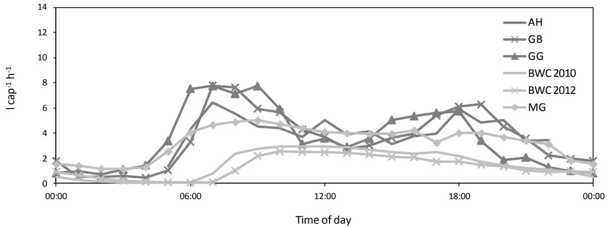
**Figure 21:** Average per capita diurnal flow fluctuations measured during six measurement campaigns at five sites
