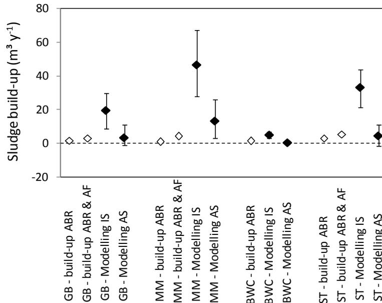
**Figure 159: Average sludge build-up rates in  $\text{m}^3 \text{y}^{-1}$ , field data (not full), modelled data (full), error-bars of full data points represent 95% confidence intervals of modelled outcomes after Monte-Carlo type uncertainty analysis taking into account the measured uncertainties of model input data**
