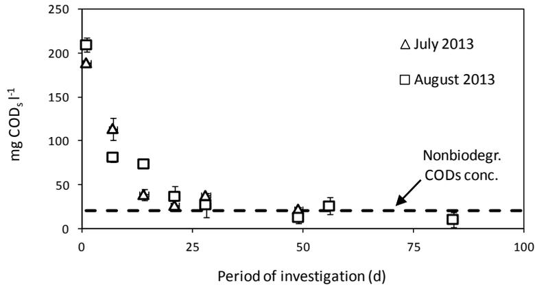
**Figure 183: Nonbiodegradable effluent COD<sub>5</sub> concentration measurements done on samples taken at three different dates at MM (indicated as month and year), data-points represent the averages of single and duplicate measurements on duplicate samples, error-bars indicate the standard deviation of these three values**
