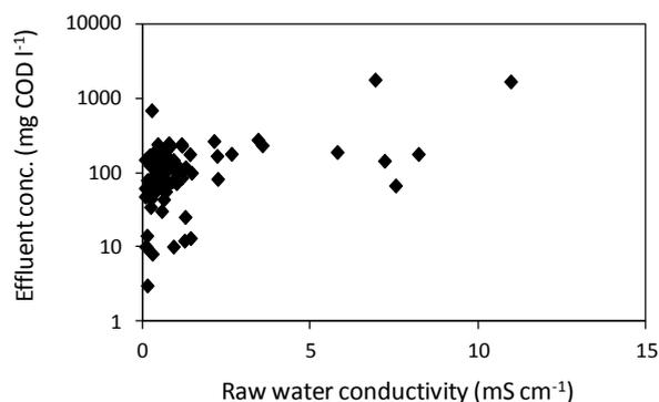
**Figure 33: DEWATS-effluent concentration vs. raw-water conductivity measurement results**
