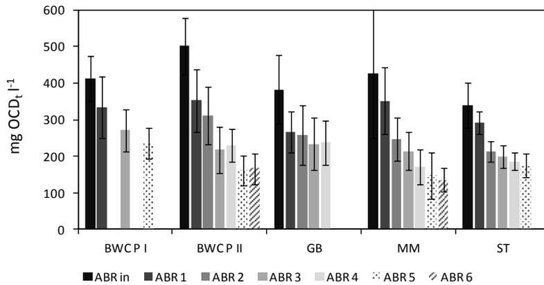
**Figure 147: Average COD<sub>t</sub> concentration profiles of the four plants and two phases in BWC, error-bars indicate standard deviations, all values exclude the plant specific nonbiodegradable COD<sub>s</sub> concentration**
