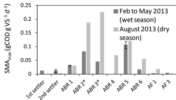
**Figure 107: SMA<sub>max</sub> of sludge sampled from different reactors in 2013, all sludges were processed within one week after sampling except when marked with \*: time between sampling and measurement is 15 d in February, error-bars indicate the standard deviation of duplicate sequential measurements, all other values are derived from single measurements**
