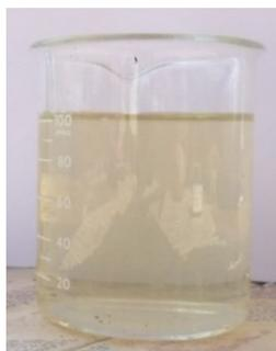
**Figure 35: Sample with measured COD concentration of  $1,649 \text{ mg COD}_t \text{ l}^{-1}$**
