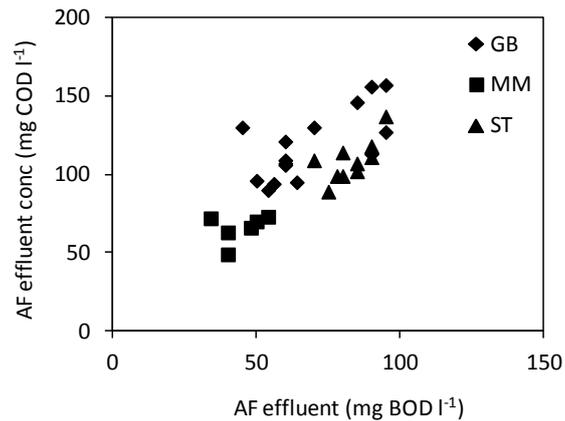
Figure 157: BOD<sub>5</sub> against COD AF effluent concentrations
