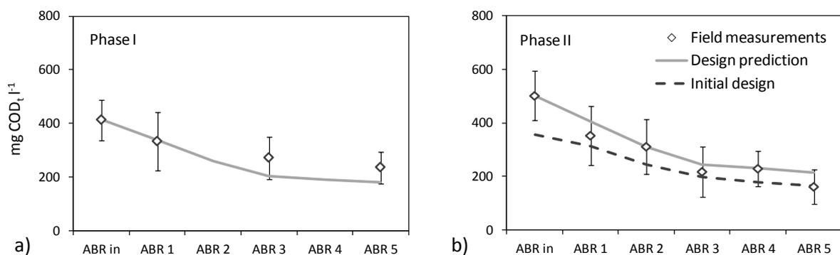
**Figure 82 a and b: Measured average  $\text{COD}_t$  concentration profiles in Phase I and II, initial design predictions („Initial design“) and design predictions with input variables adjusted to measured field values („Design prediction“)**
