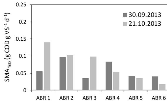
**Figure 72: SMA<sub>max</sub> values of sludge sampled from different reactors in 2013 at BWC, all sludges were processed within one week after sampling, all values were derived from single measurements**
