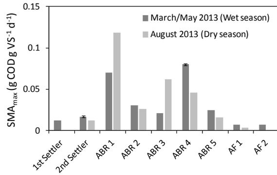
**Figure 122: SMA<sub>max</sub> of sludge sampled from different reactors in 2013, all sludge was processed within one week, error-bars indicate the standard deviation of duplicate measurements, all other values are derived from single measurements**
