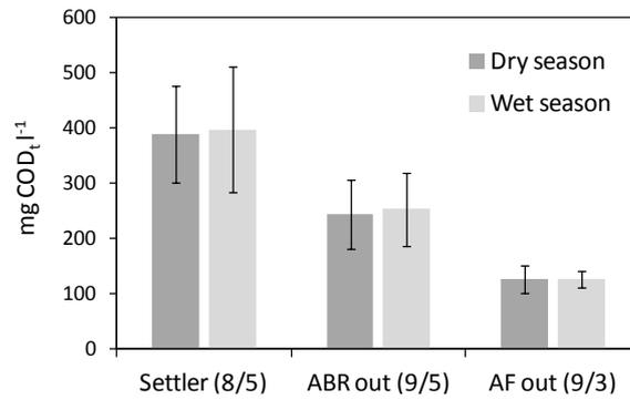
**Figure 92: Average COD<sub>t</sub> concentrations measured at settler effluent, ABR effluent and AF effluent, “dry season” is defined as the months May to September, “wet season” is defined as the months October to April, the numbers in brackets indicate the number of measurements made during dry and wet season respectively**
