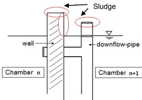
Criteria for exposure of an ABR to storm water were observations such as sludge on partition walls or on down flow pipes as shown in Figure 14.
