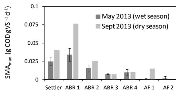
**Figure 89: SMA<sub>max</sub> of sludge sampled from different reactors in 2013, all samples were processed within one week after sampling, error-bars indicate the effect of the VS measurement standard deviation in May 2013 which was high (> 10%), all values are derived from single measurements**
