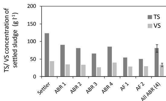
**Figure 88: Settled sludge TS and VS concentration profiles, single measurements, "All ABR" bars represent averages of all ABR values, error-bars indicate the standard deviations across all ABR values**
