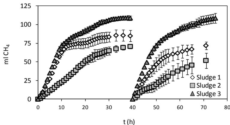
**Figure 175: Cumulative CH<sub>4</sub> production with second substrate addition after 40 h, data points are averages of triplicates and control has been subtracted, error-bars indicate the sum of standard deviations of triplicate tests and triplicate controls, the theoretical maximal CH<sub>4</sub> production is 100 ml CH<sub>4</sub>, sludge samples: ABR 4 and ABR 5, Santan, ABR 5, Minomartani**
