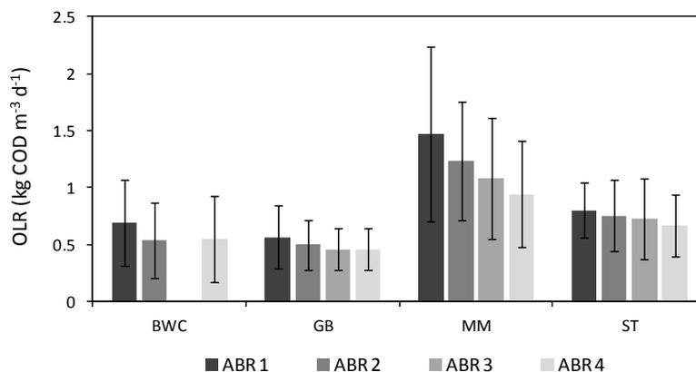
**Figure 145:** Biodegradable soluble OLRs of single ABR chambers of the four plants, error-bars indicate the standard deviation of COD<sub>s</sub> concentration measurements and a 20% variation of Q
