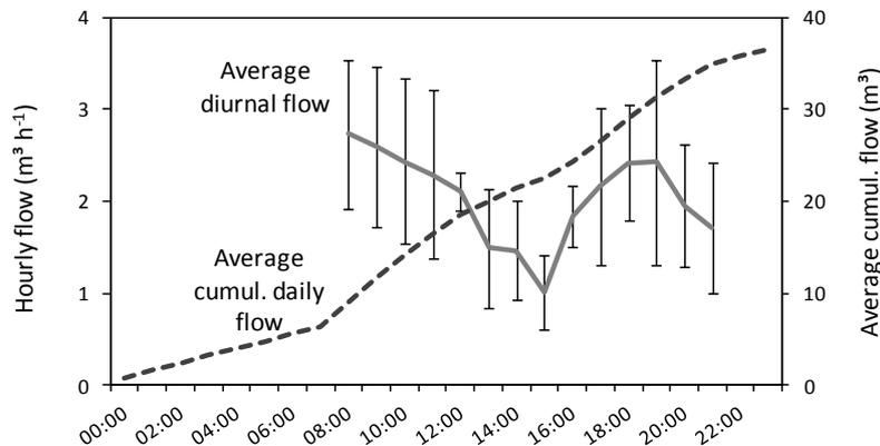
**Figure 118: Average flows as measured in 2013, averages were calculated with data from 7 d (19.09.2013 to 25.09.2013), error-bars indicate the standard deviation of hourly flows over that period, no rain**
