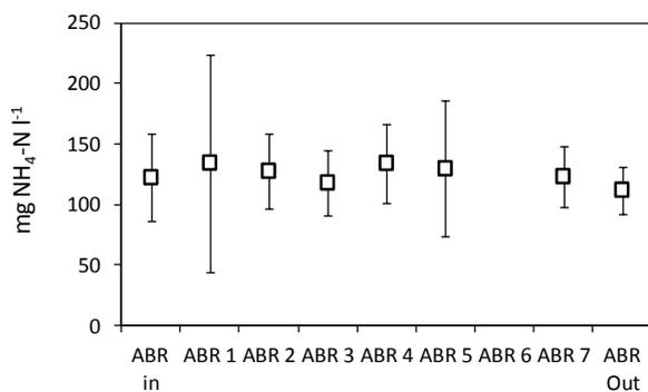
**Figure 76: Average wastewater NH<sub>4</sub>-N concentration profile across reactor chambers as measured in Phase I, error-bars indicate standard deviations, 4 to 23 data points per sampling point**
