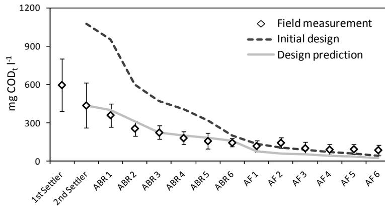
**Figure 114: Measured average  $\text{COD}_t$  concentration profile, initial design prediction („Initial design“) and design prediction with input variables adjusted to measured field values („Design prediction“)**
