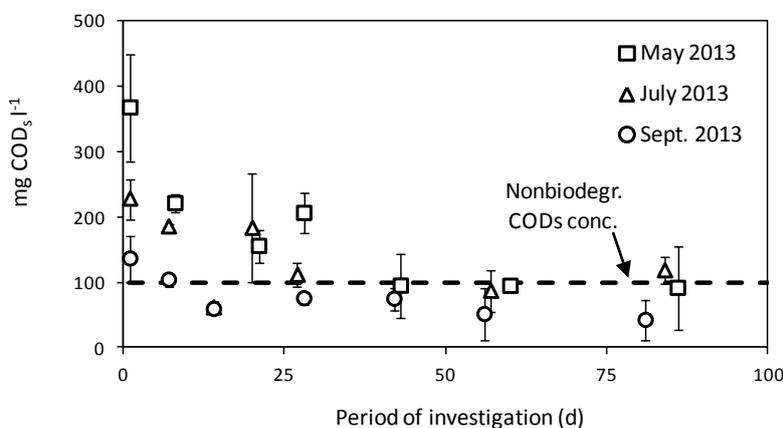
**Figure 181: Nonbiodegradable effluent COD<sub>5</sub> concentration measurements done on samples taken at three different dates at BWC (indicated as month and year), data-points represent the averages of duplicate measurements on duplicate samples, error-bars indicate the standard deviation of these four values**
