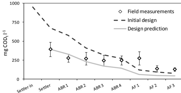
**Figure 98: Measured average  $COD_t$  concentration profile, initial design prediction („Initial design“) and design prediction with input variables adjusted to measured field values („Design prediction“)**
