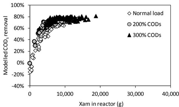
**Figure 168: Xam in reactor at the end of each modelling iteration vs modelled COD<sub>s</sub> removal depending on feed concentration**
