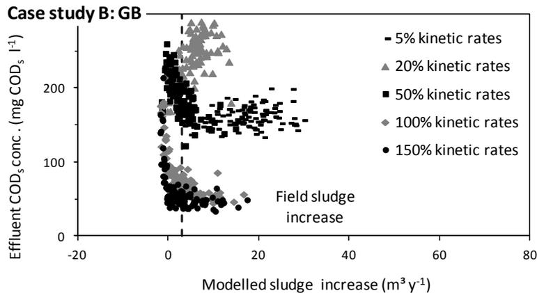
**Figure 163: Sensitivity of the modelled effluent COD<sub>s</sub> concentration towards the hydrolysis rate and methanogenesis growth rate constant, modelling runs done with GB data**
