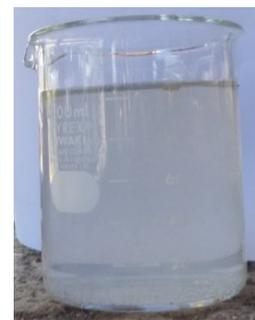
**Figure 37: Sample with measured COD concentration of  $416 \text{ mg COD}_t \text{ l}^{-1}$**
