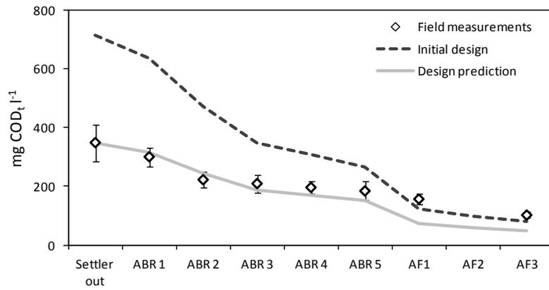
**Figure 130: Measured average COD<sub>t</sub> concentration profile, initial design prediction („Initial design“) and design prediction with input variables adjusted to measured field values („Design prediction“)**
