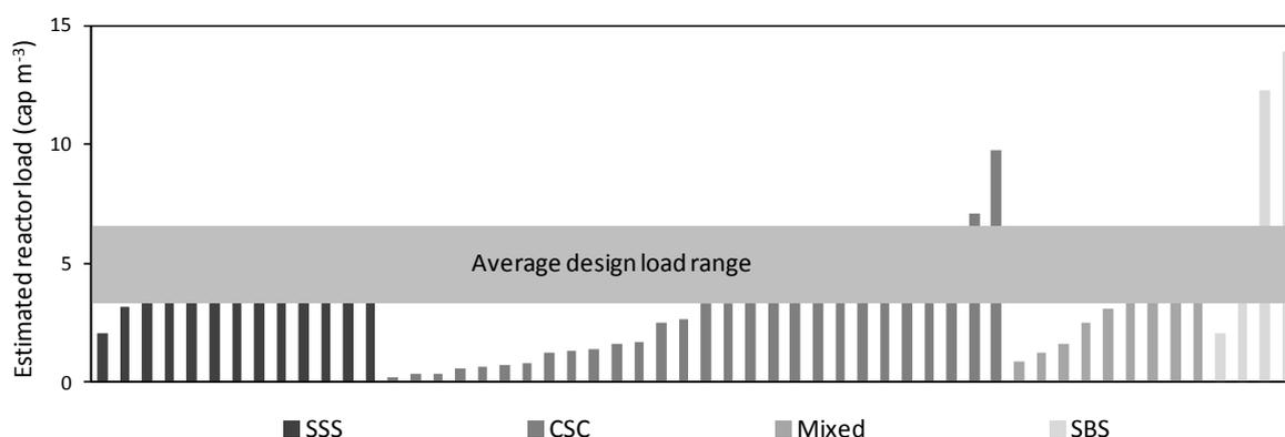
**Figure 41: Loading estimation of plants (n = 54), the confidence range of the average design load is computed with the average load of 4.9 and the standard deviation of 1.6 cap m<sup>-3</sup> (see Section 5.2.6)**
