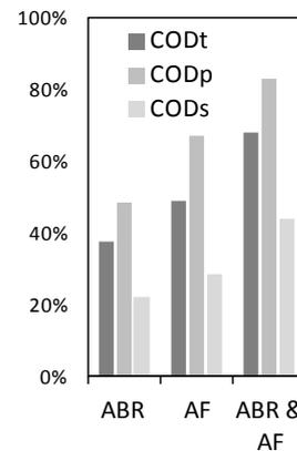
**Figure 96: Average removal rates of COD fractions in ABR and AF**
