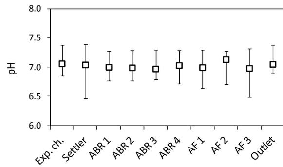
**Figure 91: Maximum, median pH profiles across reactor chambers as measured from 2009 to 2013, error-bars indicate min and max values, 8 to 13 data points per sampling point**
