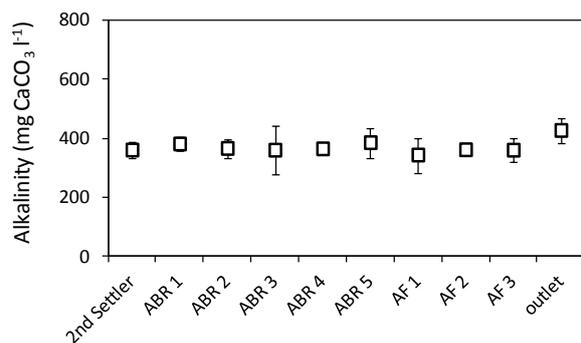
**Figure 123: Average alkalinity concentration profile across reactor chambers as measured from 2012 to 2013, error-bars indicate standard deviation, 2 to 6 data points per sampling point**
