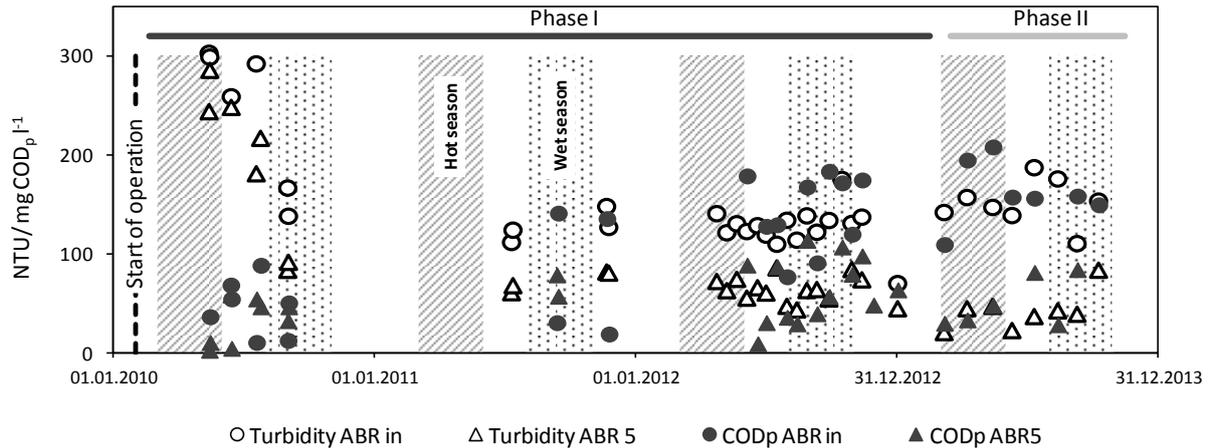
**Figure 77: ABR<sub>in</sub> and ABR 5 turbidity and COD<sub>p</sub> concentrations, the light red areas indicate the warmest period of the year, the light blue areas indicate the wettest period of the year**
