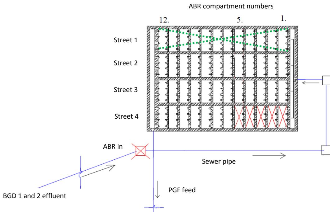
**Figure 60: Top view and selection of sampling points (crosses) of the ABR at BWC, sewer pipes and four parallel ABR streets, the dashed line indicates the ABR street that was shut off in 2012 in order to increase the load to the remaining two streets, water depth of system 1,800 mm, Figure adapted from Miller (2011)**
