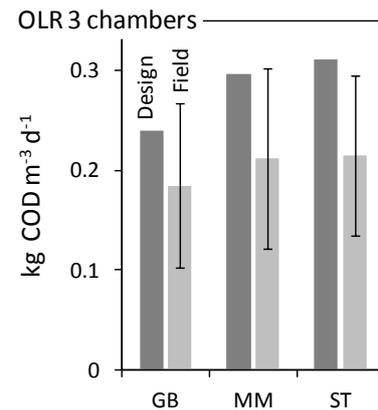
**Figure 154: Average AF OLRs (three chambers) of three plants, error-bars indicate standard error of COD<sub>t</sub> conc. measurements and a 20% variation of Q**
