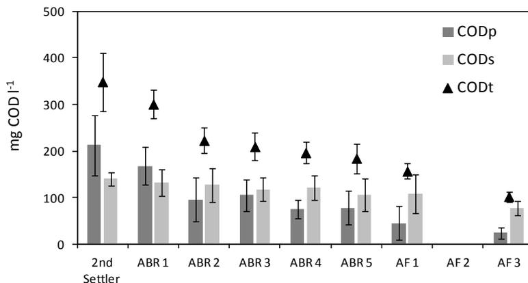
**Figure 127: Average total, particulate and soluble COD profiles across reactor chambers as measured from 2011 to 2013, averages were calculated with 9 to 10 data points per sampling point, error-bars indicate standard deviation**
