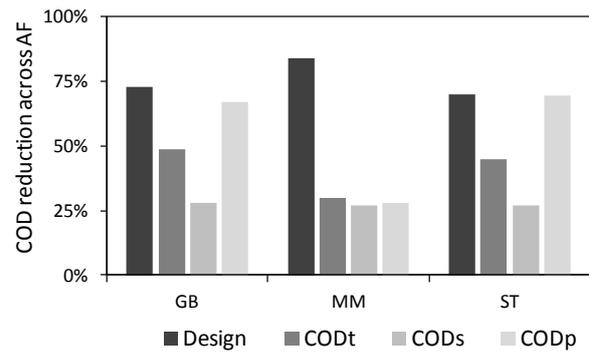
**Figure 156: Average COD<sub>t</sub>, COD<sub>s</sub> and COD<sub>p</sub> AF reduction rates of three plants**
