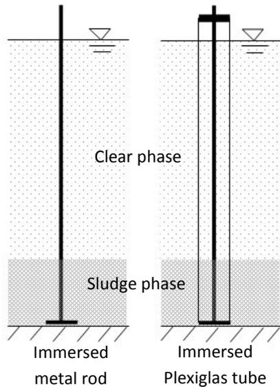
**Figure 15: Schematic depiction of the sludge core sampler as used in this study, cross section of a reactor chamber containing sludge**
