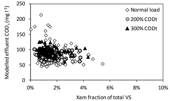
**Figure 167: Xam fraction of total VS in reactor at the end of each modelling iteration vs modelled effluent COD<sub>t</sub> concentration depending on feed concentration**
