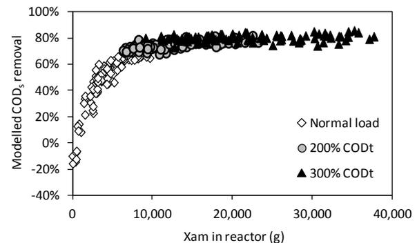
**Figure 169: Xam in reactor at the end of each modelling iteration vs modelled COD<sub>t</sub> removal depending on feed concentration**
