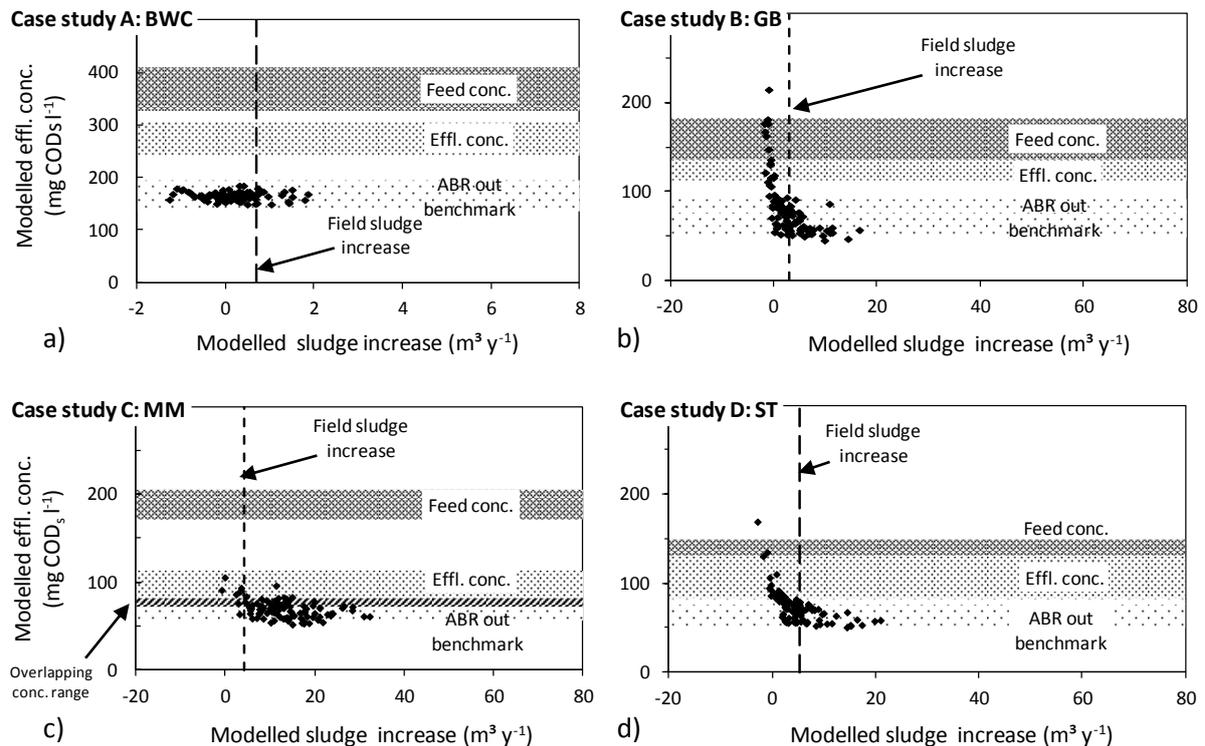
**Figure 162 a, b, c and d: Modelled sludge increase representing active anaerobic treatment vs. effluent COD<sub>s</sub> concentration. The red and blue horizontal bands represent the 95% confidence intervals of measured feed and effluent COD<sub>s</sub> concentration means respectively, the grey horizontal band highlights the benchmark effluent COD<sub>s</sub> concentration given by the model**
