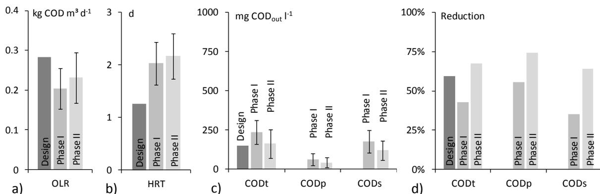
**Figure 81 a, b, c and d: Loading and treatment parameters of the first five ABR chambers in Phase I and II: OLR, HRT, effluent COD concentrations and COD reduction rates, OLR error-bars indicate combination of standard error of mean of  $COD_t$  measurements and standard deviation of Q, all other error-bars indicate standard deviations**
