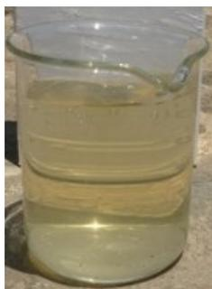
**Figure 34: Sample with measured COD concentration of  $1,747 \text{ mg COD}_t \text{ l}^{-1}$**
