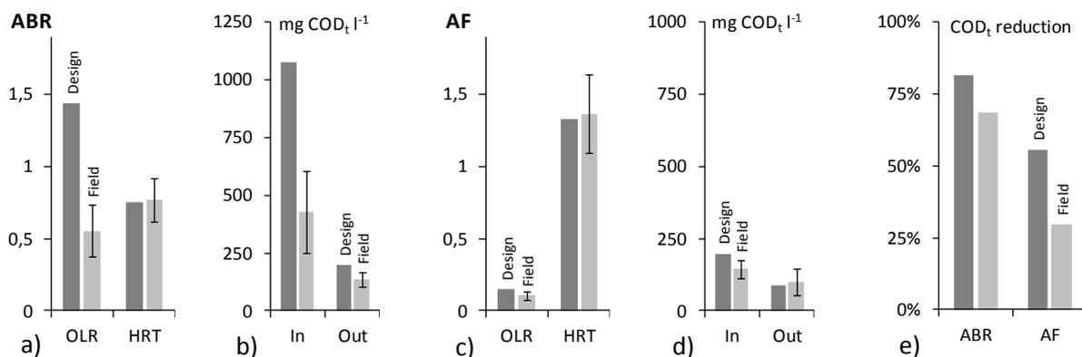
**Figure 113 a, b, c, d and e: Loading and treatment parameters of ABR and AF reactors: OLR, HRT, feed and effluent COD concentrations and COD reduction rates, OLR error-bars indicate combination of standard error of mean of  $COD_t$  measurements and standard deviation of  $Q$ , all other error-bars indicate standard deviations**
