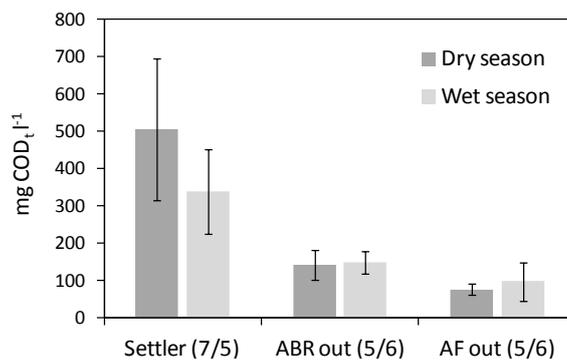
**Figure 110: Average COD<sub>t</sub> concentrations measured at settler effluent, ABR effluent and AF effluent, “dry season” is defined as the months May to September, “wet season” is defined as the months October to April, the numbers in brackets indicate the number of measurements made during dry and wet season respectively**
