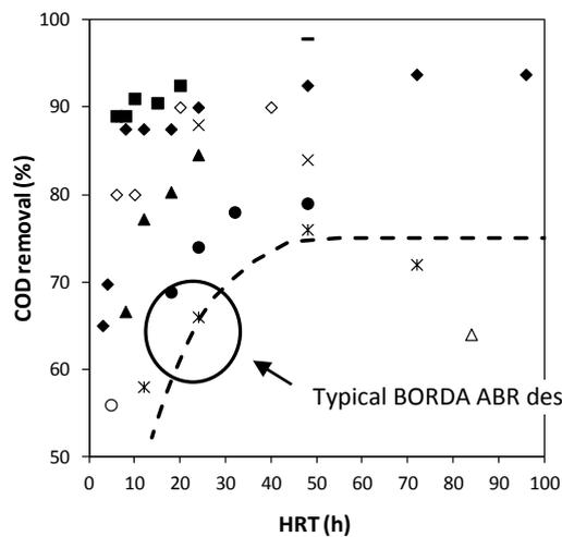
**Figure 11: Performance efficiency against various hydraulic retention times**
