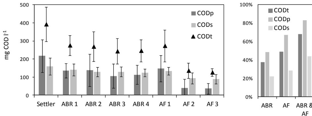
**Figure 95: Average total, particulate and soluble COD profiles across reactor chambers as measured from 2009 to 2013, averages are calculated with 12 to 15 data points per sampling point, error-bars indicate standard deviations**
