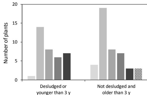
**Figure 53: Histograms for the effluent concentration frequency distribution depending on desludging**
