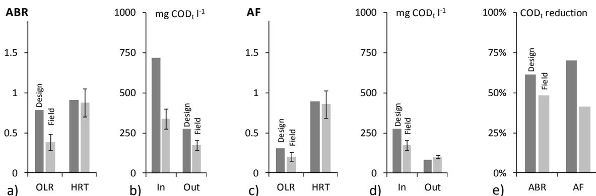
**Figure 129 a, b, c, d and e: Loading and treatment parameters of ABR and AF reactors: OLR, HRT, feed and effluent COD concentrations and COD reduction rates, OLR error-bars indicate combination of standard error of mean of  $COD_t$  measurements and standard deviation of  $Q$ , all other error-bars indicate standard deviations**
