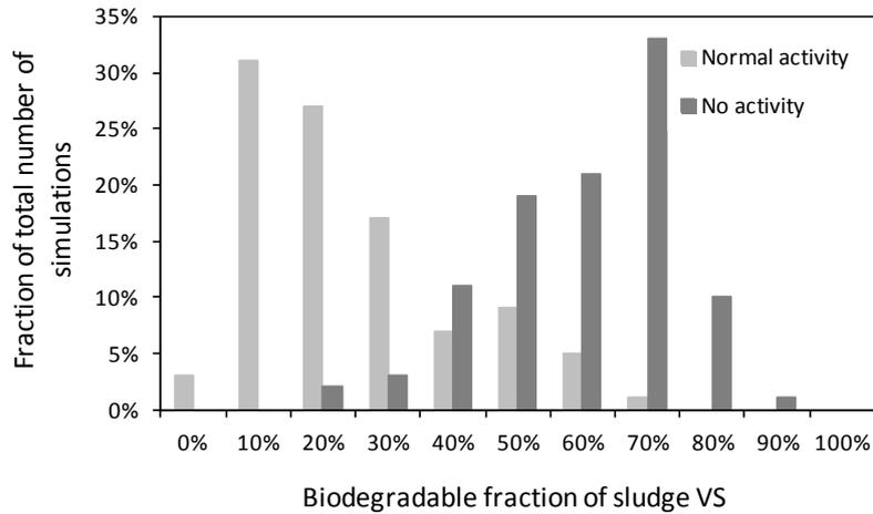
**Figure 161: Biodegradable sludge VS fraction vs sludge activity, probability distribution as given by model uncertainty analysis, modelling runs done with GB data**
