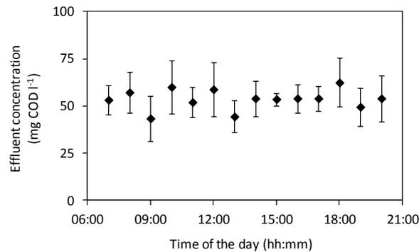
**Figure 24: Average hourly effluent COD-concentrations from hourly measurements done on five consecutive days from the 19<sup>th</sup> to the 23<sup>rd</sup> of July, 2008 in Minomartani, Indonesia, error-bars indicate the standard deviation of hourly measurements (Reynaud, 2008)**
