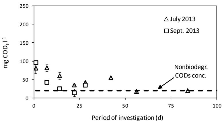
**Figure 182: Nonbiodegradable effluent COD<sub>5</sub> concentration measurements done on samples taken at three different dates at GB (indicated as month and year), data-points represent the averages of single and duplicate measurements on duplicate samples, error-bars indicate the standard deviation of these three values**
