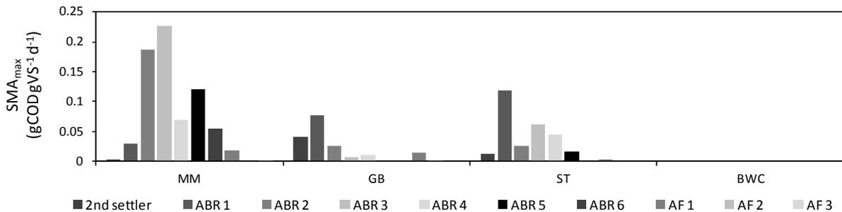
Figure 139: SMA<sub>max</sub> values measured across reactor chambers of three case study plants during dry-season
