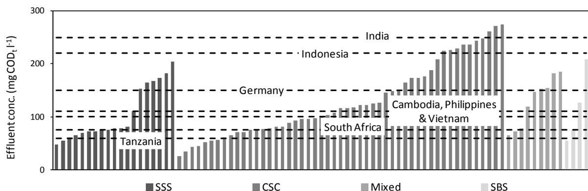
**Figure 39: Effluent  $COD_t$  values at visited plants not affected by rain water and with raw-water conductivity below  $6 \text{ mS cm}^{-1}$  ( $n = 82$ ), the dotted red lines represent national standard discharge COD concentration values for various countries**
