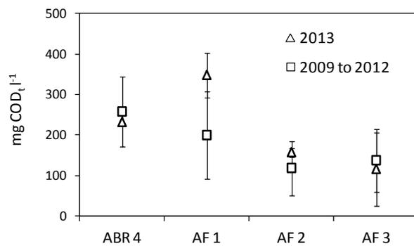
**Figure 94: Comparing COD<sub>t</sub> concentration profiles across AF chambers measured in 2013 and before September 2013**
