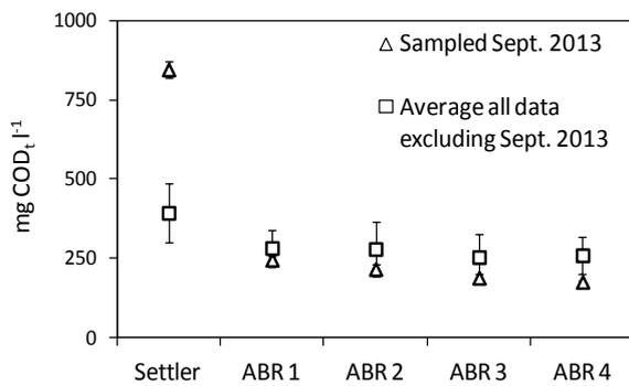
**Figure 93: COD<sub>t</sub> concentration profiles across ABR chambers and outlier value measured in September 2013**
