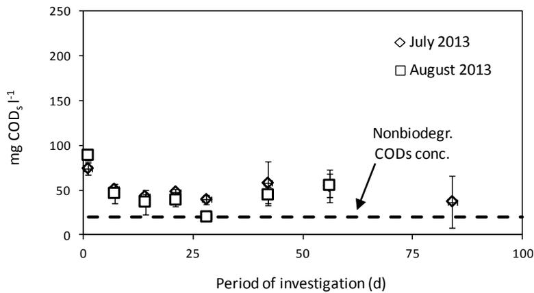
**Figure 184: Nonbiodegradable effluent COD<sub>5</sub> concentration measurements done on samples taken at three different dates at ST (indicated as month and year), data-points represent the averages of single and duplicate measurements on duplicate samples, error-bars indicate the standard deviation of these three values**
