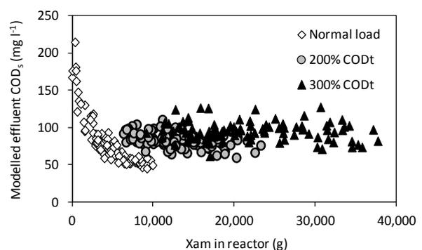
**Figure 165: Xam in reactor at the end of each modelling iteration vs modelled effluent  $\text{COD}_t$  concentration depending on feed concentration**
