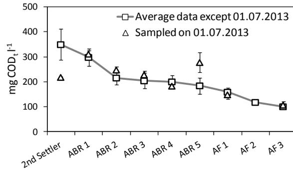
**Figure 126: COD<sub>t</sub> concentration profiles across ABR chambers and outlier values measured in July 2013**
