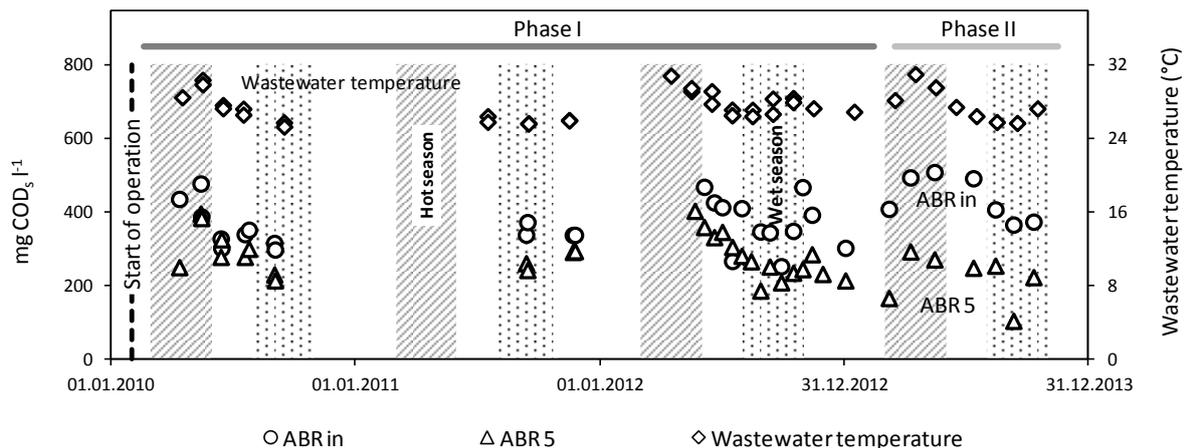
**Figure 78: ABR<sub>in</sub> and ABR 5 COD<sub>s</sub> concentrations and measured wastewater temperature, the light red areas indicate the warmest period of the year, the light blue areas indicate the wettest period of the year**
