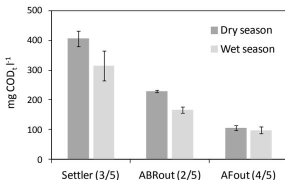
**Figure 125: Average COD<sub>t</sub> concentrations measured at settler effluent, ABR effluent and AF effluent, “dry season” is defined as the months May to September, “wet season” is defined as the months October to April, the numbers in brackets indicate the number of measurements made during dry and wet season respectively**
