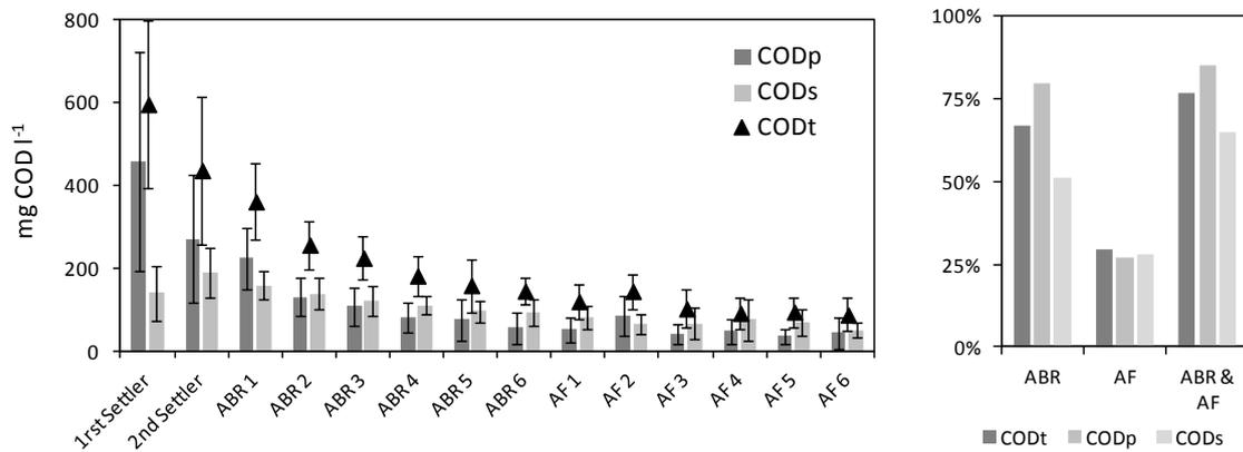
**Figure 111: Average total, particulate and soluble COD profiles across reactor chambers as measured from 2010 to 2013, averages were calculated with 6 to 12 data-points, error-bars indicate standard deviations**
