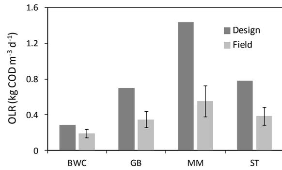
**Figure 144:** Average ABR OLRs of the four plants, error-bars indicate the standard error of COD<sub>t</sub> concentration measurements and a 20% variation of Q
