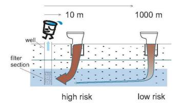
Figure 1: Example for high and low risk due to different horizontal separation distances.
