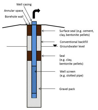
Figure 3: Example for placement of sealings.
