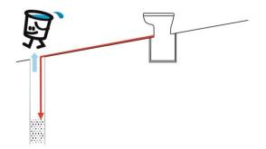
Figure 7: Example for strong increase in risk: septic tank 20 m uphill of the water supply well which does not have a properly constructed sanitary sealing /defect headworks.
