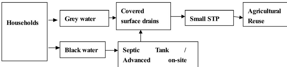
**Option-6: (Sanitation system using covered surface drains)**
