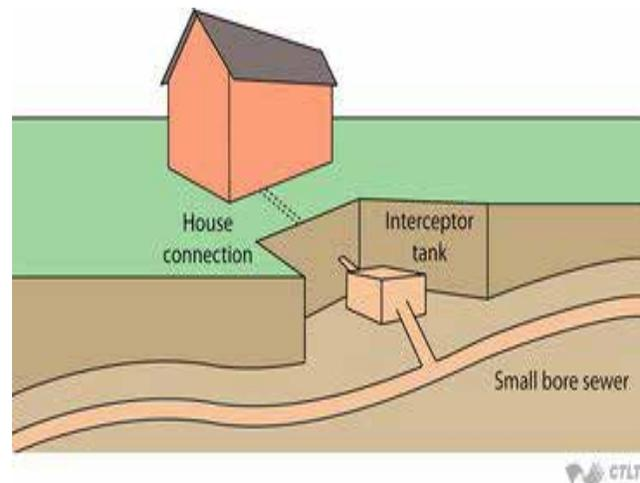
Figure 2.2: A schematic diagram of Small bore sewer (Source: Website Jhsphopen Courseware, 2013)
