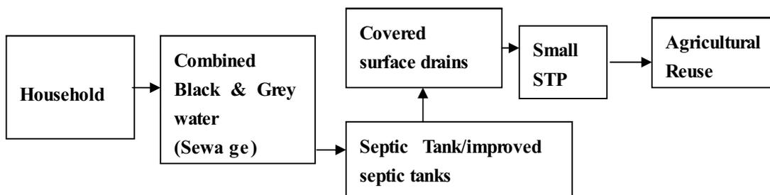
**Option-7: (Partly Sewered sanitation using small bore sewer)**
