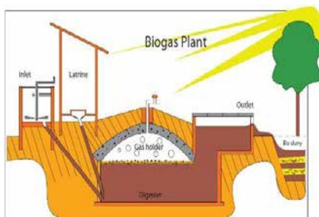
Fig. 3.10 A section of family size biogas plant of Deenbandhu Model (Source: Grassrootindia.com2013)
