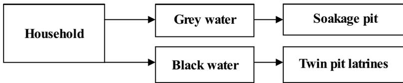
**Option-2: Sanitation System using Soak pits (Sandy soil and deep groundwater table, piped water supply sparse population)**
