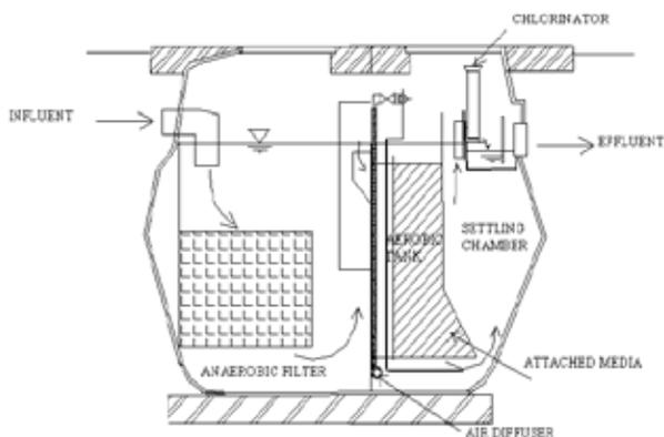
Figure 2.12. Typical cross-sectional drawings of package anaerobic filter-contact aeration system (Kazmi, 2003)
