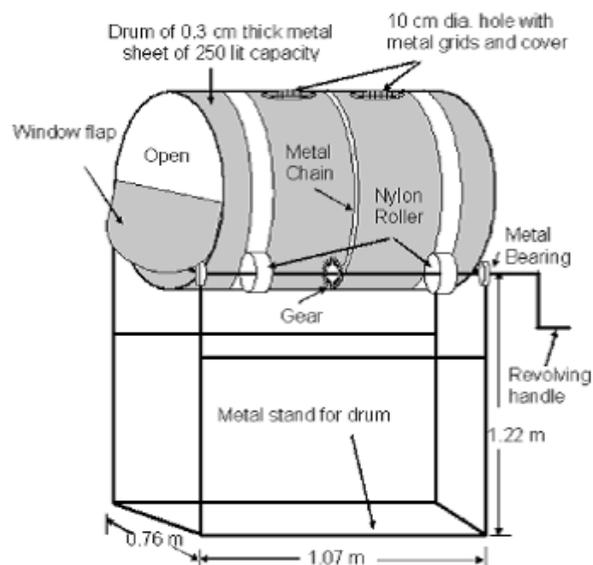
Figure 3.8. Single Household Rotary Drum Composter installed in IIT Roorkee (Source: Kalamdhad & Kazmi 2009)
