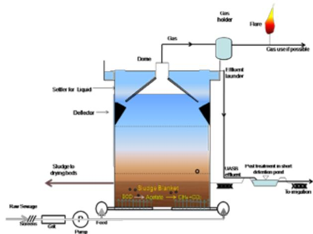
Figure 2.31. Schematic Diagram of UASB based plant (Source Kazmi A. A.2003)
