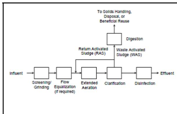
Figure 2.36 A typical flow sheet of Extended Aeration system (Source: USEPA 2000)
