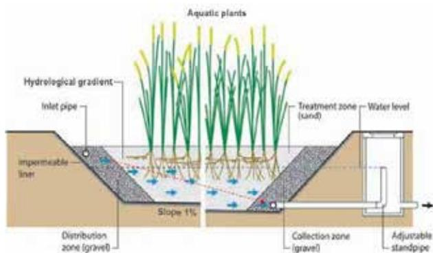
Figure 2.25. Horizontal flow constructed wet land:
