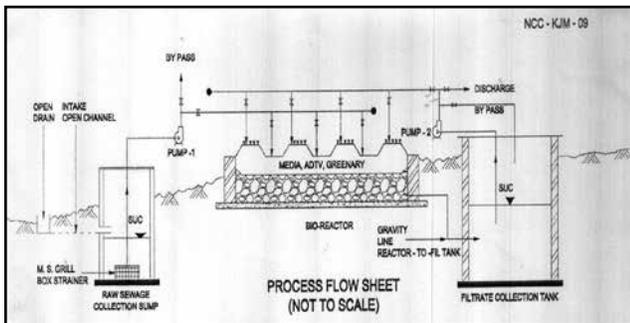
Fig 2.27 Design of a typical SBT
