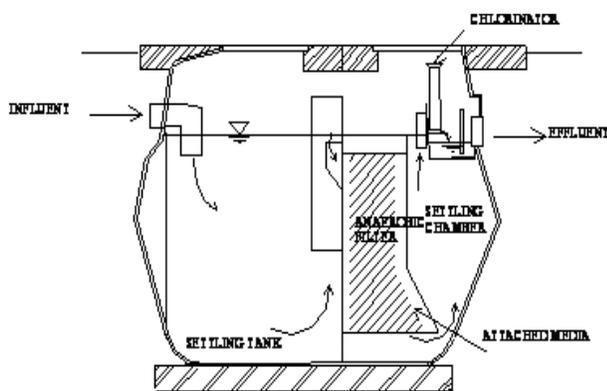
**Figure 2.8. Typical cross-sectional drawings of prefabricated septic-tank anaerobic filter type systems**
