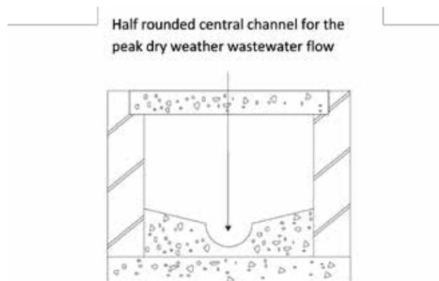
Figure 2.1. A Typical Channel section for carrying both dry weather wastewater flow and storm water.
