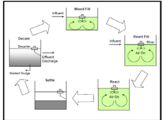
Figure 2.37. A Typical Cycle of Sequencing Batch Reactor (USEPA 2000)
