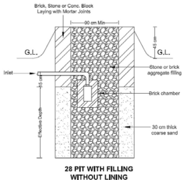
Figure 2.13 Typical illustrations of Soakage pit (IS 2470 : Part 2 : 1985)
