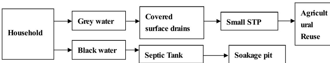
**Option-5: (Sanitation system using covered surface drains)**
