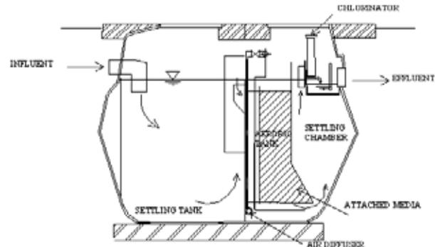
Figure 2.11: Typical cross-sectional drawings of package contact aeration system ( Kazmi 2003)
