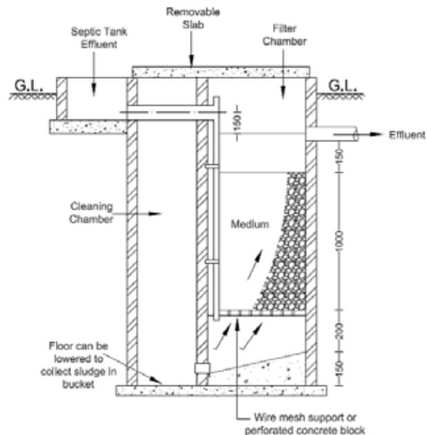
**Figure 2.9. Typical cross-sectional drawings of conventional septic-tank anaerobic filter type systems**
