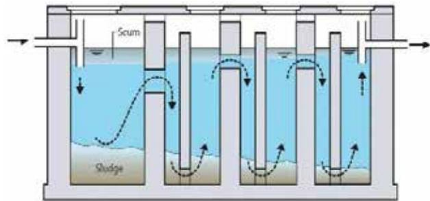
Fig. 2.28. Anaerobic Baffled Reactor;
