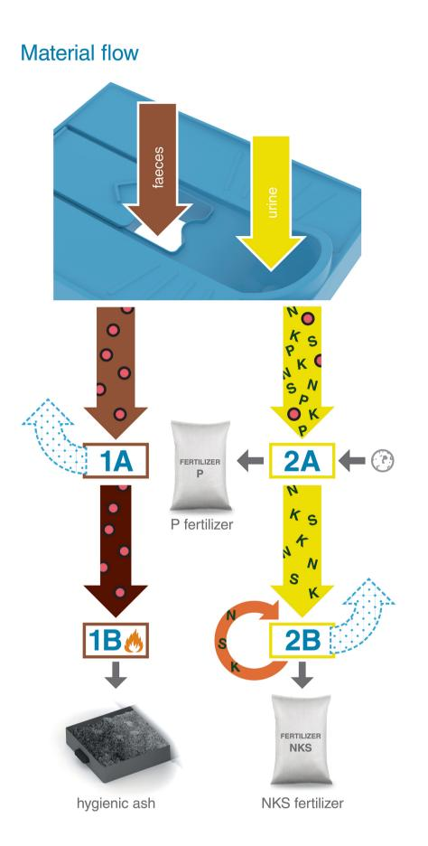
**2A** Stabilization of fresh urine Hydrated lime deposit preserves urea and inactivates viruses and bacteria
