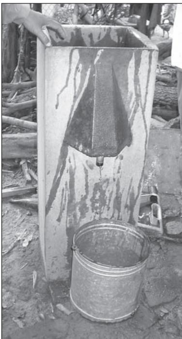
Figure 9.59. Sand water filter.
