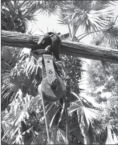
Figure 9.52. Locally made wood and metal pulley.
