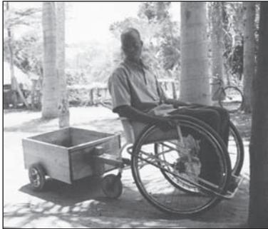
Figure 9.150. Two-wheeled wooden trailer.
