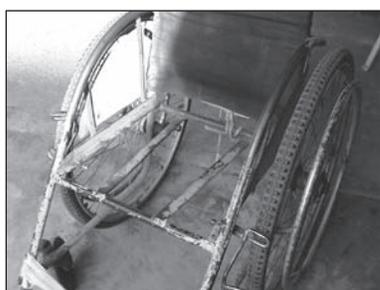
Figure 9.19. Wheelchair with cushion and seat board removed.
