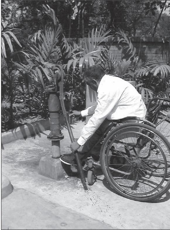
Figure 6.5. The same handpump operated by a wheelchair user on a level apron.
