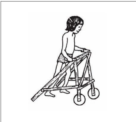
Figure 7.56. Example of a walking frame.
