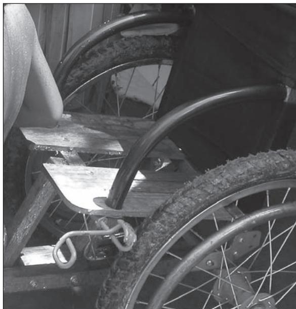
Figure 7.40. Wheelchair with a centre plank removed to leave a gap in the seat for toileting.\*
