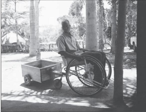
Figure 6.29. Two-wheeled wooden wheelchair trailer.
