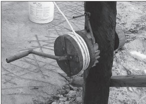
Figure 6.9. Detail of ratchet and pawl winding mechanism.
