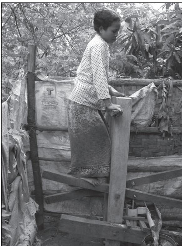
Figure 6.10. Treadle pump in operation.
