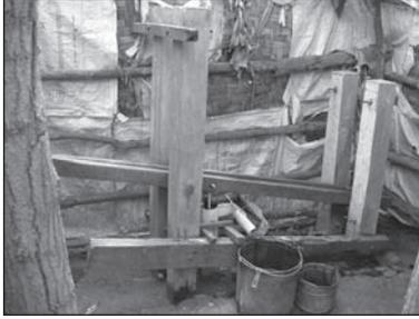
Figure 9.55. Treadle pump.
