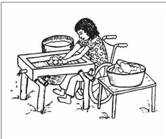
Figure 6.84. Concrete or wooden washstand with ridged bottom for washing clothes.
