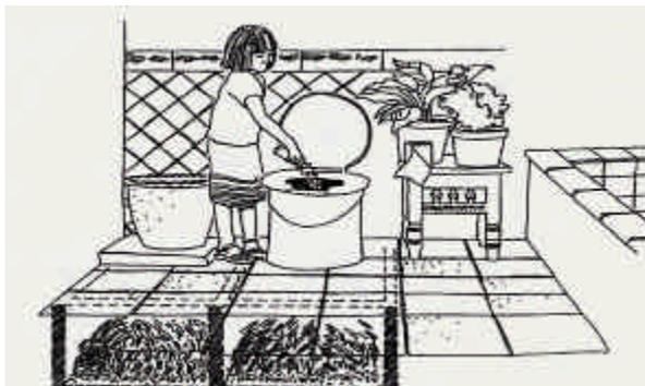
**Figure 2:** Dry, double-vault urine diversion toilet from Mexico.
