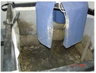
**Fig. 11:** Compost filter bags at trial stage, here with straw as structure material (source: LINZ AG, November 2007).
