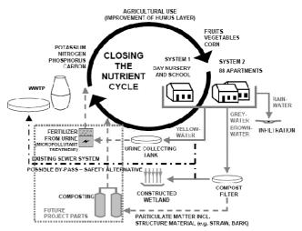
**Fig. 4:** Technological concept applied in the solarCity project (source: LINZ AG).
