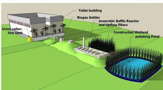
► figure 1: In Badlapur (agglomeration of Mumbai, India) an innovative sanitation concept has been implemented at a college for 1600 students. One measure is that the effluent from pour-flush squatting toilets is used for biogas production by passing it through an Upflow Anaerobic Sludge Blanket reactor. The treated blackwater is then purified in a constructed wetland and used for irrigation. (Source: ESF)
