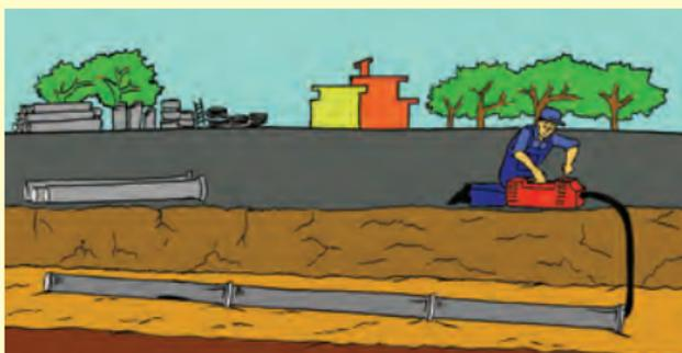
**Smoke Test:** Create thick smoke inside the pipe. Maintain a pressure of 25 mm of water for 15 minutes after all trap seals have been filled with water. Any evidence of smoke coming out of joints indicates leakage.
