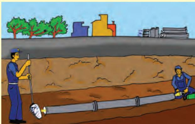
**Mirror Test:** Hold a mirror at one end of the line and lamp at the other. Full circle reflection of light indicates that the pipe is straight and free from any obstruction.
