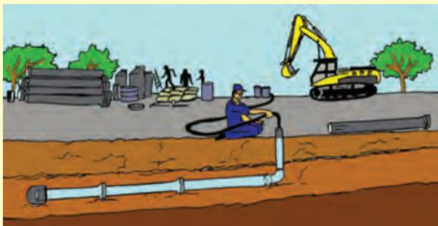
**Water Test:** Create Pressure of 1.5 m head of water at highest point of section being tested by closing the lower end. After 24 hours any drop in water level in the vertical end indicates leakage. This test is not used for cast iron pipes.
