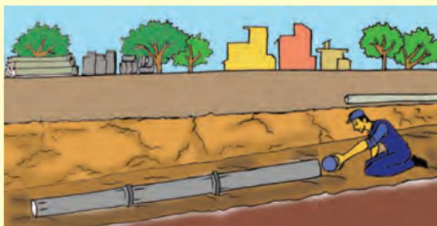
**Ball Test:** Insert a smooth ball of diameter 13 mm less than the pipe bore at the upper end. Smooth emergence of the ball at the lower end indicates absence of any obstruction.
