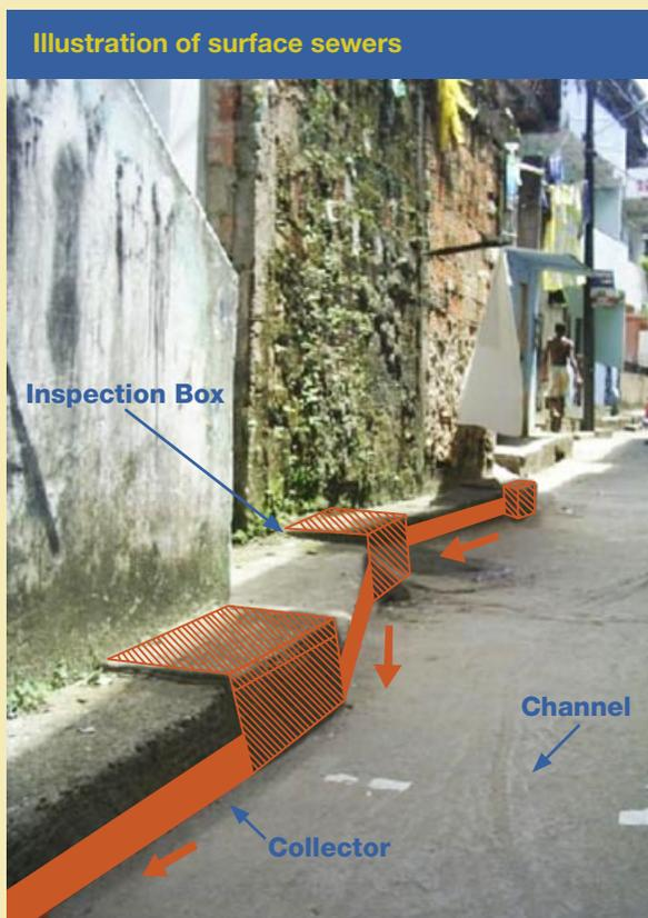
**Aerial sewers.** An extreme case of the aforementioned approach had to be used in cases where urban density was even higher and water runoff was not adequately covered or channeled. In these cases, flooding is usually prevented by placing the lower floors of the houses above the runoff level. This normally enables the installation of network branches bordering the houses, above the water runoff channels, either by using pipes attached to the house walls or supported on pillars.
