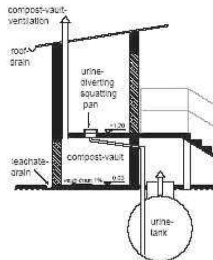
Figure 6: section of the toilet building (source TUHH)
