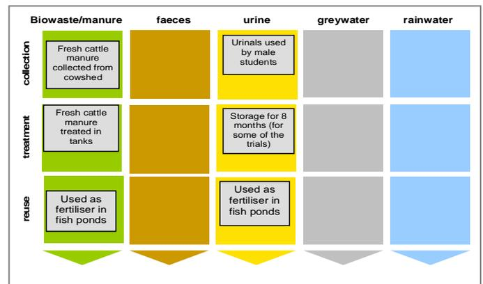
Fig. 2: Sanitation components used in the project
