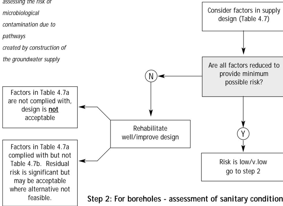
**Step 2: For boreholes - assessment of sanitary condition below surface**
