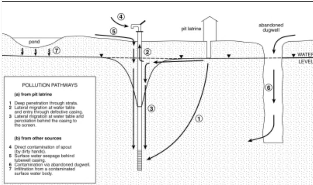
**Figure 3.10.** Pathways for contamination into groundwater supplies
