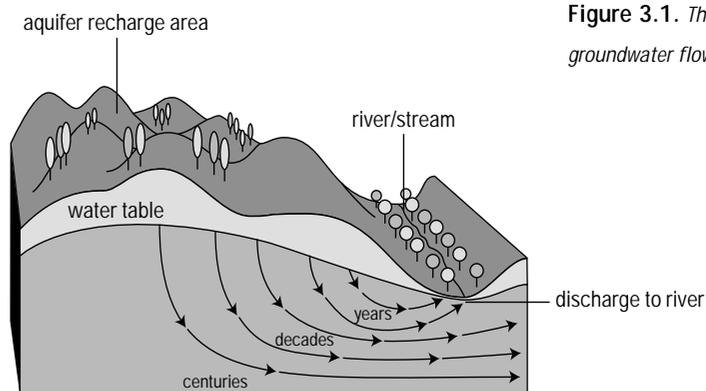
Figure 3.1. The groundwater flow system
