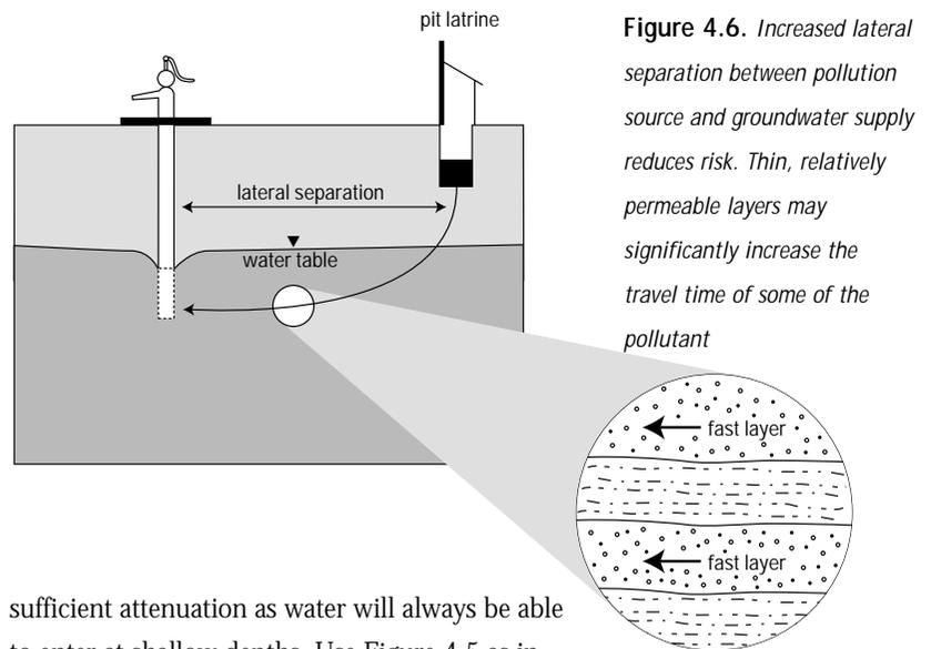
**Figure 4.6.** Increased lateral separation between pollution source and groundwater supply reduces risk. Thin, relatively permeable layers may significantly increase the travel time of some of the pollutant
