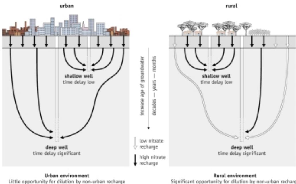
**Figure 4.11.** *Where boreholes are deep, the onset of high nitrate concentrations will be significantly delayed due to the time taken for the front of high nitrate waters to reach the borehole inlet. In smaller 'rural' settlements deep boreholes may tap lower nitrate waters derived from outside the settled area, which is less likely in an urban environment.*
