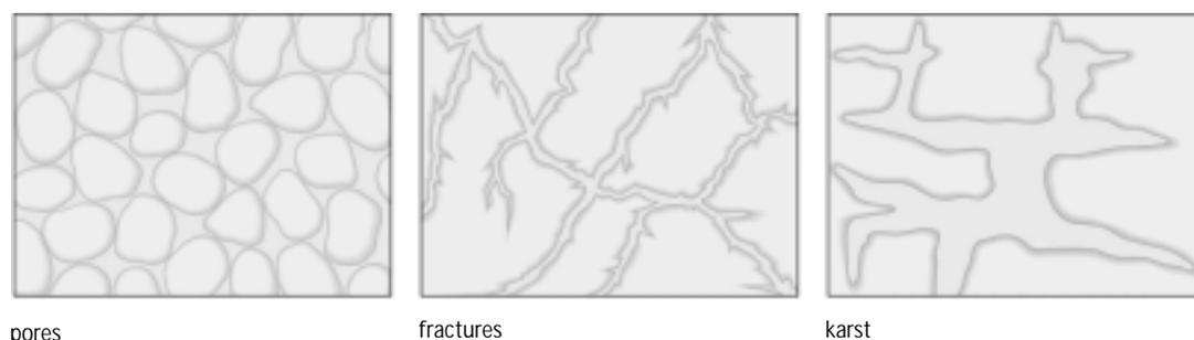
**Figure 3.2.** *Illustration of types of voids within rocks: pores - spaces between sediment grains; fractures - cracks in hard rock; karst - enlargement of fractures in calcareous rocks due to dissolution by infiltrating water that is slightly acidic*
