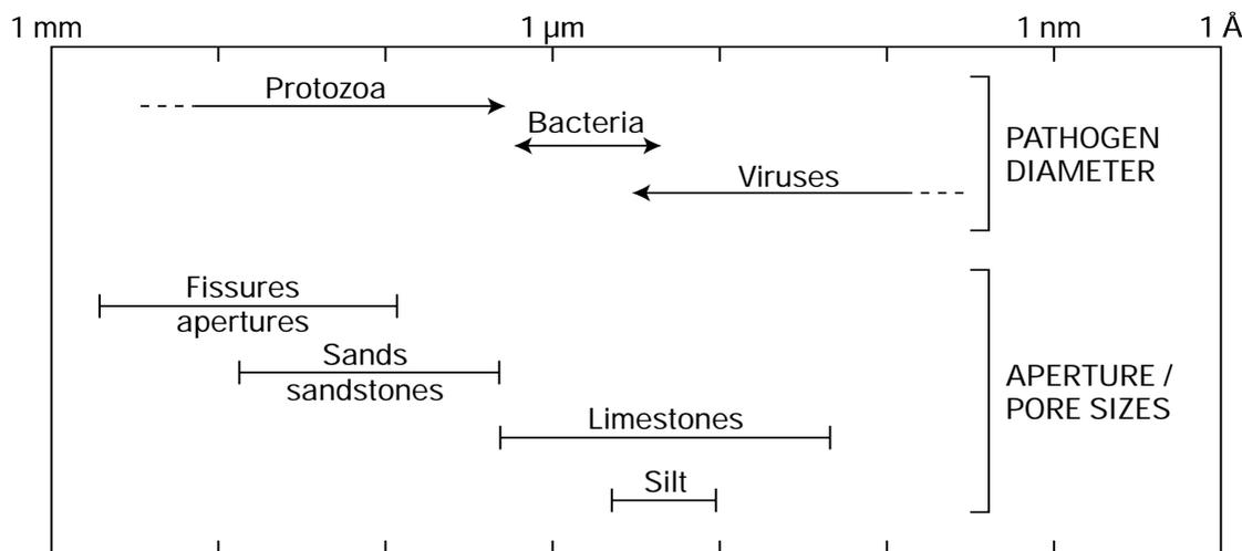
Figure 3.9. Pathogen diameters compared with aquifer matrix apertures
