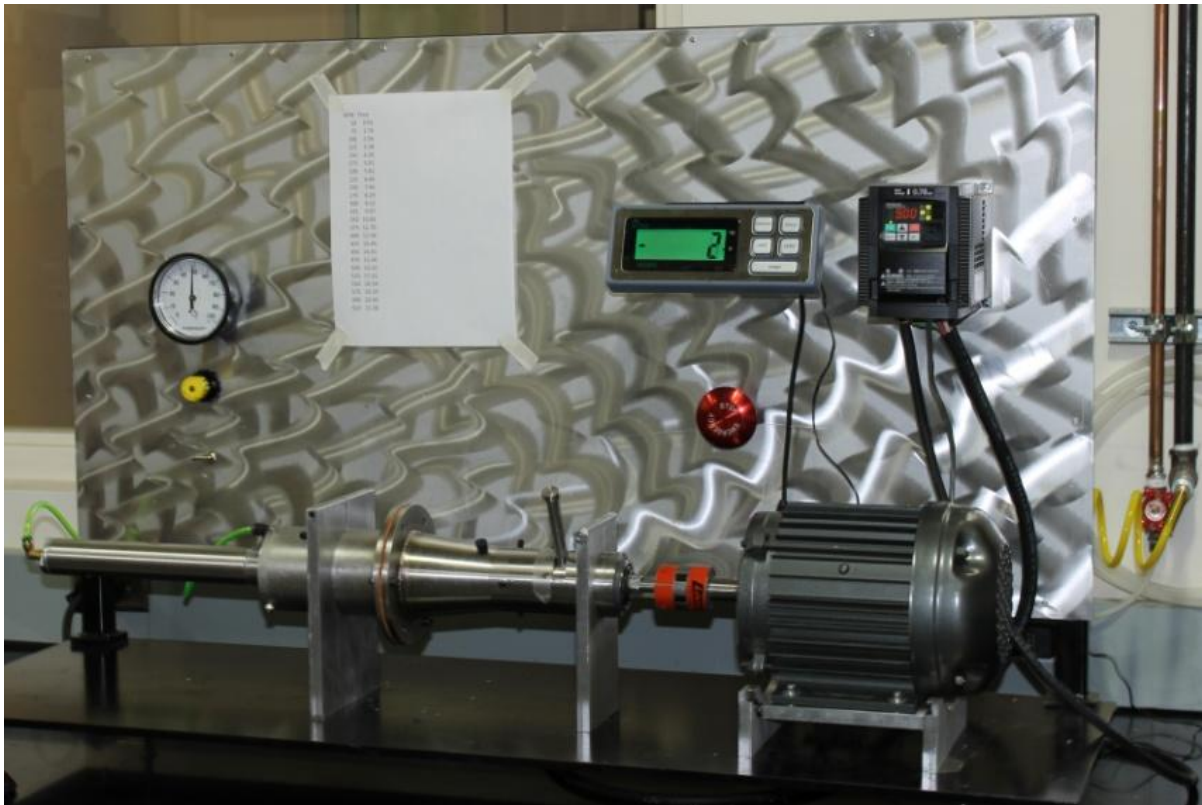
Figure 2. Instrumented reactor to process fecal and simulant solids
