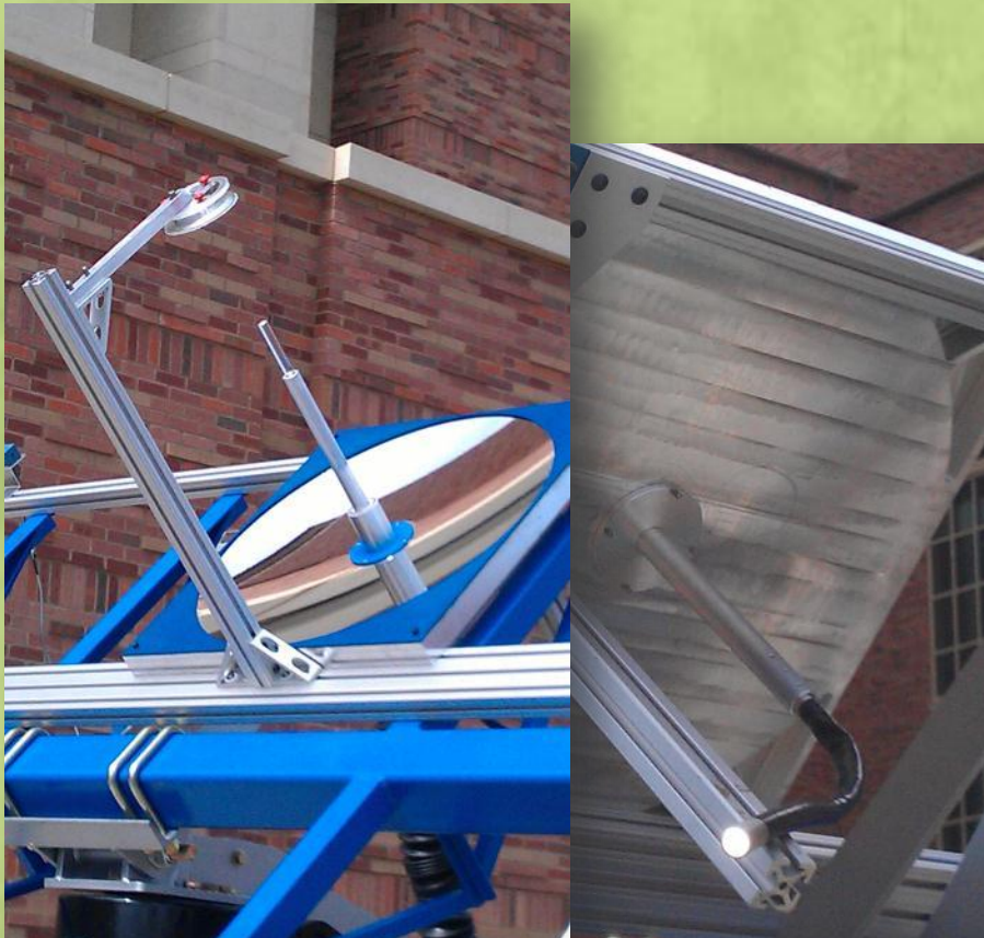
CSP transmitted through fiber optic bundle
