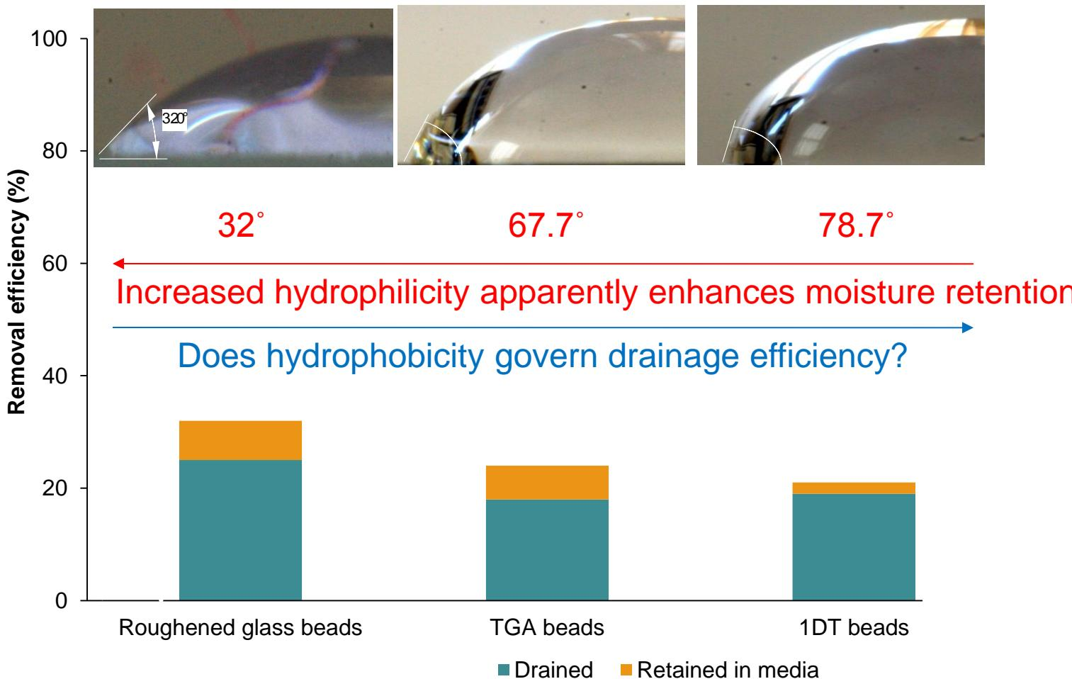
Synthetic urine vapour. Flow rate (4 LPM), BV (0.13 L),  $v$  (2.9 m/min), EBCT (1.95 s), temperature differential ( $< 2^\circ\text{C}$ )
