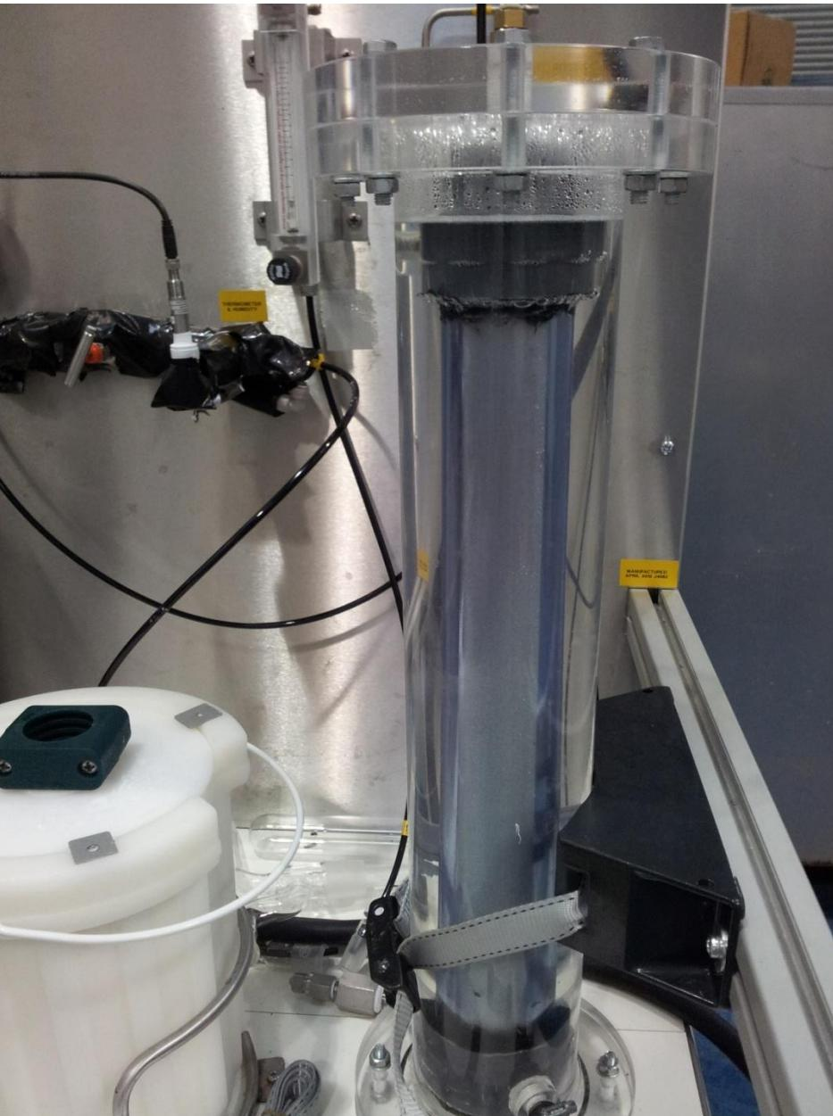
Initial data sets benchmarking standard glass media have shown ~ 40 % water capture from the vapour stream
