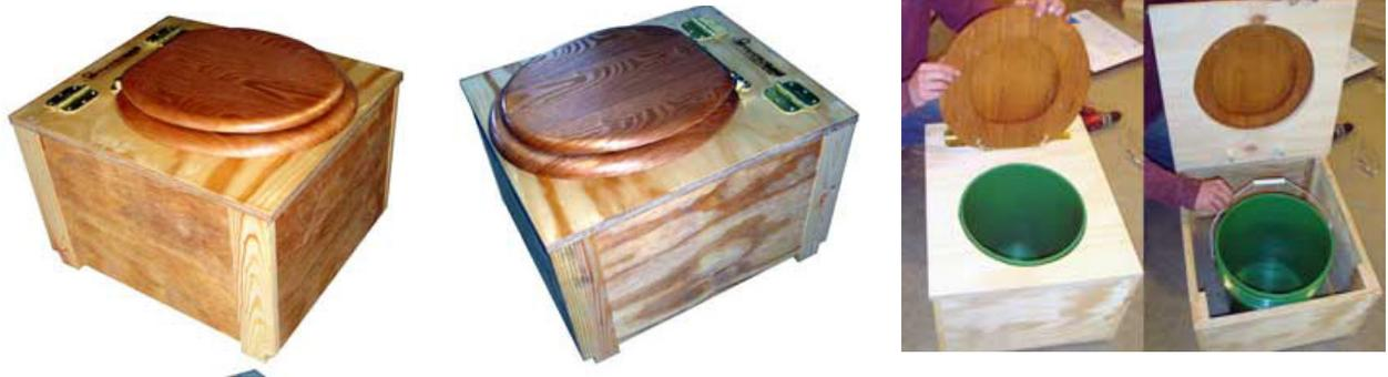
The finished loo is approximately 18" wide, 21" long and a little higher than the toilet receptacle, approximately 17". The toilet itself: 3/4" plywood base (polyurethane finish if selected), glued and screwed together, hinged 3/4" plywood top (with polyurethane finish if selected), with an oak style, wood core toilet seat. The toilet can be additionally painted or varnished, if desired, but can also be used as is.
