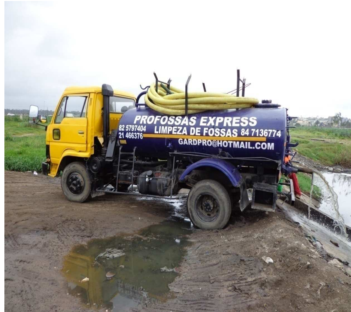
Truck discharges content of septic tanks from household's to stabilization ponds in Maputo.
