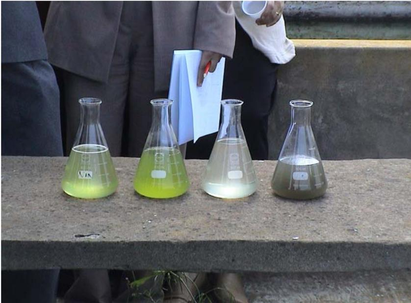
Raw wastewater (right), TSUAR second, HRAP third and final effluent (left)
