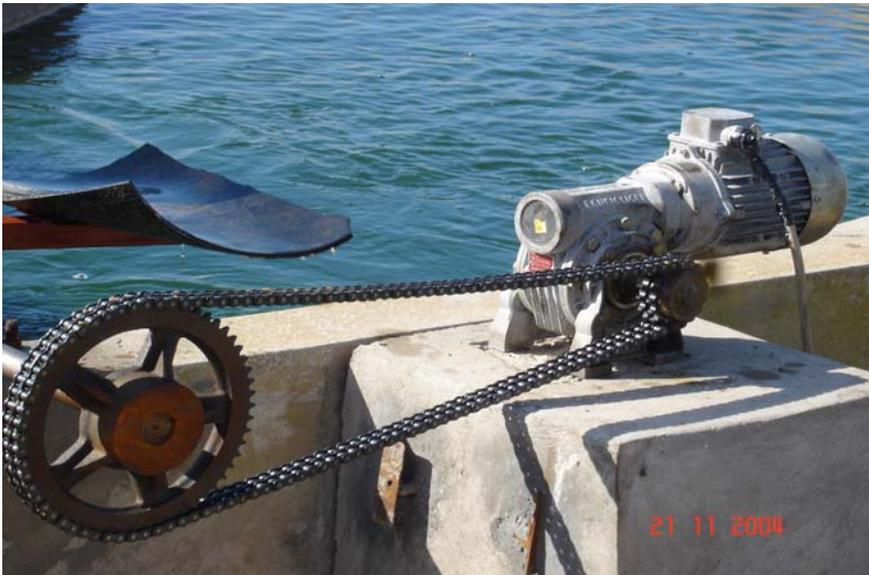
**Paddle wheel driving mechanism (electric motor and gear box control)**
