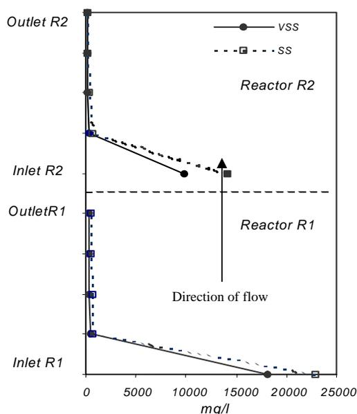
Figure 2. SS and VSS profiles in reactors R<sub>1</sub> and R<sub>2</sub>
