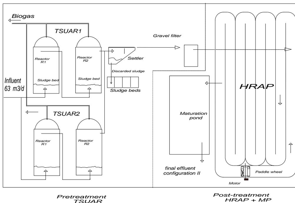
Figure 1. Layout of the treatment plant
