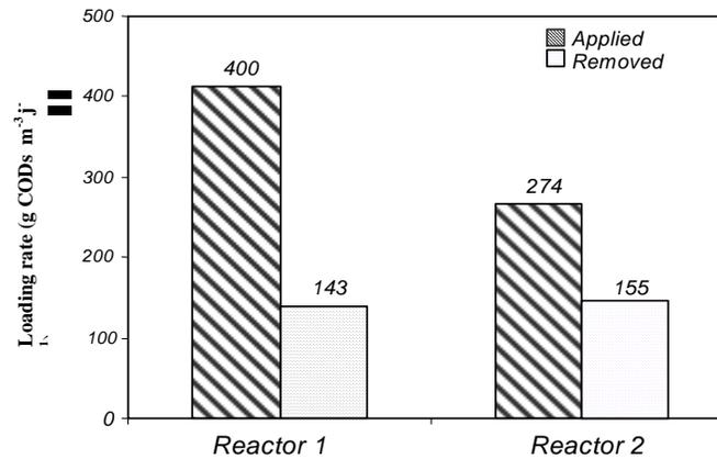
Figure 3. Applied and removed CODs for reactors  $R_1$  and  $R_2$
