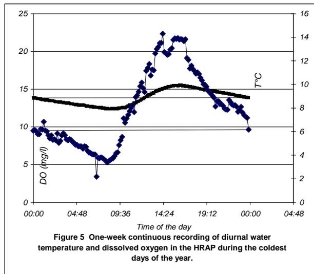
the same HRAP operated under configuration I (El Ouarghi *et al.*, 2000). The anoxic period recorded in the night, which extended for approximately 4 h was absent under configuration II.
