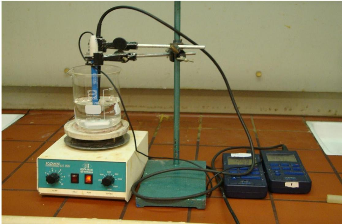
**Figure 3.6 Precipitation set-up**
