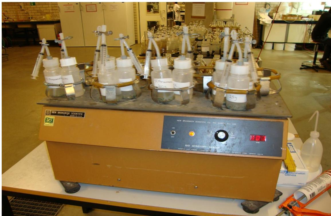
Figure 3.4 Batch adsorption set up
