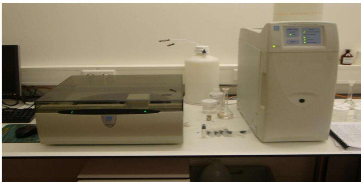
**Figure 3.7 IC Machine (Model: Dionex ICS-1000 ION Chromatography system).**
