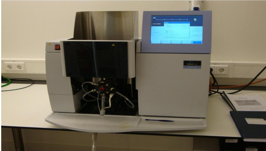
**Figure 3.5** Atomic emission spectrometer (Model: Perkin-Elmer AAnalyst 200)
