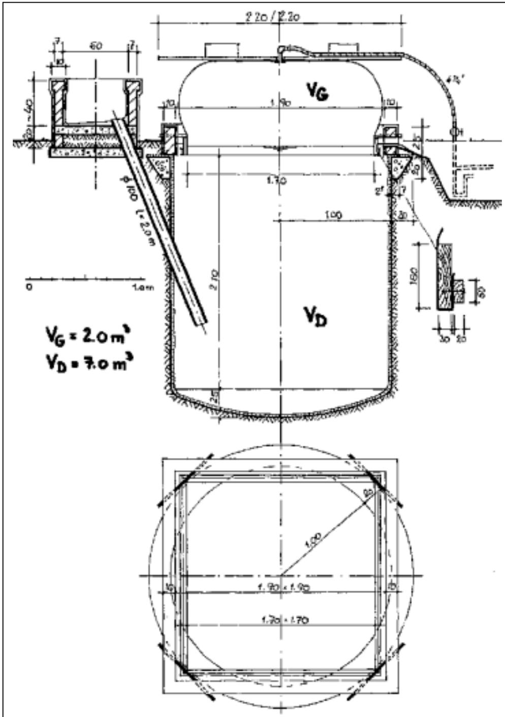
**Fig. 52:** Constructional drawing of a channel-type digester with folia (Henning system) The digester walls consists of netting-wire-reinforced rendering on the surrounding ground. The balloon serving as gasholder is mounted on a wooden frame. A plywood panel or straw mat on lathing serves as a sunshade. Weights placed on top make the gas pressure higher.
