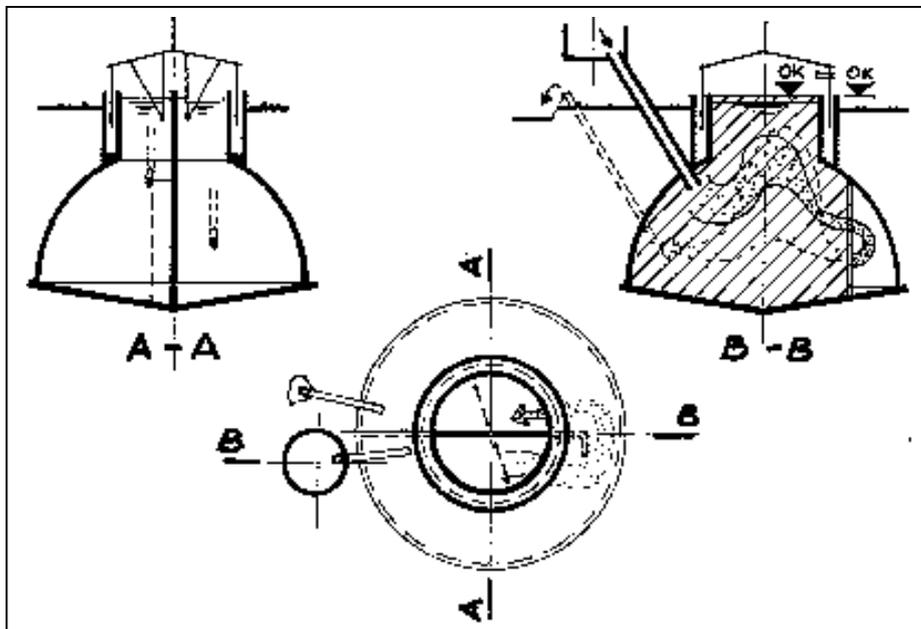
**Fig. 26:** Hemispherical plant with partition wall The principle of the fermentation channel is obtained by the fact that the inlet and outlet pipes are close together. The partition wall extends up above the surface level of the fermentation slurry. The gasholder must therefore float in a water jacket. The "horizontal KVIC gobar gas plant", which is similar in design, works perfectly with high gas production.
