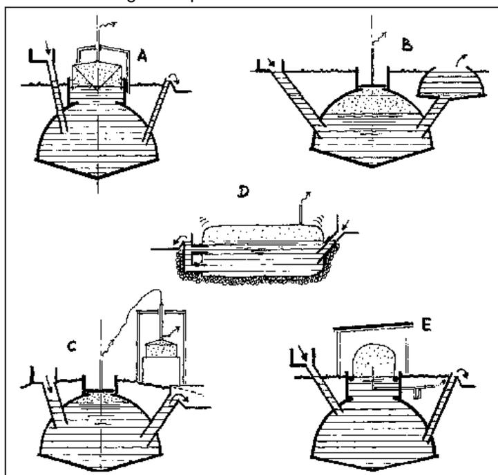
**Fig. 3:** Simple biogas plants A Floating-drum plant B Fixed-dome plant C Fixed-dome plant with separate gasholder. The gas pressure is kept constant by the floating gasholder. The unit can be operated as a continuous overflow-type plant with no compensating tank. The use of an agitator is recommended. D Balloon plant E Channel-type digester with folia and sunshade
