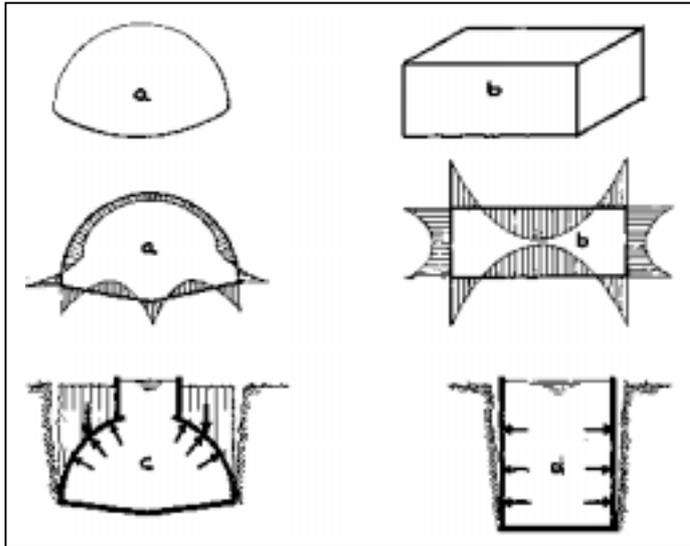
**Fig. 17:** Same volume - different shape. Different shapes have different stress patterns under the same load (a and b). The round shape has lower stresses. The angular shape has high stresses and many stress peaks. Different shapes are often loaded differently. In a vaulted shape, the loads acting in different directions are more reliably balanced than with a vertical wall (c and d).
