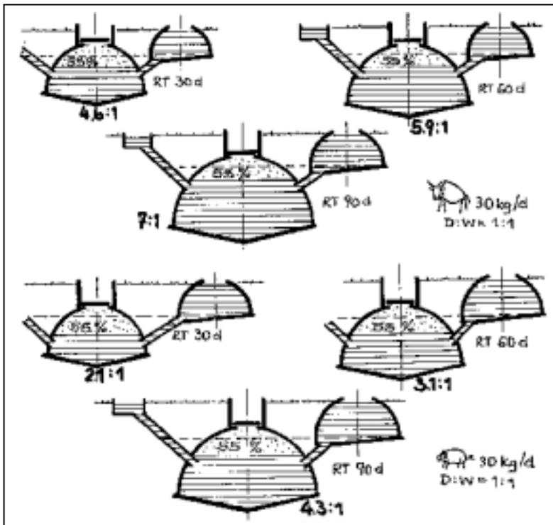
**Fig. 13:** Dependence of shape on retention time on a fixed-dome plant (cattle dung above; pig manure below) The filling volume and gasholder capacity ( $C = 55\%$ ) are the same in each case. The differences in digester/ compensating tank ratios result solely from the different retention time (Gd as a result of RT, Figures 7 and 8).
