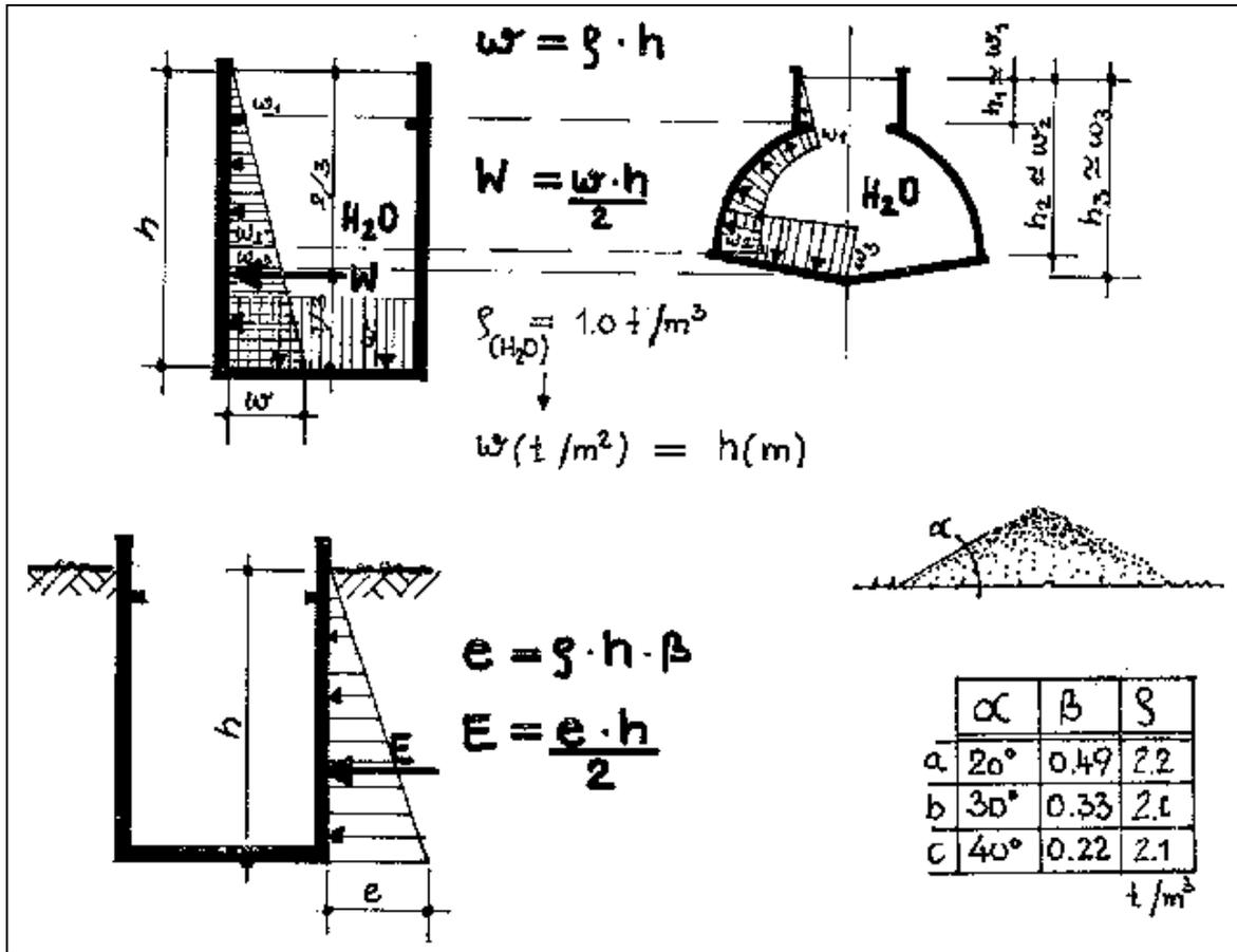
**Fig. 57:** Water pressure and earth pressure Water pressure depends directly on height. The amount of water has no effect on the pressure. The earth pressure depends on height, the angle of repose (alfa) and density (ro) of the earth. In the table, (a) is soft loam or clayey sand, (b) is pure sand and (c) is marl or murrum.
