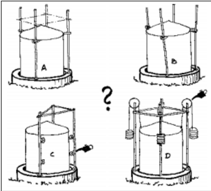
**Fig. 32:** Unsuitable guidance systems for floating drums. With these guides, the gas drum cannot be rotated. This means that floating scum cannot be broken up. The rollers and bearings must be lubricated. In arrangement (C), the paintwork of the drum is damaged. Plant (B) is jammed if only one of the guide rods is not vertical. A central guide tube is always better!
