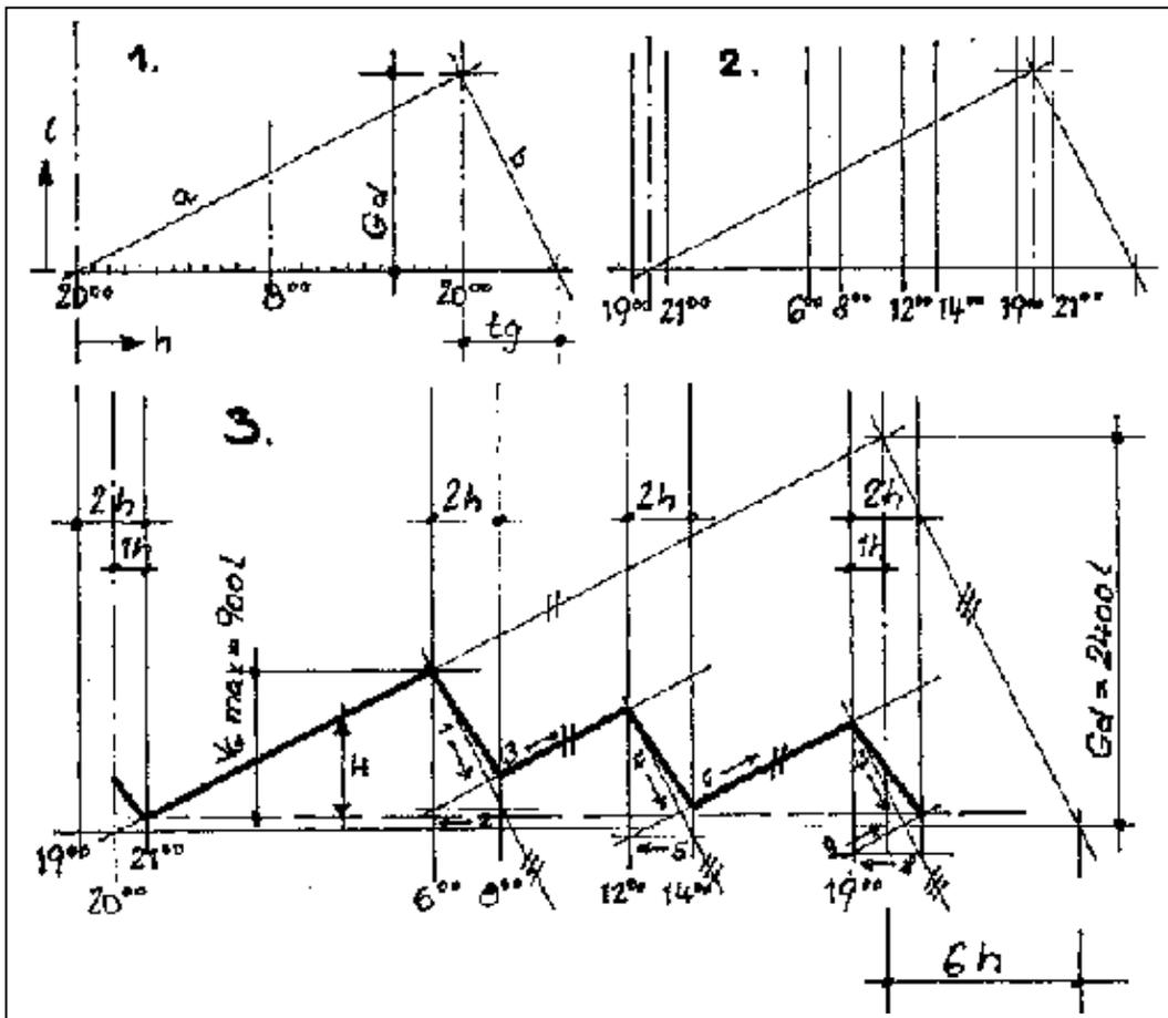
**Fig 9:** Graphic determination of required gasholder volume in accordance with the first example, page 21/22. Working steps: 1. Plotting of gas production curve (a) and gas consumption curve (b). 2. Plotting of gas consumption times. 3. The gasholder curve (thick line) is determined by parallel shifting in accordance with the numbered arrows (1-9). The value VG does not yet include the safety margin of 25 %
