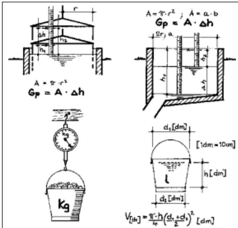
**Fig. 15:** Measuring gas production on the plant. In a floating-drum plant, the height of the gasholder is measured (top left). In a fixed-dome plant, the height of the slurry level is measured (top right). The manure is either weighed or measured in litres before introduction to the plant. Containers whose shape is easy to calculate are more accurate. If the lengths are measured in dm (1 dm = 10 cm), the volume in litres is obtained directly.
