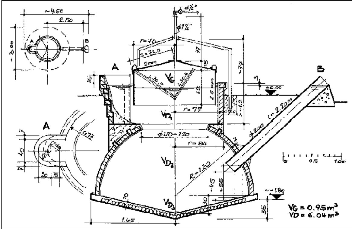
Fig. 43: Constructional drawing of a floating-drum plant with filler funnel for long-fibre feed material; external guide, external gas outlet.
