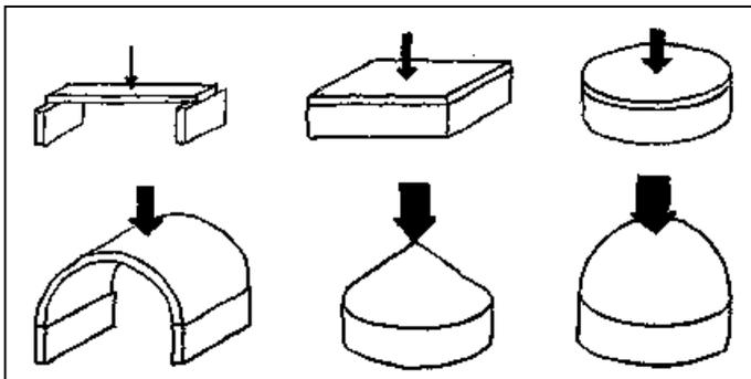
**Fig. 16:** Shape and load-bearing capacity.
