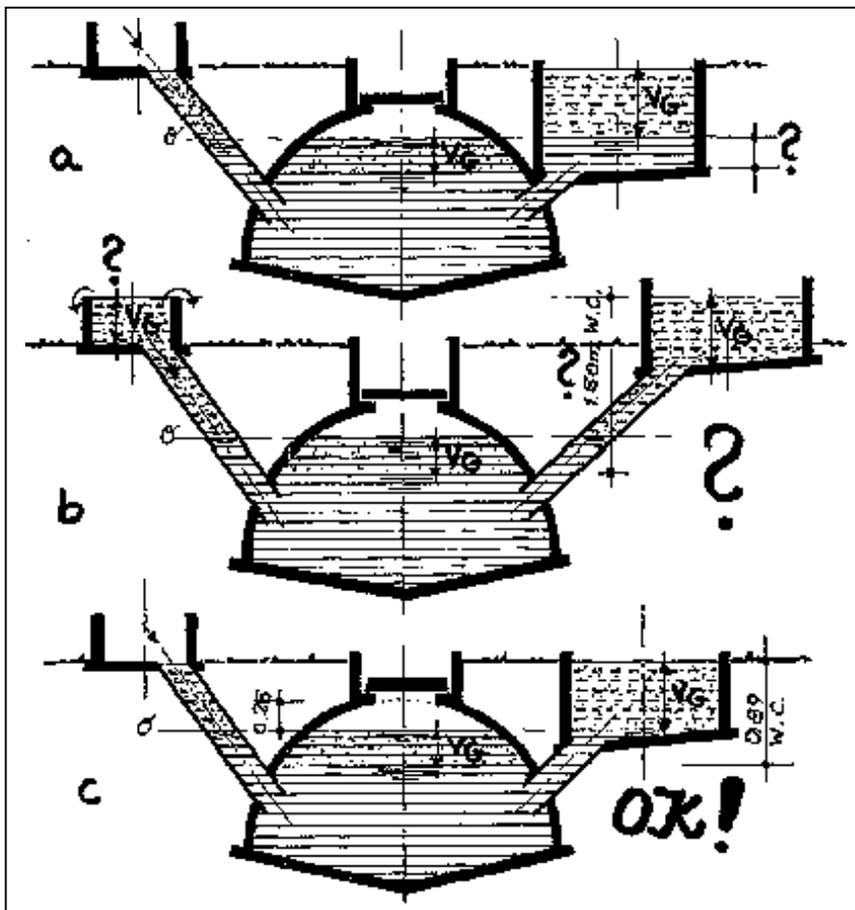
**Fig. 35:** Correct height of compensating tank The bottom of the compensating tank is at the level of the zero line (filling line). The zero line is 25 cm below the head of the digester dome (c). Wrong: (a) the bottom of the compensating tank is too low. Part of the slurry is always in contact with air. Gas is lost. Unnecessary cost. (b) The bottom of the compensating tank is too high. The gas pressure rises very fast and to a very high level.
