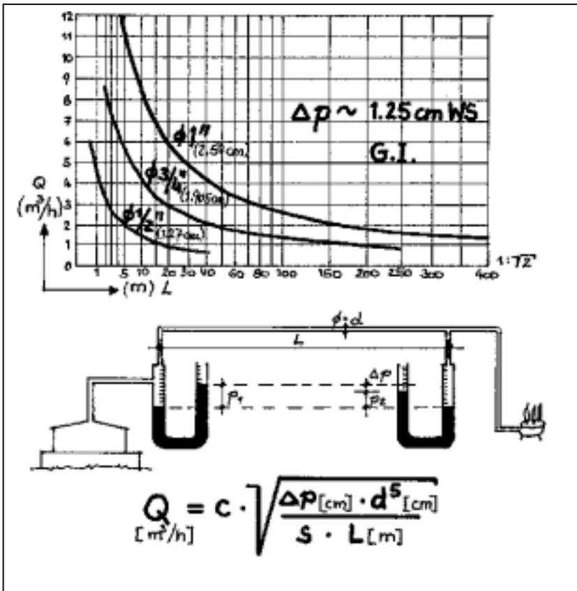
**Fig. 39:** Pressure drop in gas pipes. The gas pressure ( $p$ ) falls with pipe length ( $L$ ). The density relative to air is indicated by "s". The pressure drop depends on the pipe friction ( $c$ ) and especially on the diameter of pipe ( $c = 2.24$  in galvanized steel pipes (G.I.);  $c = 2.80$  in smooth plastic pipes). The curve shows the gas flow ( $Q$ ) in a galvanized steel pipe allowing for a pressure drop of  $p = 1.25$  cm WC. Bends increase the pressure drop.
