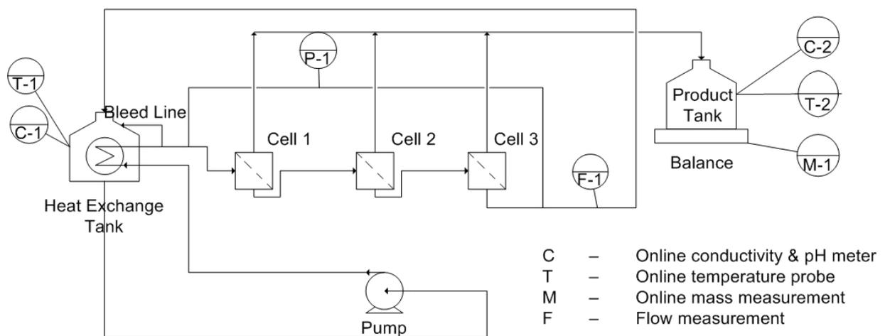
**FIGURE A7.5 NANOFILTRATION RIG PROCESS FLOW DIAGRAM**
