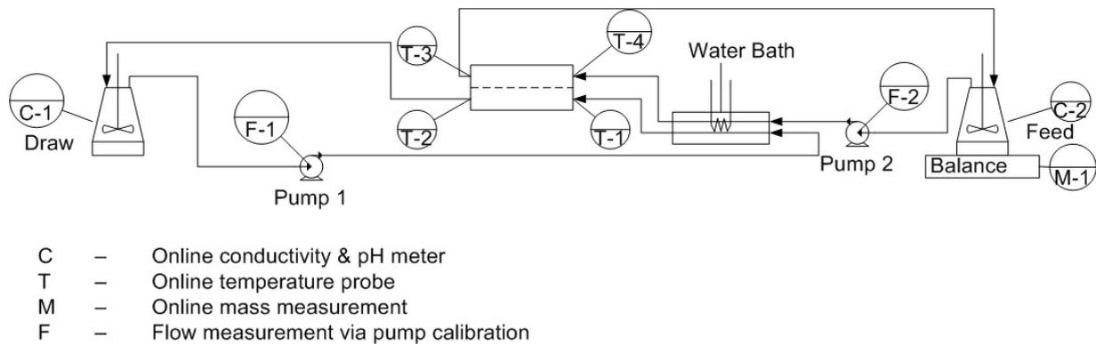
**FIGURE A7.8 FORWARD OSMOSIS RIG PROCESS FLOW DIAGRAM**
