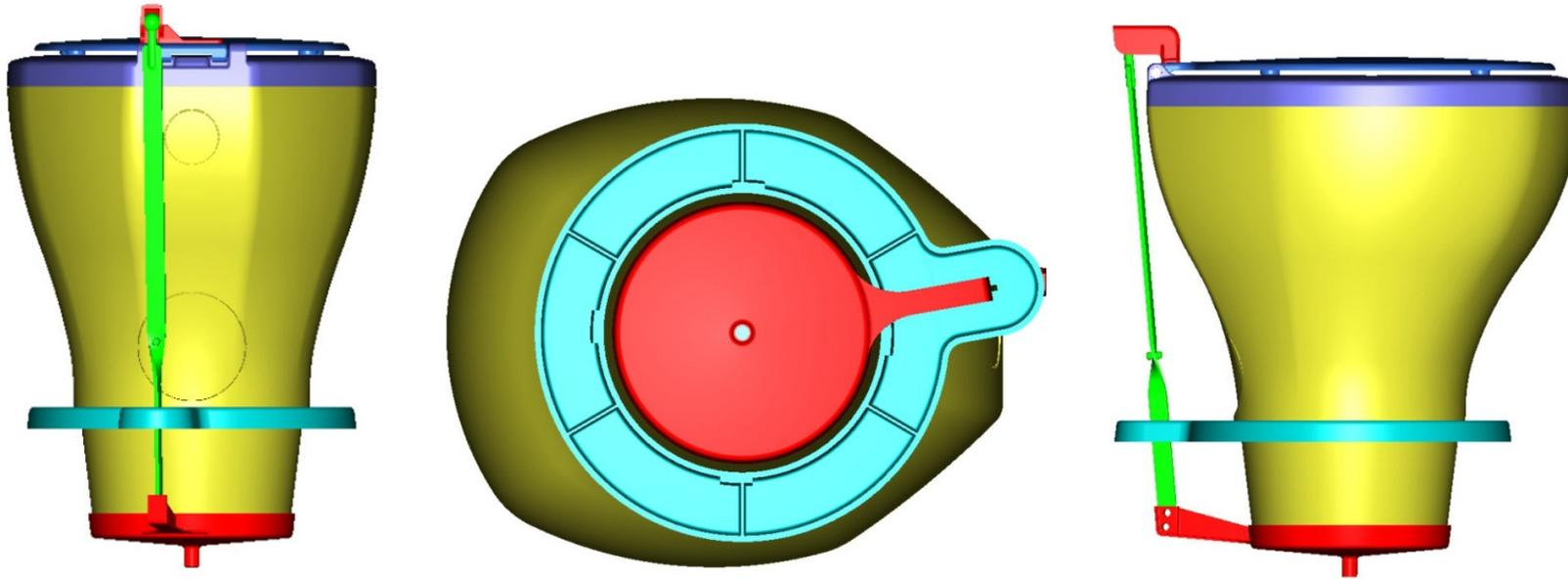
**FIGURE A5.2 DESIGN DRAWINGS FOR FIRST STAGE PEDESTAL PROTOTYPE. STRUT SECTION (GREEN) CONVERTS TOILET LID-LIFTING ACTION INTO A ROTATIONAL MOTION TO SWING THE WASHWATER DIVERSION BOWL (RED SECTION) AWAY FROM THE BOTTOM OF THE PEDESTAL, ALLOWING SOLIDS TO DROP THROUGH THE PEDESTAL TO THE PROCESSING SECTION BELOW.**
