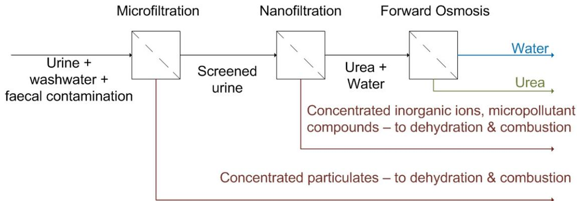
**FIGURE 6.2 HIGH-LEVEL PROCESS FLOW DIAGRAM FOR MEMBRANE PROCESSING OF URINE**
