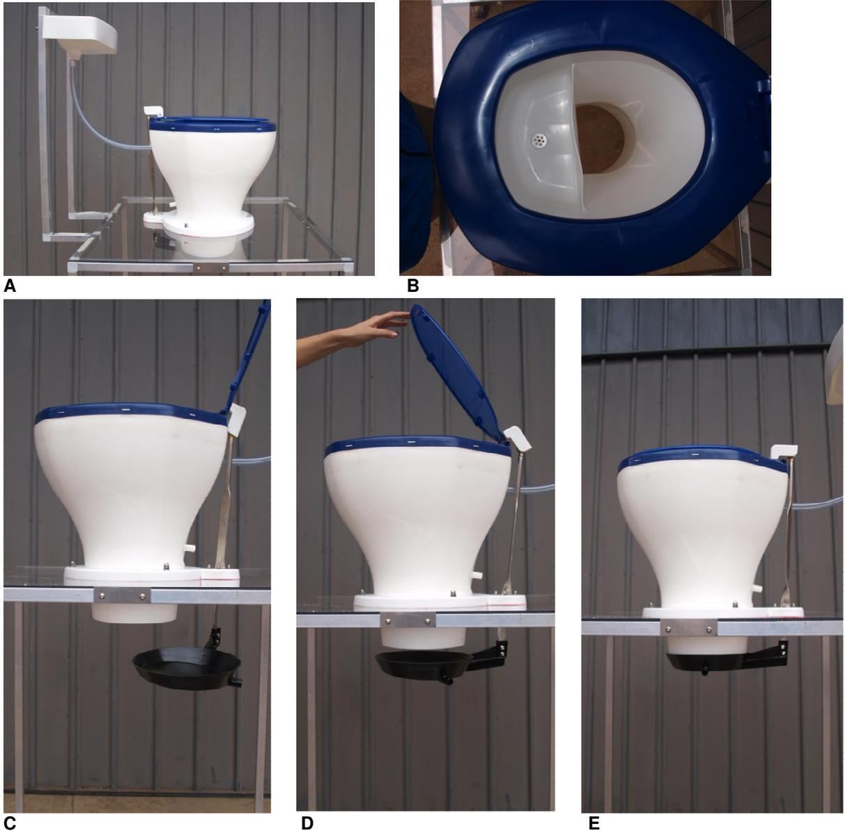
**FIGURE 4.1 TOILET PEDESTAL: THREE-STREAM SOURCE SEPARATION (A) DIVERSION OF USED HAND-WASHING WATER TO RINSE TOILET PEDESTAL (B) URINE SEPARATION SECTION (C) – (D) MECHANISM FOR CONTAMINATED WASHWATER DIVERSION**
