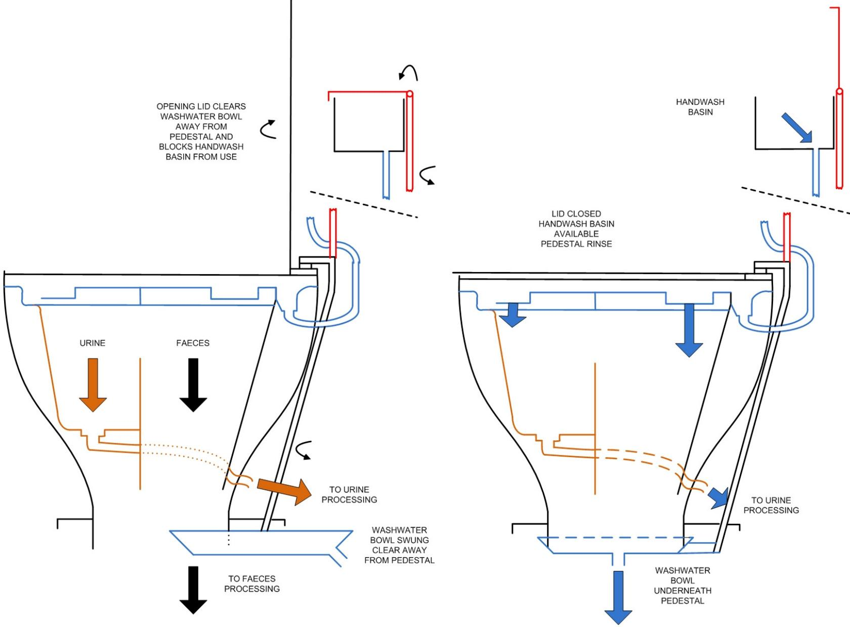
FIGURE A5.1 DESIGN CONCEPT FOR SOURCE-SEPARATION PEDESTAL
