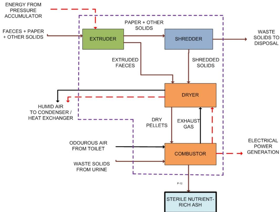
**FIGURE 5.2 PROCESS FLOW DIAGRAM OF SOLIDS-PROCESSING SECTION OF TOILET SYSTEM**
