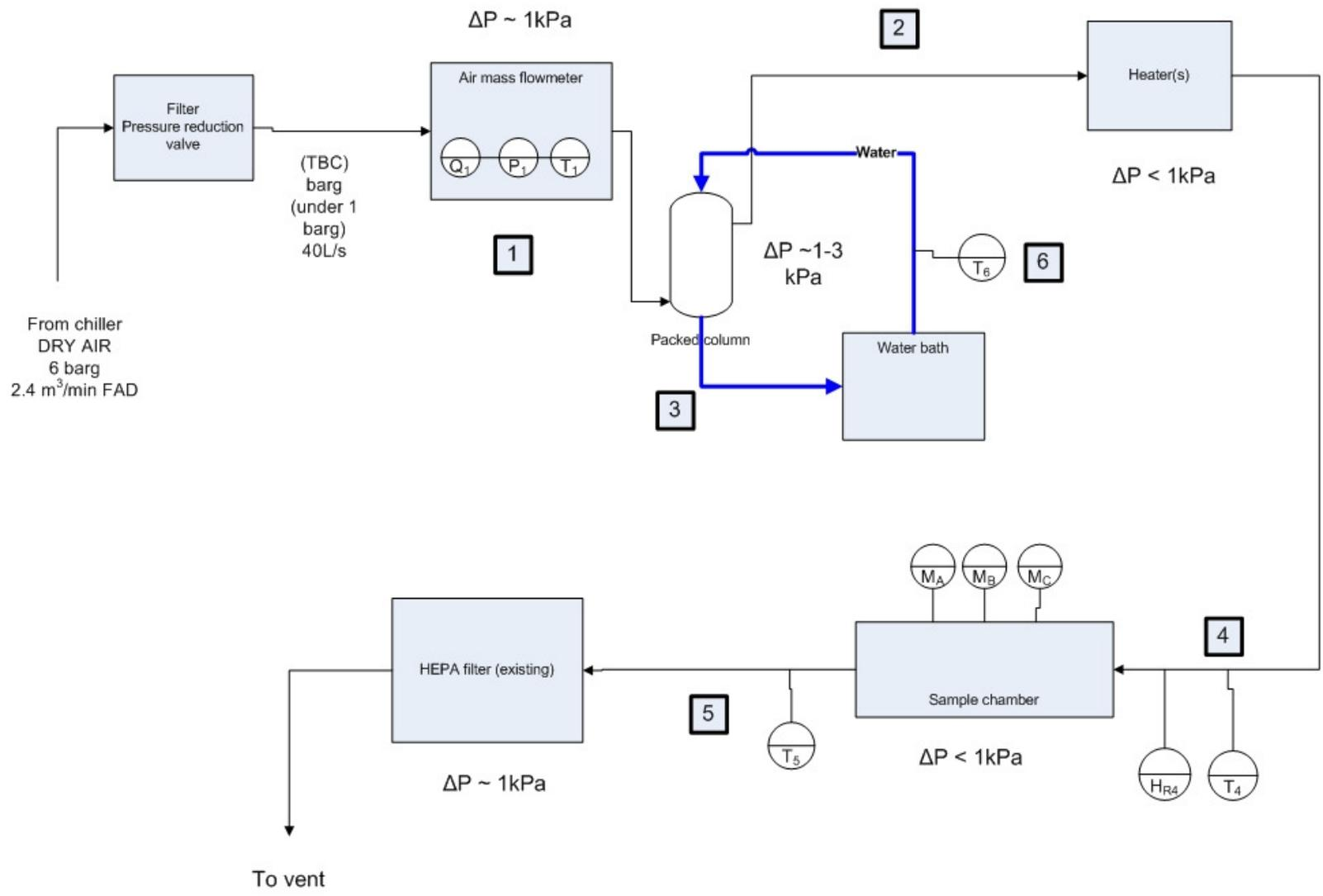
FIGURE A7.1 PROCESS FLOW DIAGRAM OF DRYING RIG
