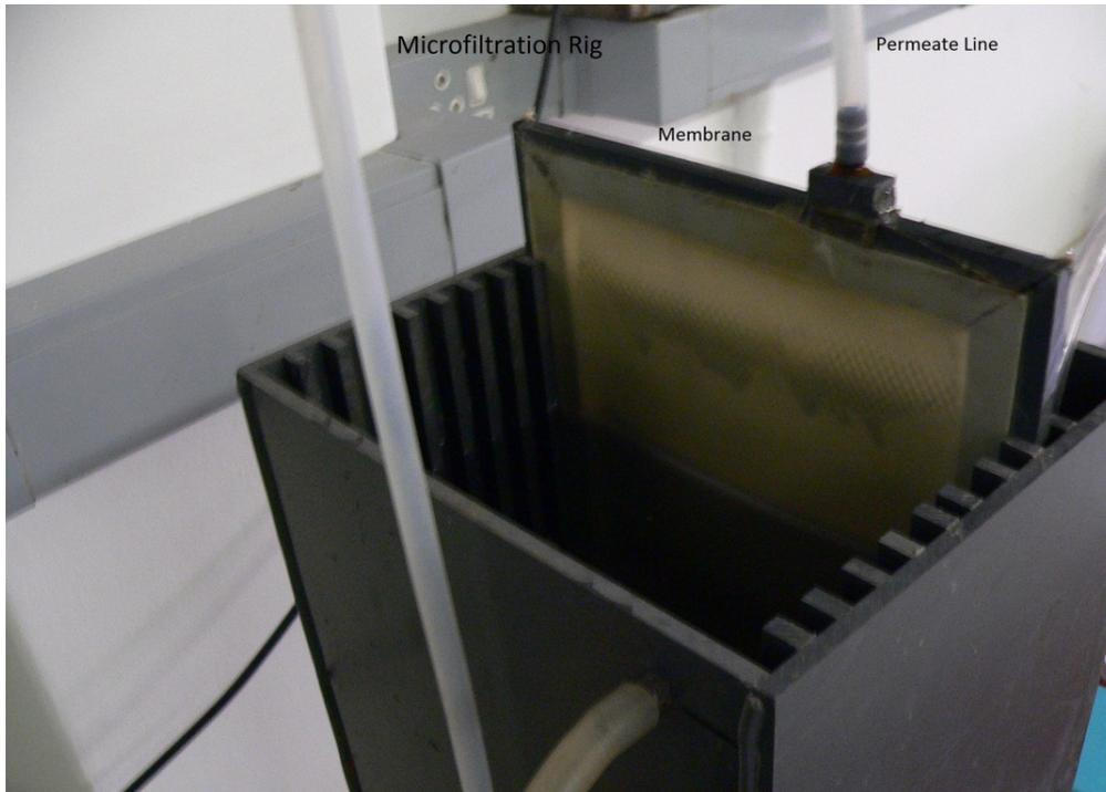
**FIGURE A7.4 MICROFILTRATION TEST RIG – MEMBRANE HOLDER**
