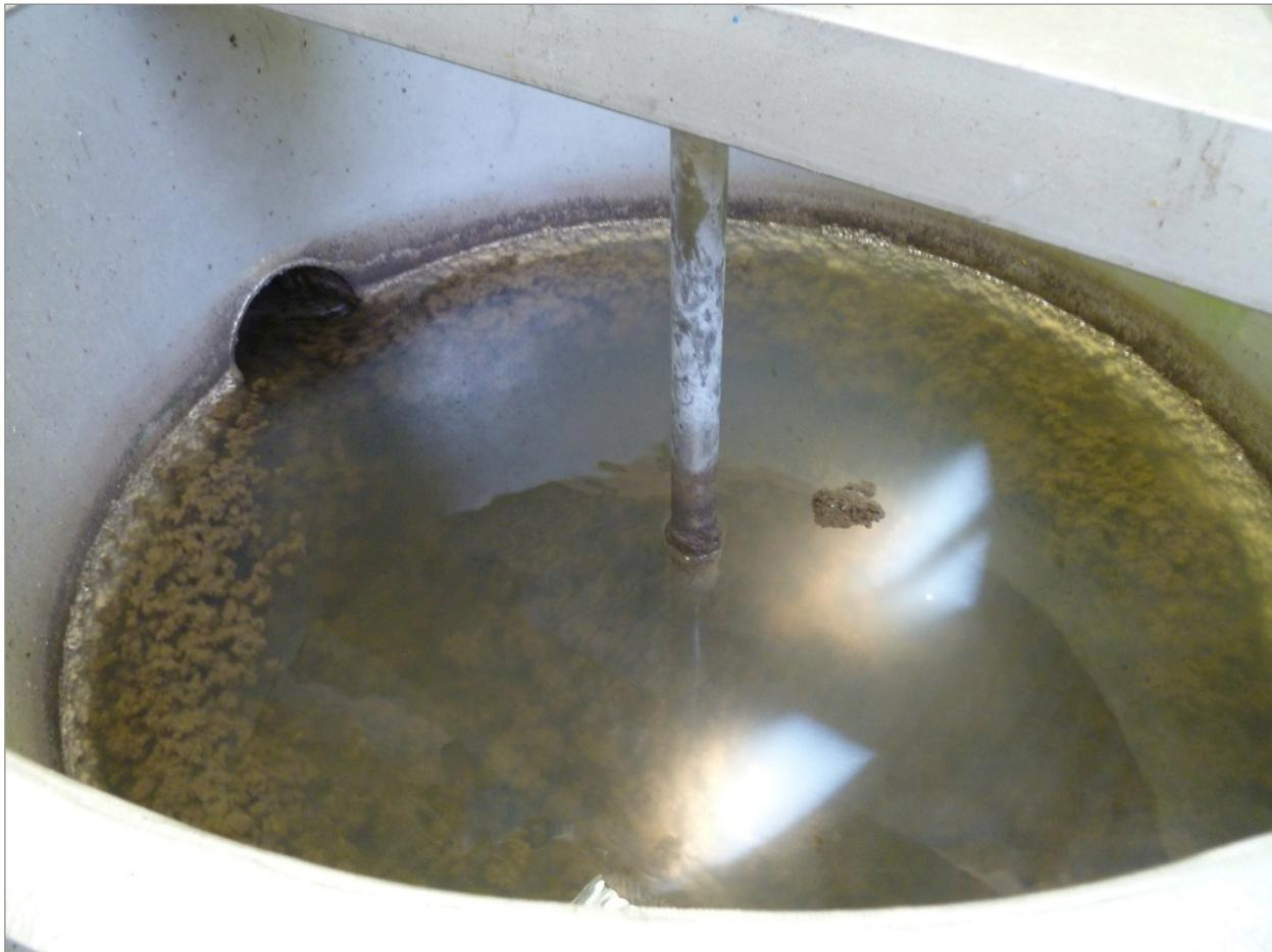
**FIGURE 2:** Flocculation Tank. Note the relative clarity of the separated liquid. Before the polymer mixing process, the liquid entering the system was a thick dark brown color.
