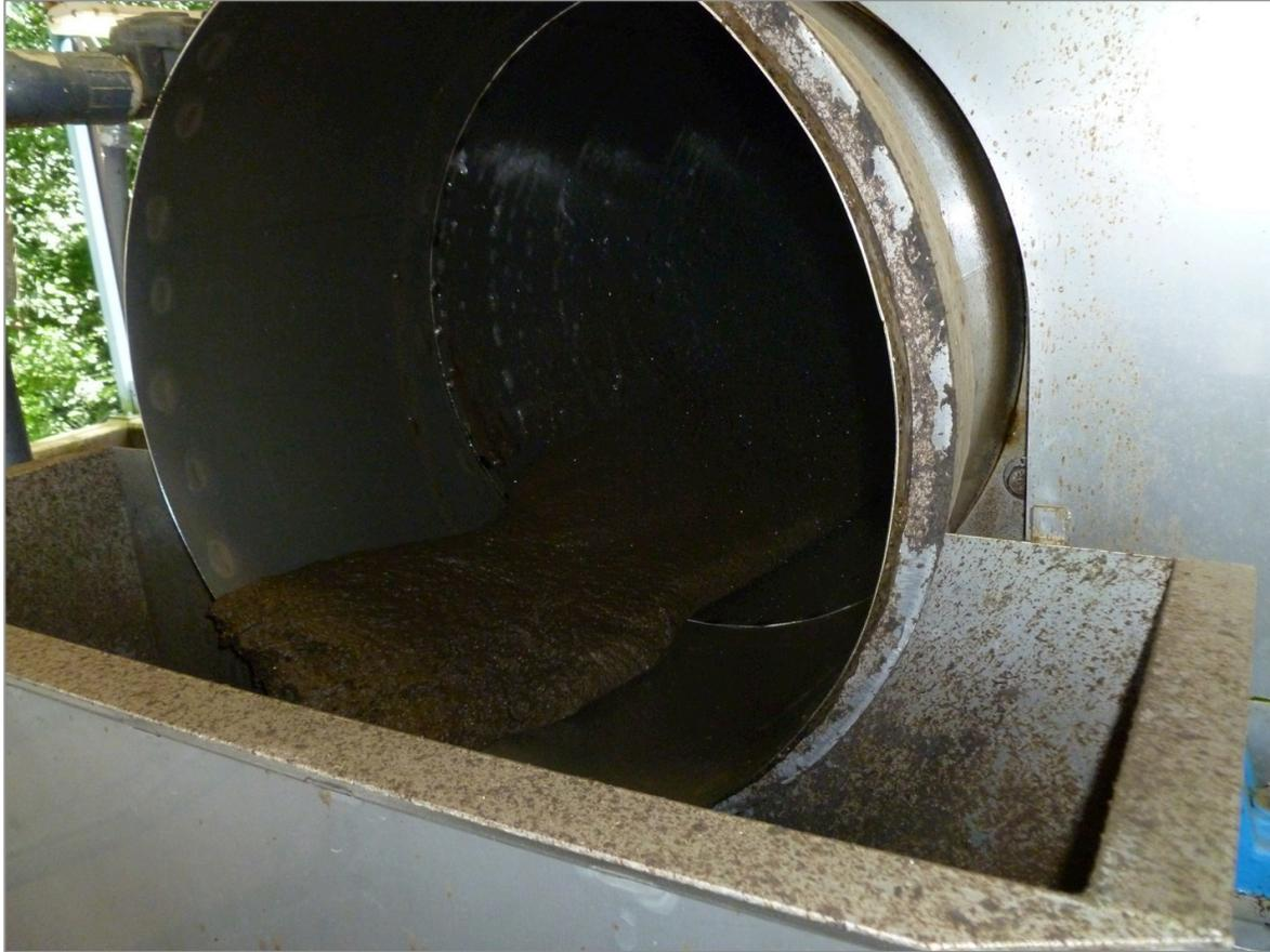
**FIGURE 3:** Discharged thickened sludge
